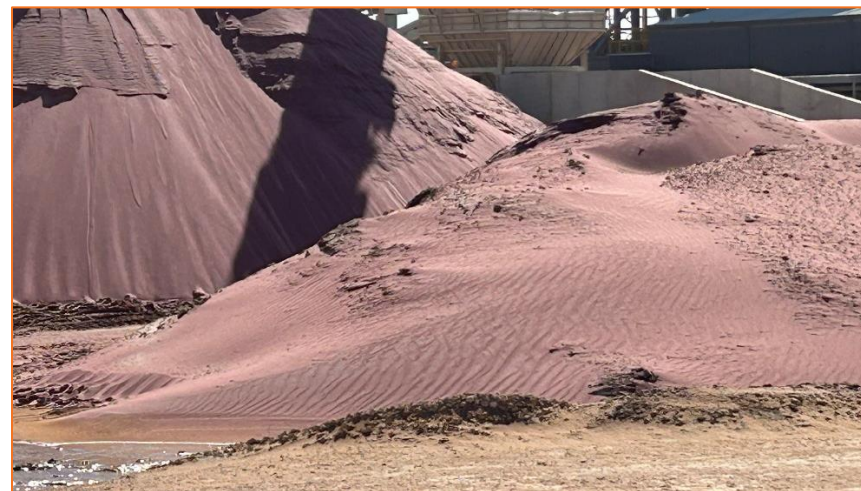
Figure 3-11: Product exposed to wind, note rilling indicative of wind erosion (ETA, 2023)
