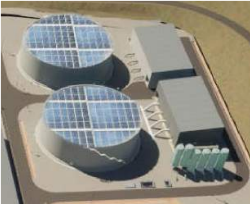
Plate 32 - 3D Model of Drinking Water Tanks, Drinking Water Pump Station and Surge Vessels (Northern Water Partnership, 2023)
