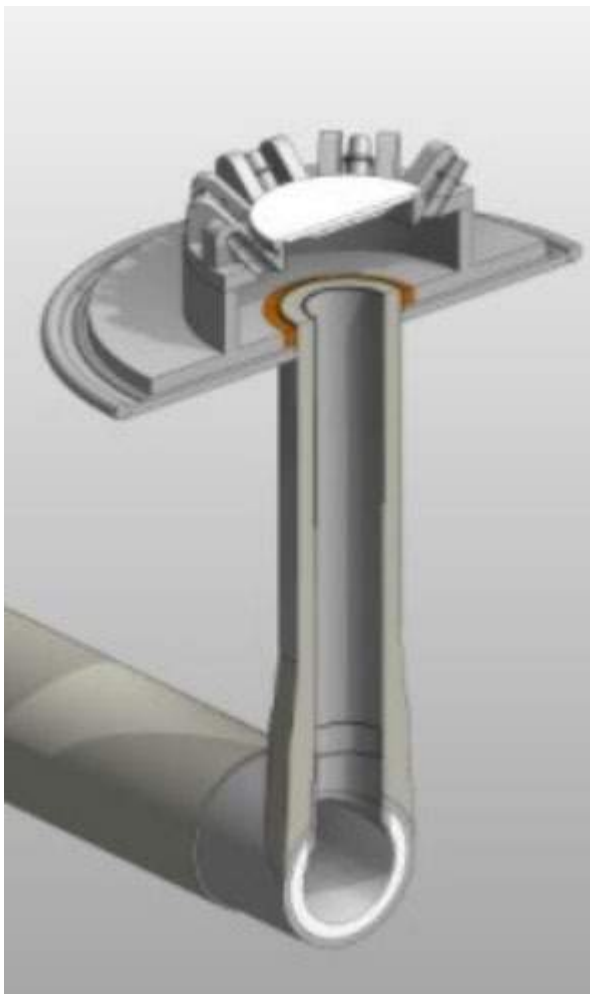
Plate 11 - 3D Model Section View through a Brine Diffuser Structure and Riser (Northern Water Partnership, 2023)
