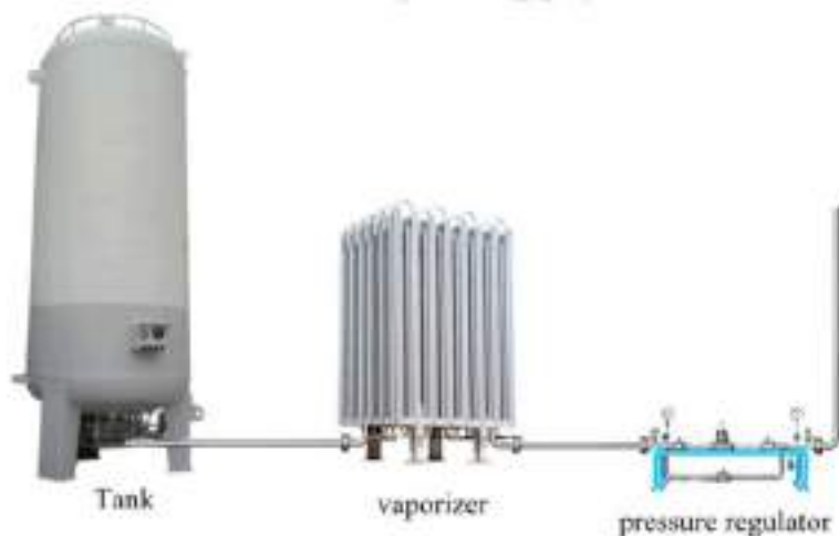
Plate 24 - Cryogenic liquid carbon dioxide tank, atmospheric vaporizer and pressure regulator illustration (Northern Water Partnership, 2023)
