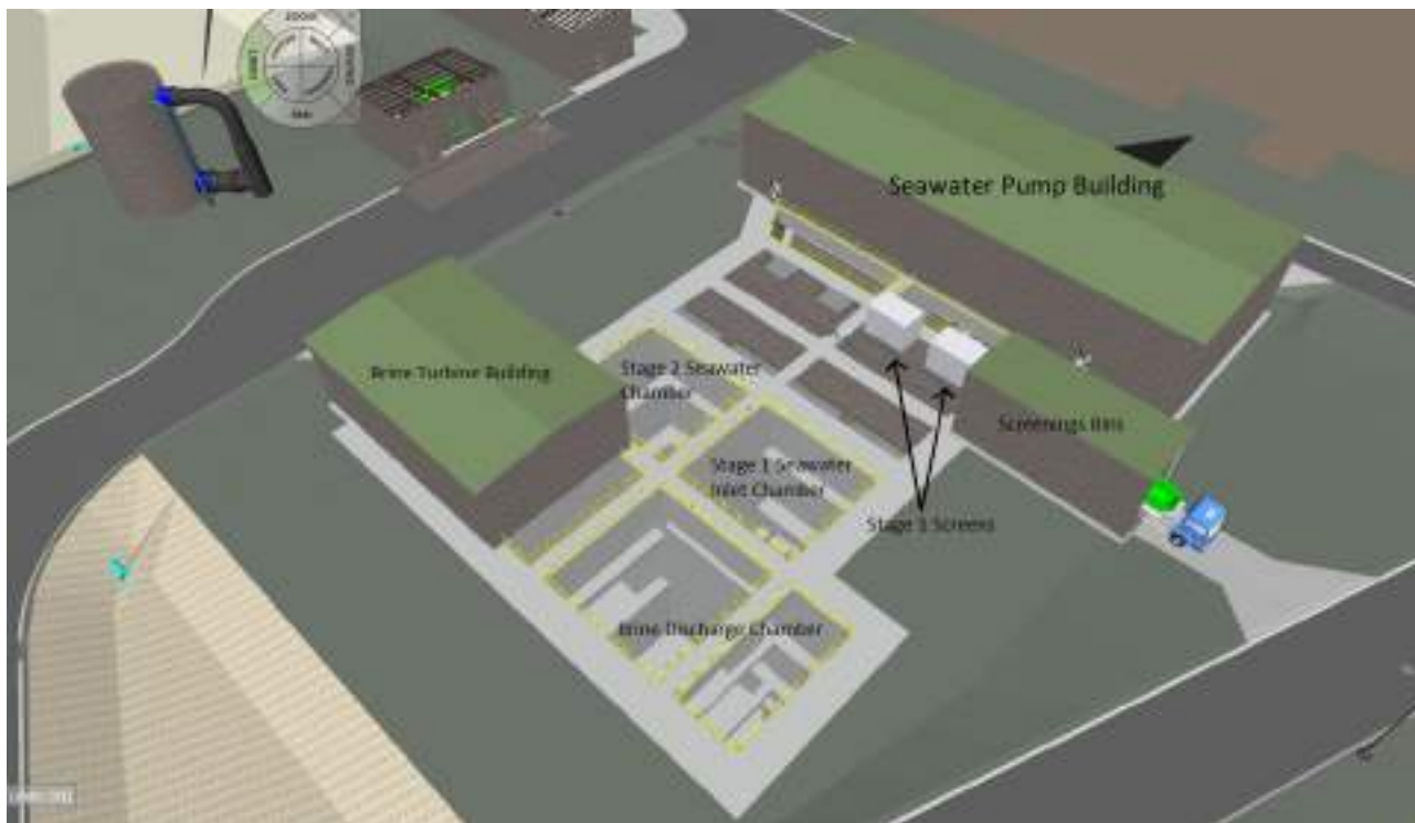
Plate 14 - 3D Model of Seawater Intake Pumping Station (SWIPS) and Brine Discharge Chamber (Northern Water Partnership, 2023)
