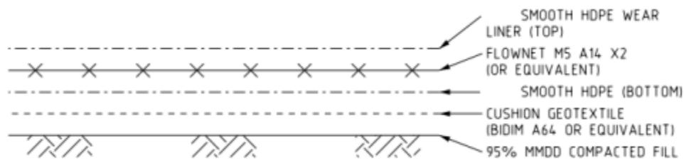
Figure 2: Liner and membrane arrangement and details
