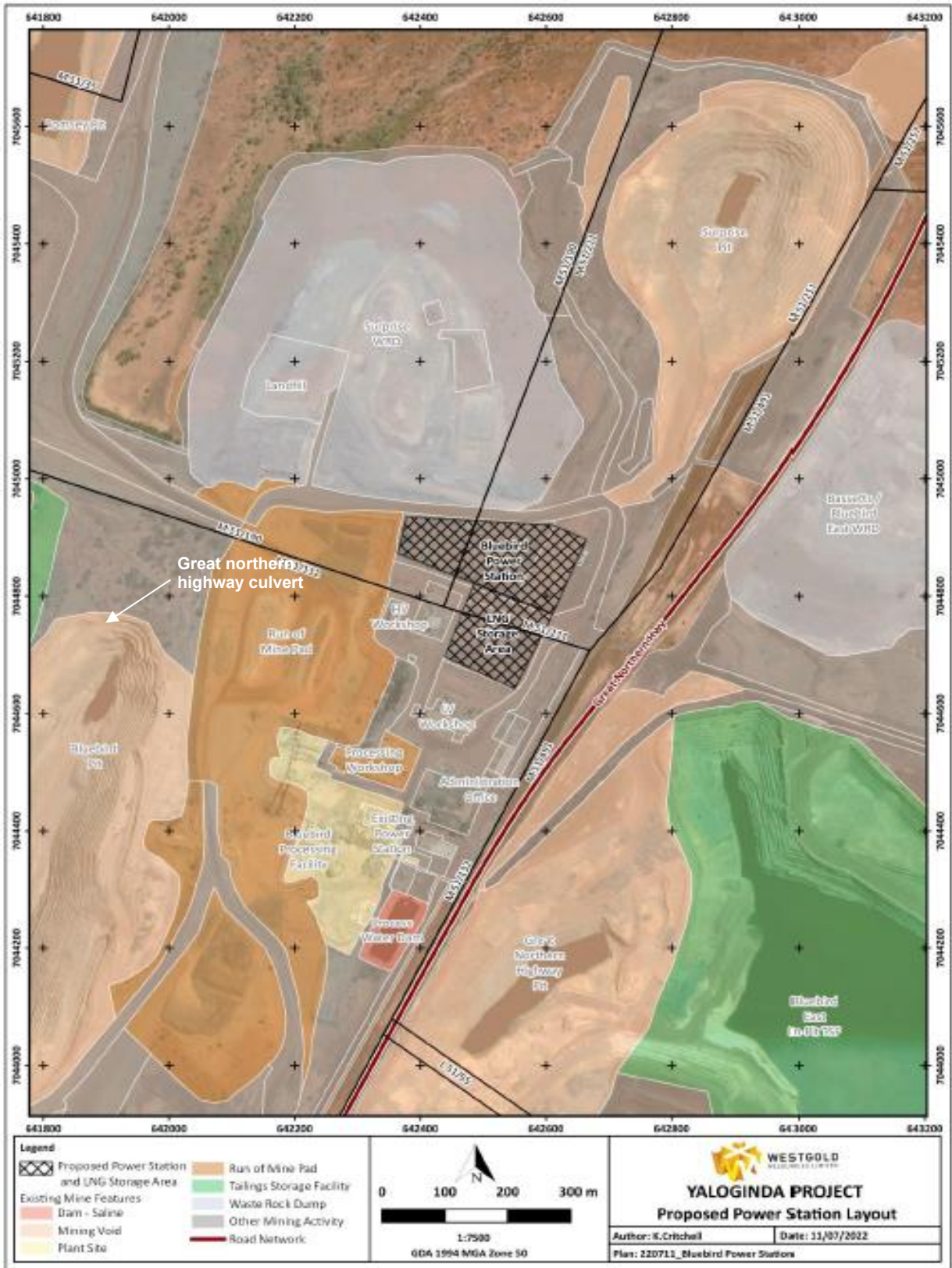
Figure 21: Hybrid Power Generation Facility (Bluebird Power Station) and LNG Storage Area
