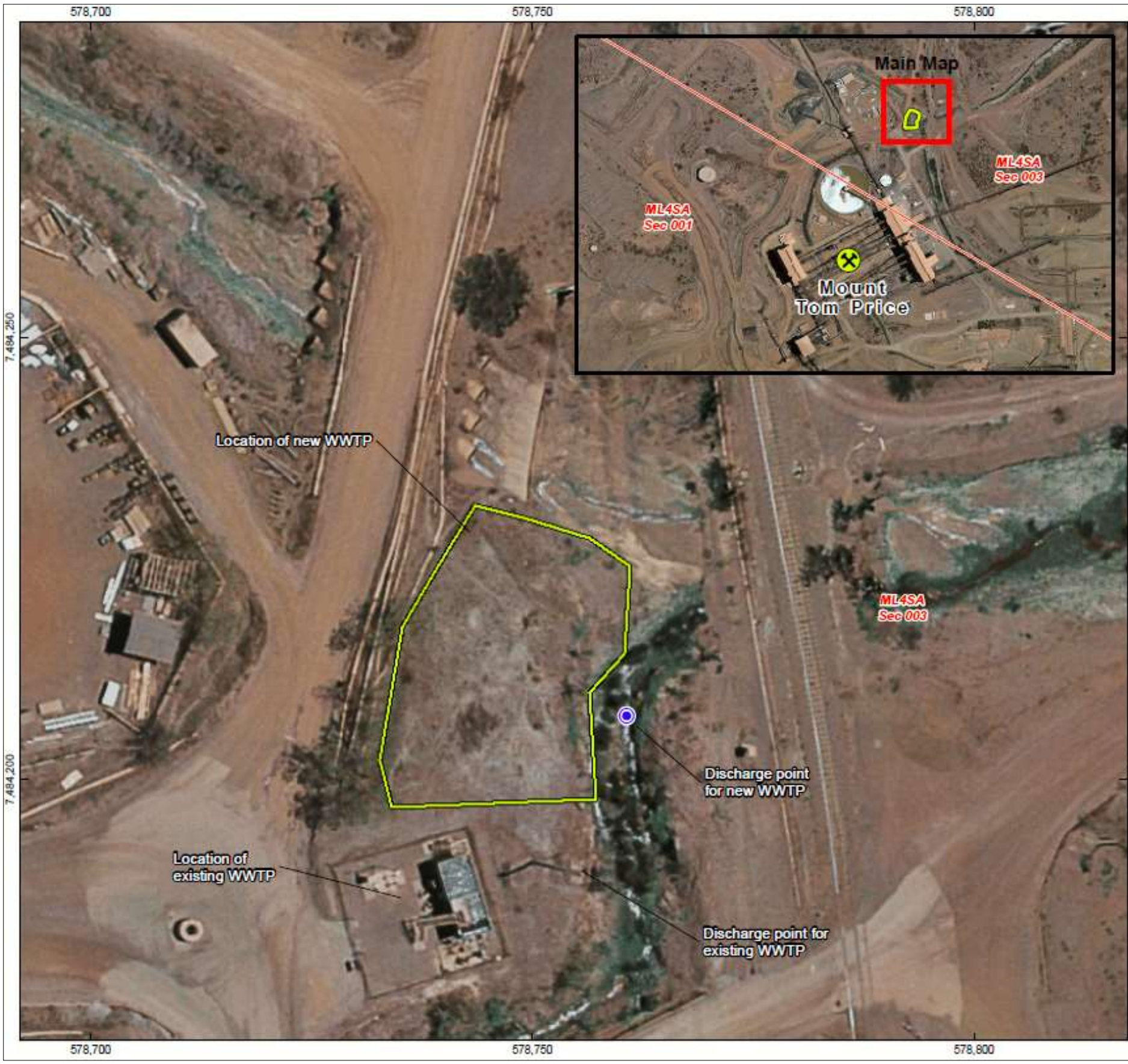
Figure 7: Existing and proposed new discharge point for WWTPs.
