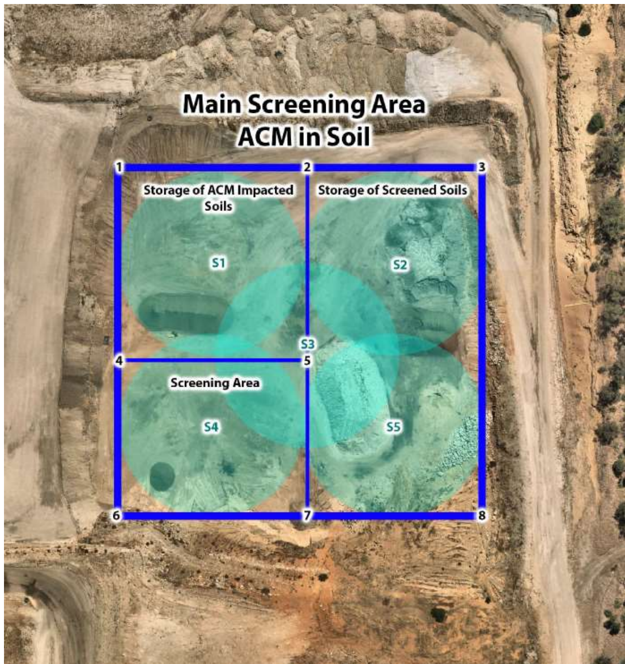
Figure 3: Detailed view of Main Screening Area and layout of dust suppression sprinklers.
