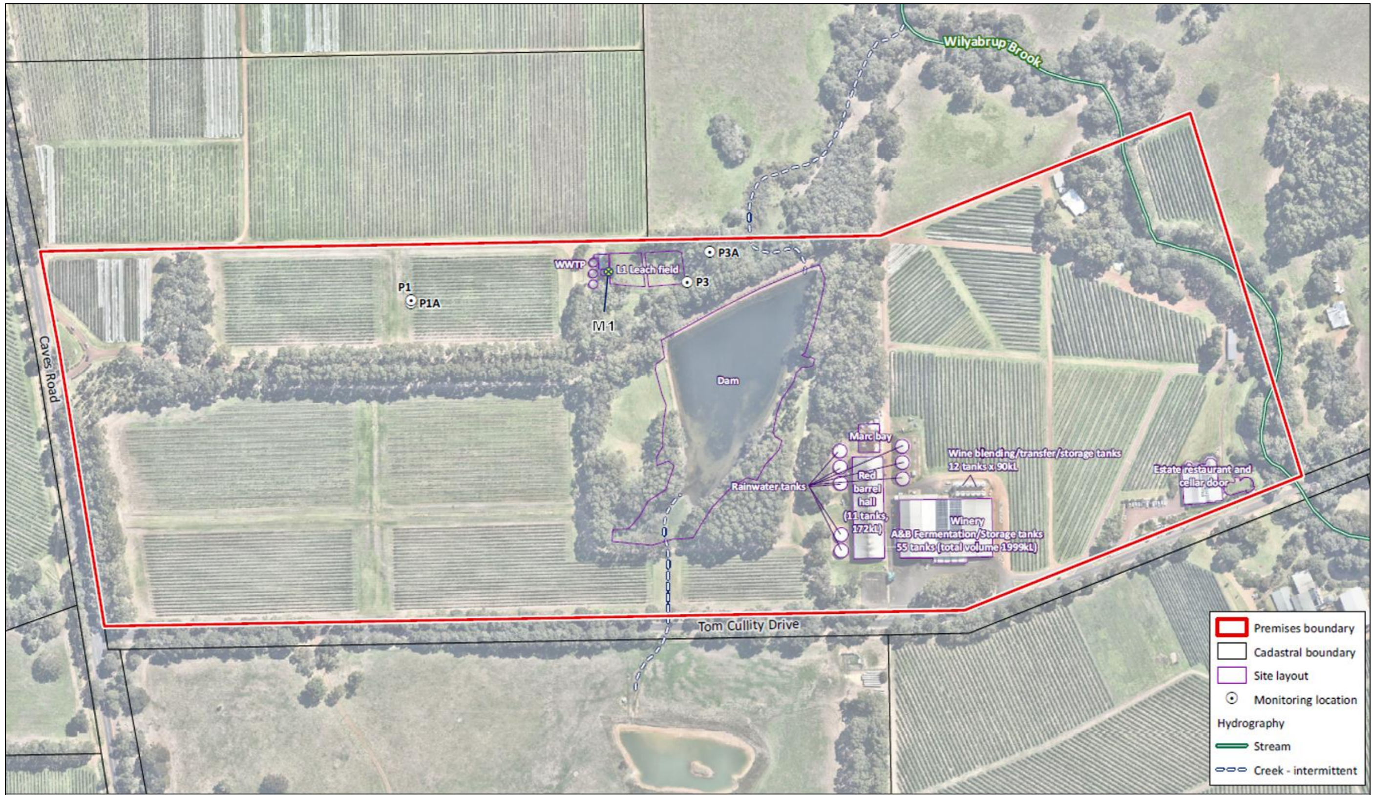
Figure 1: Prescribed premises boundary, monitoring points and key site infrastructure including the winery, red barrel hall, tank farm, marc bay, wastewater treatment plant and leach drain field
