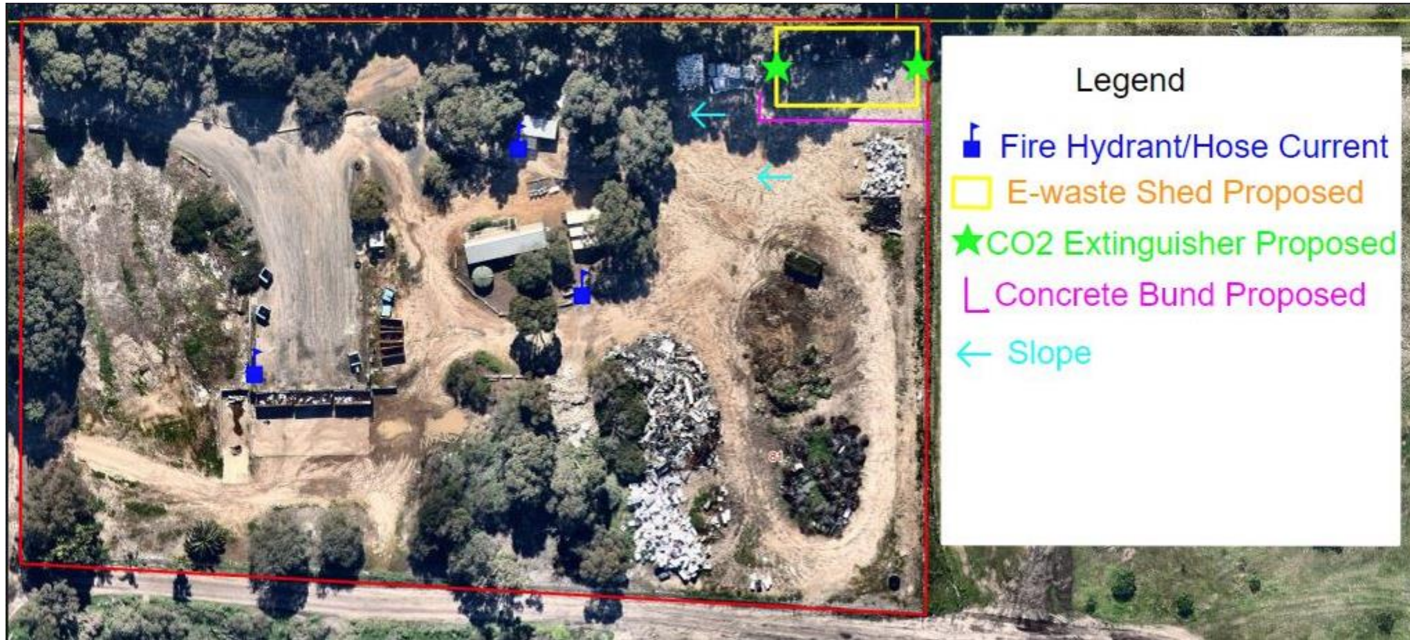
Figure 2: Fire and fire water controls
