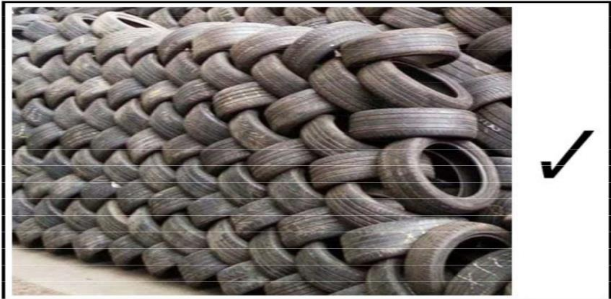
Figure 9: Laced storage of tyres
