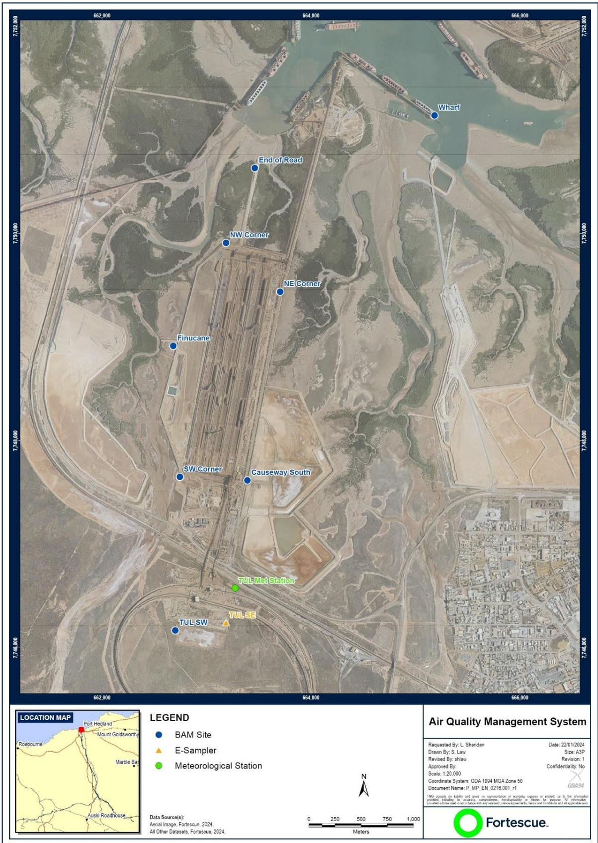
Figure 7: Premises dust monitoring network
