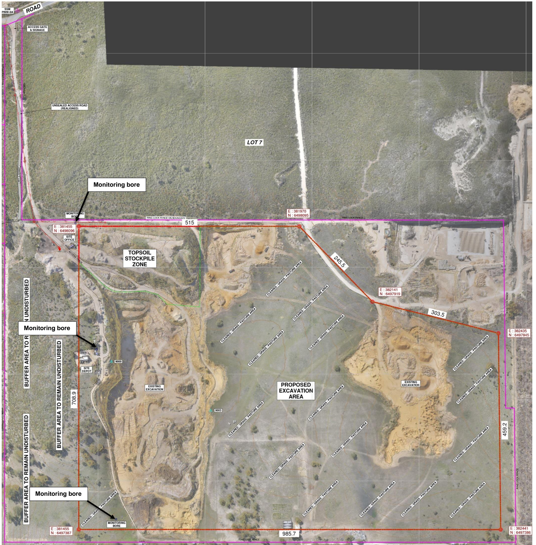
Figure 4: Monitoring bore locations
