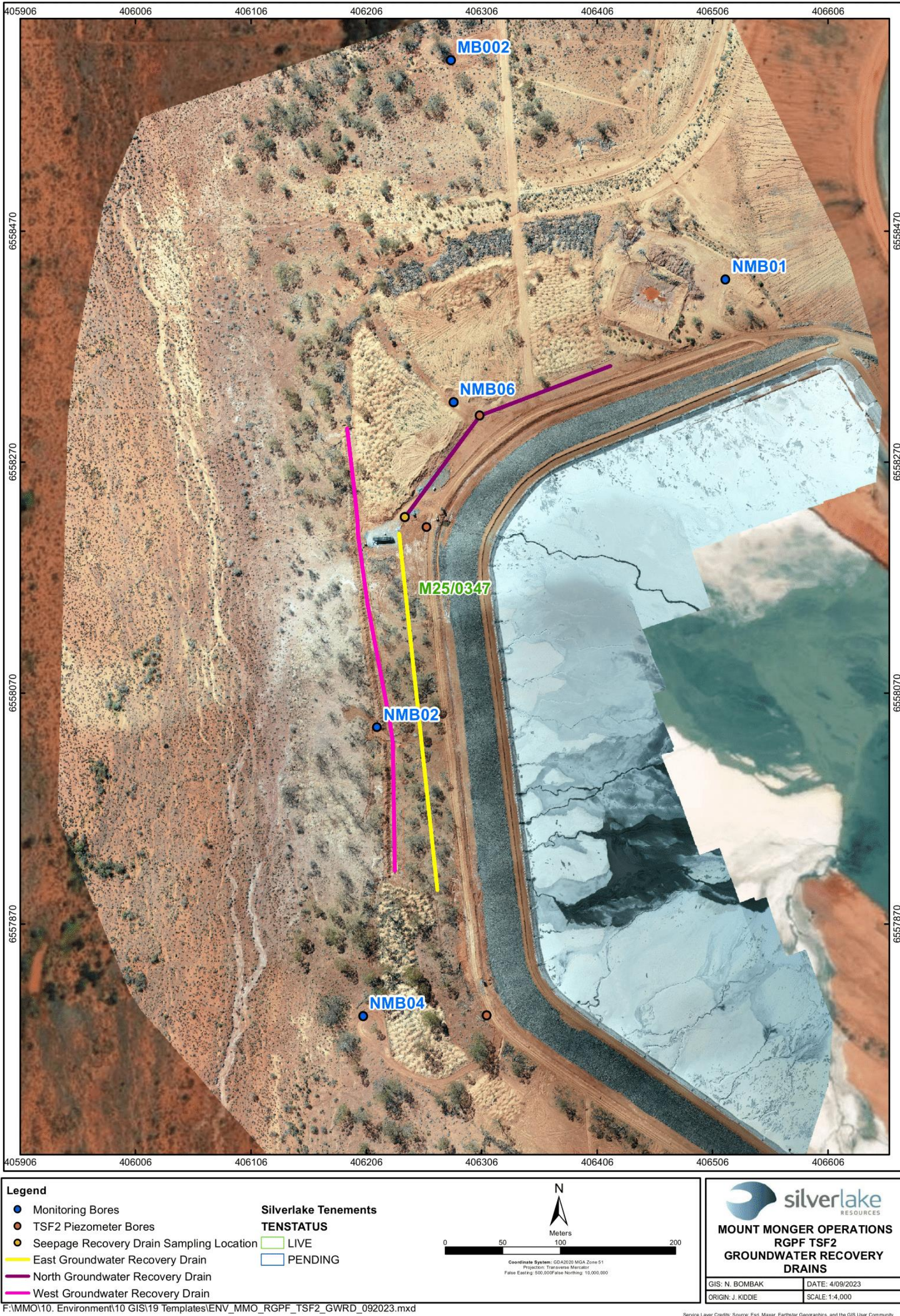
Figure 4: Location of groundwater recovery drains
