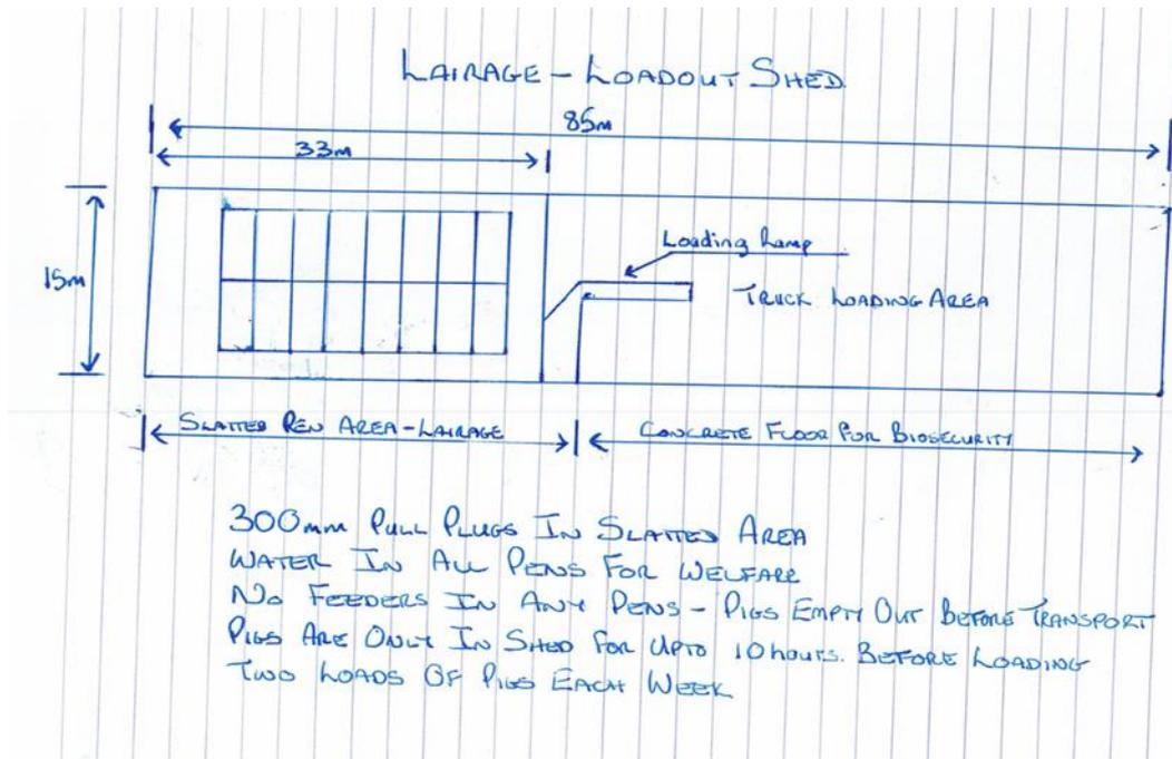
Figure 6: New load out shed design.
