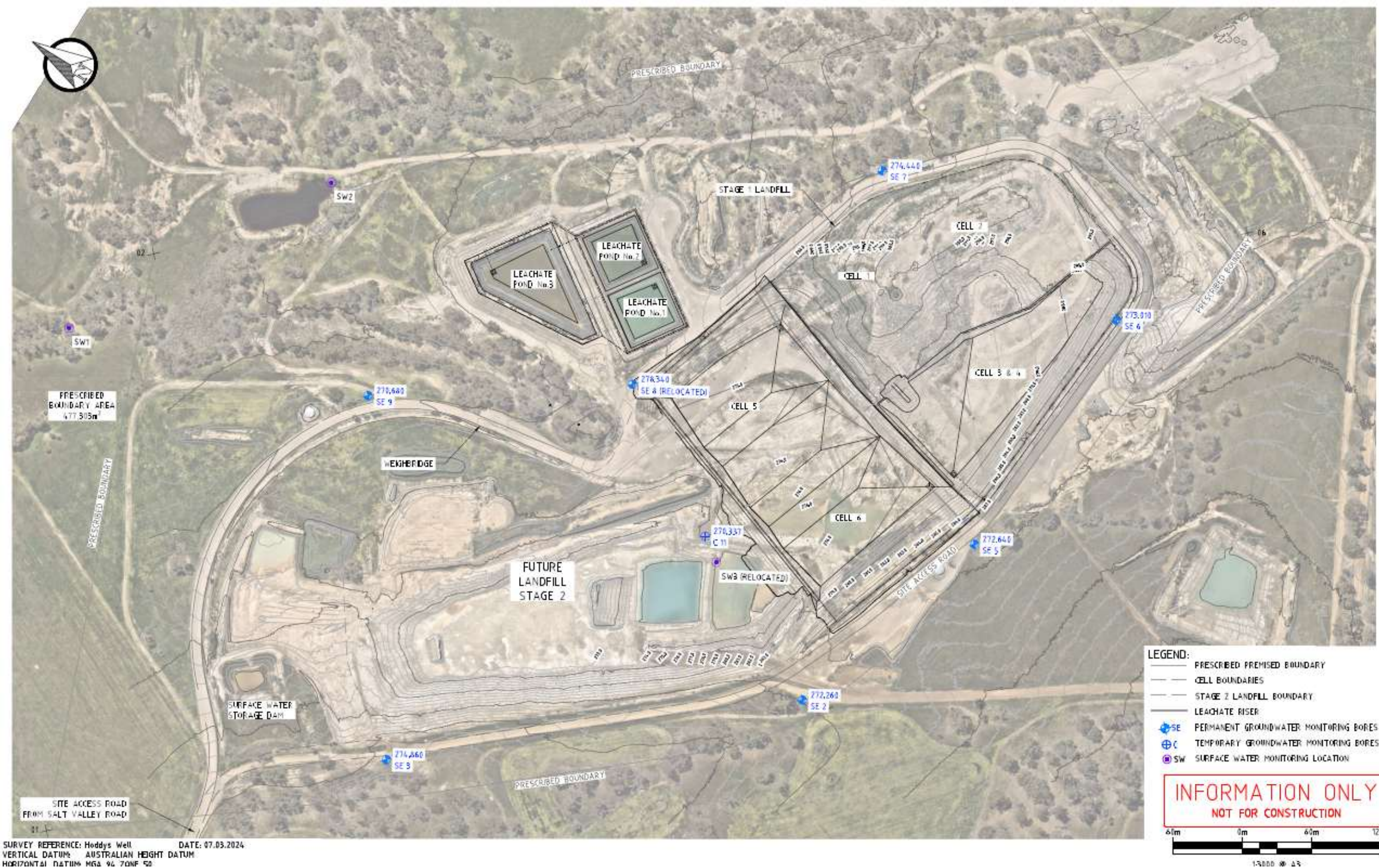
Figure S1-6: Groundwater monitoring well and surface water monitoring network
