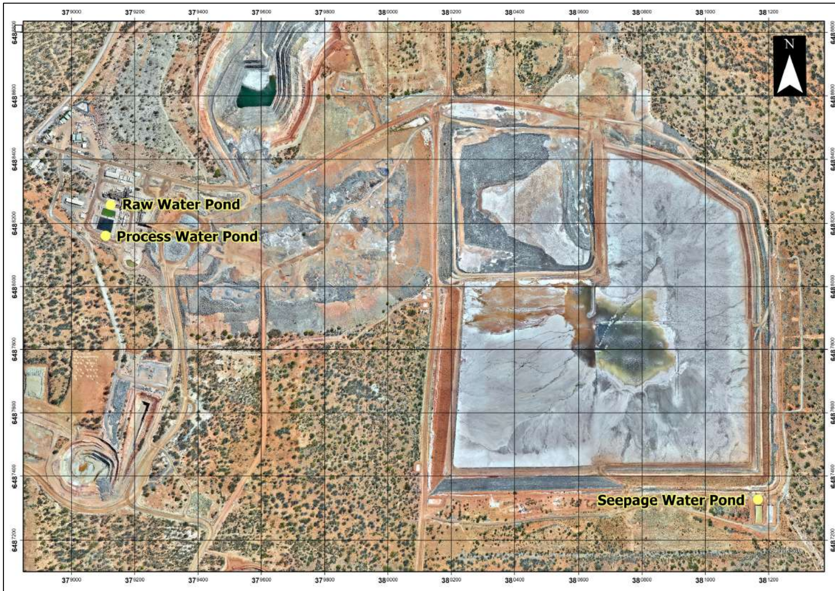
Figure 7: Location of raw water, process water and seepage water ponds in relation to TSF2-4
