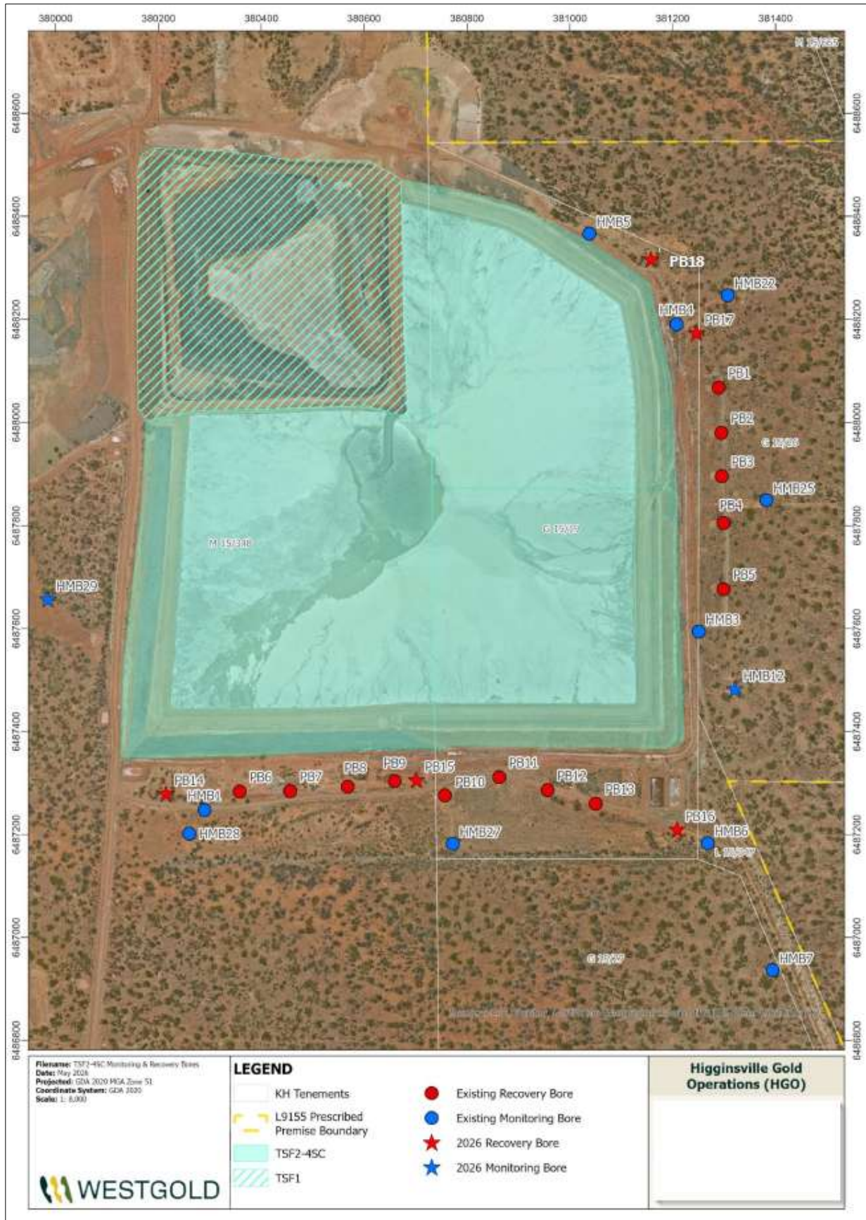
Figure 11: TSF 2-4 monitoring and recovery bores
