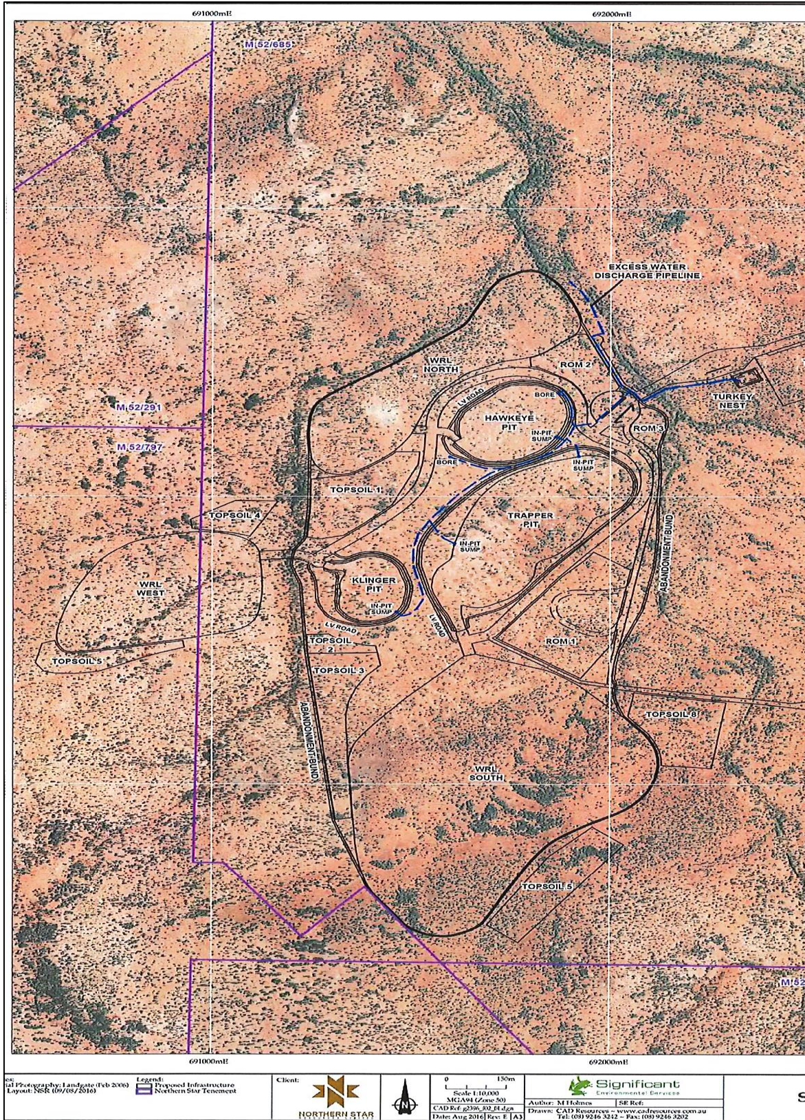
Figure 1: Site layout and excess water discharge pipeline
