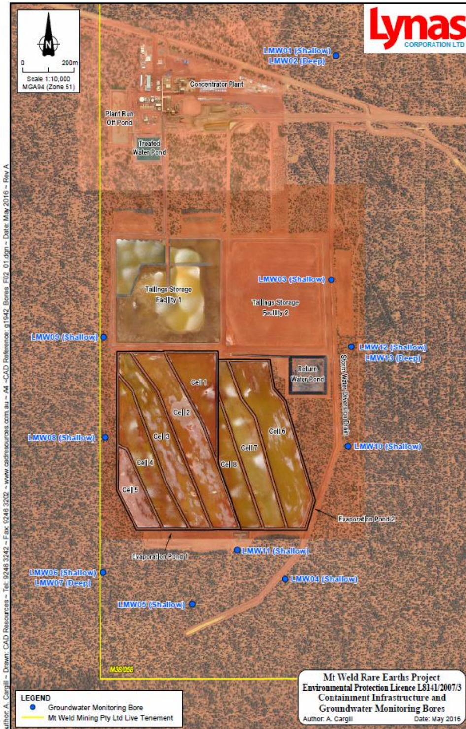
Figure 2: Premises containment infrastructure and groundwater monitoring sites.
