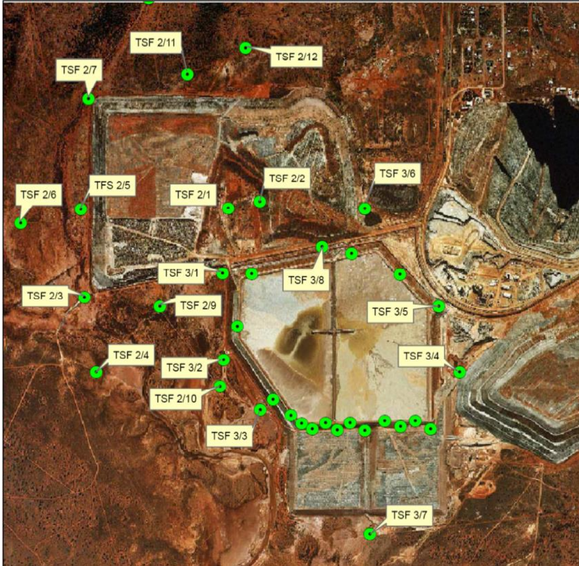
Figure 6: Location of the groundwater monitoring bores surrounding TSF 2 (decommissioned) and active TSF 3.
