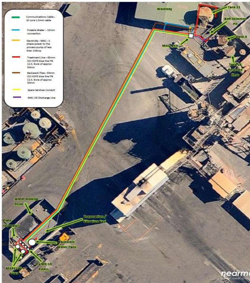
Figure 1: proposed washbay wastewater treatment upgrades layout.
