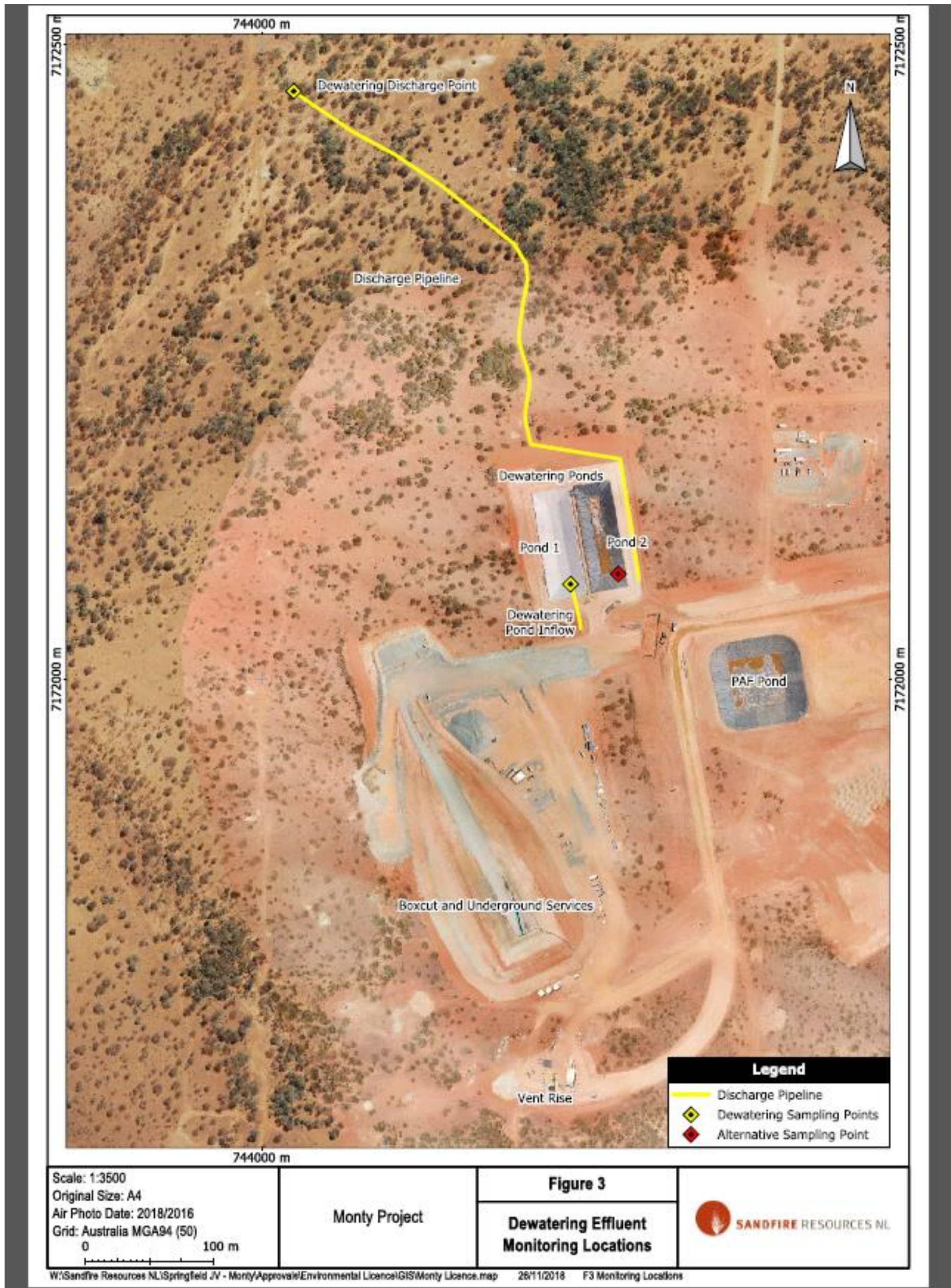
Figure 3 Dewater effluent monitoring locations
