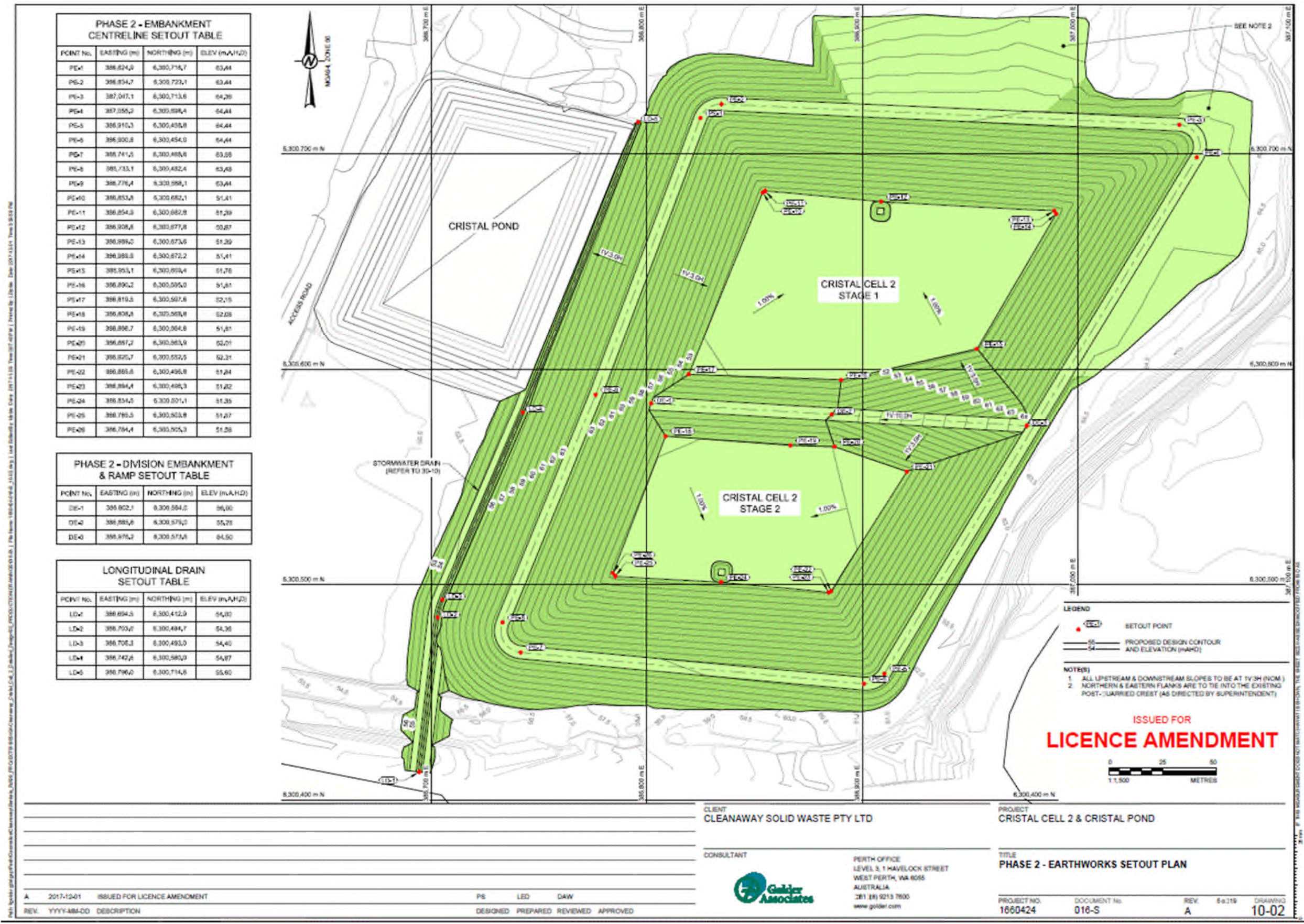
Plan 15: CC2 Stage 1 and Stage 2 earthworks plan (Source: Golder Associates 2017)
