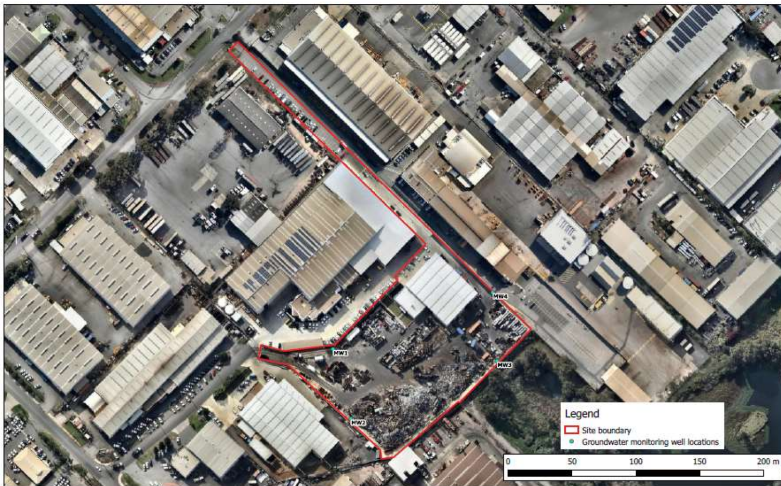
Figure 3: Groundwater monitoring well locations
