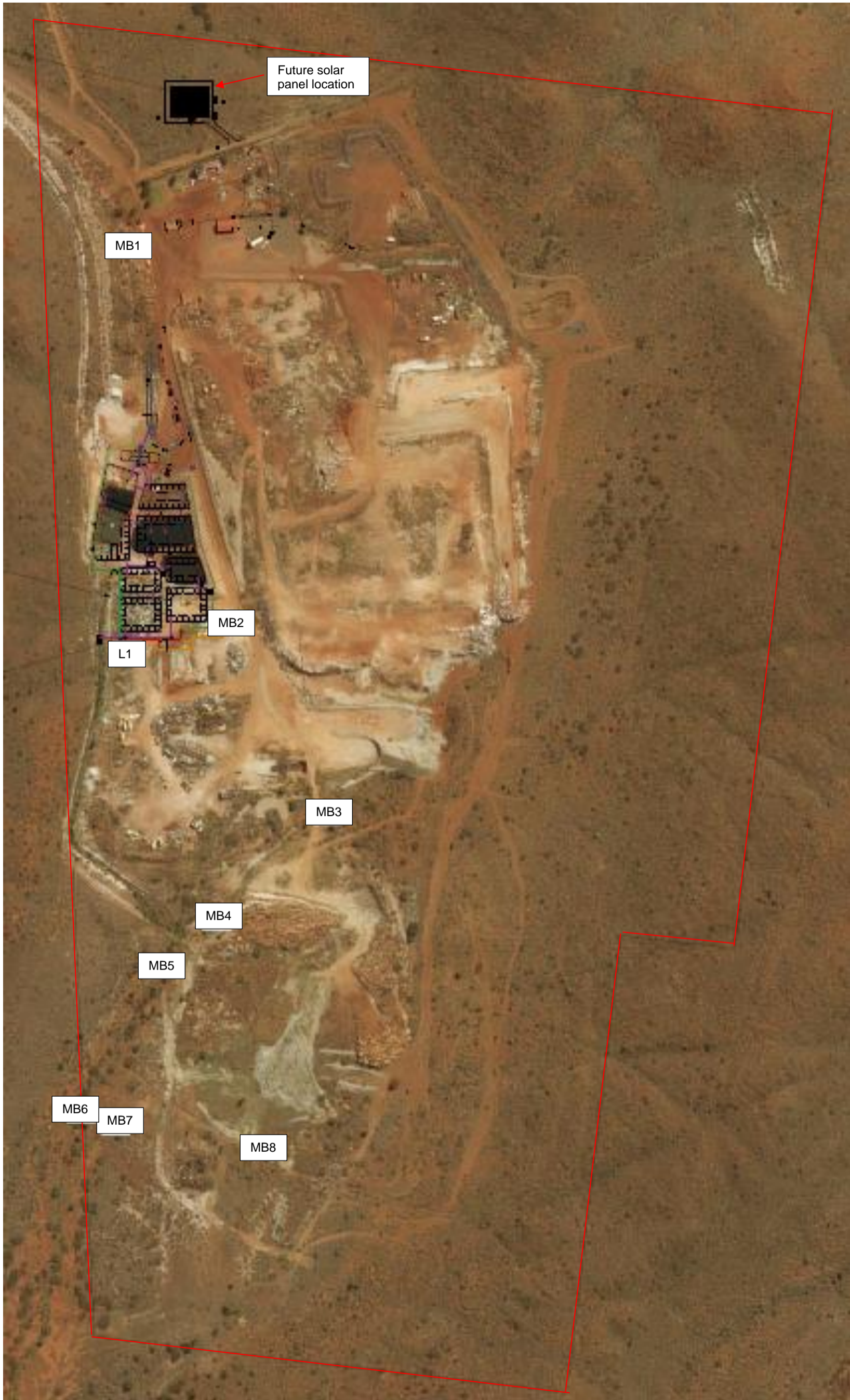
Figure 2: Location of groundwater monitoring bores
