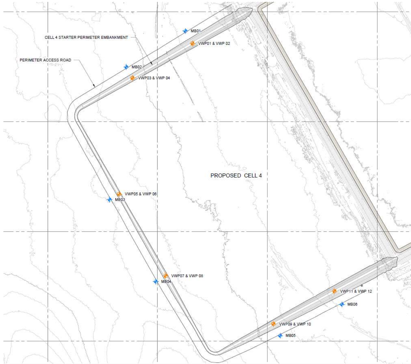
Figure 16: Monitoring bores and piezometers
