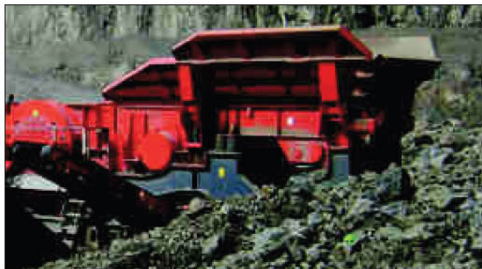
Hopper and Feeder
