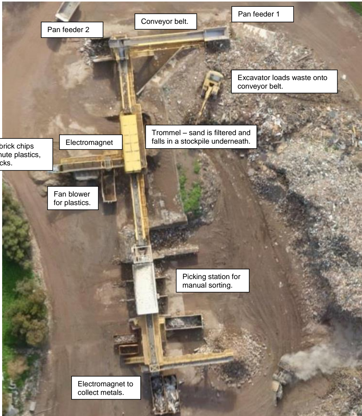
Figure 3: Recycling Station Process
