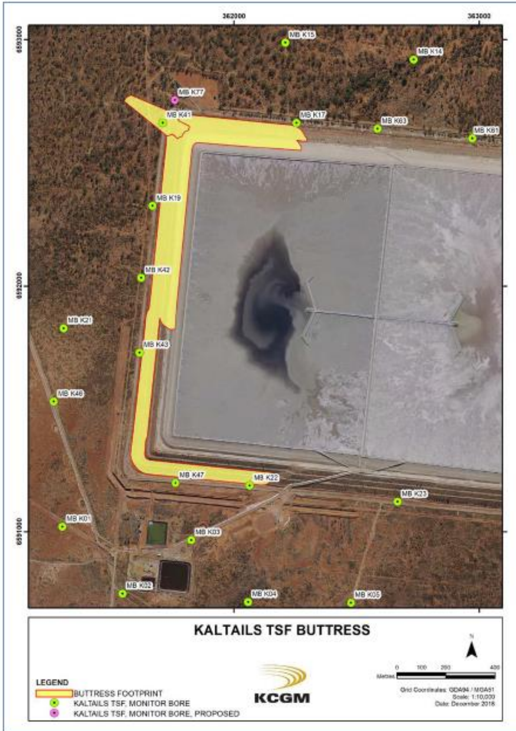
Figure 1: Location of Kaltails TSF buttress and groundwater monitoring bores (new bore MB K77 shown in pink)
