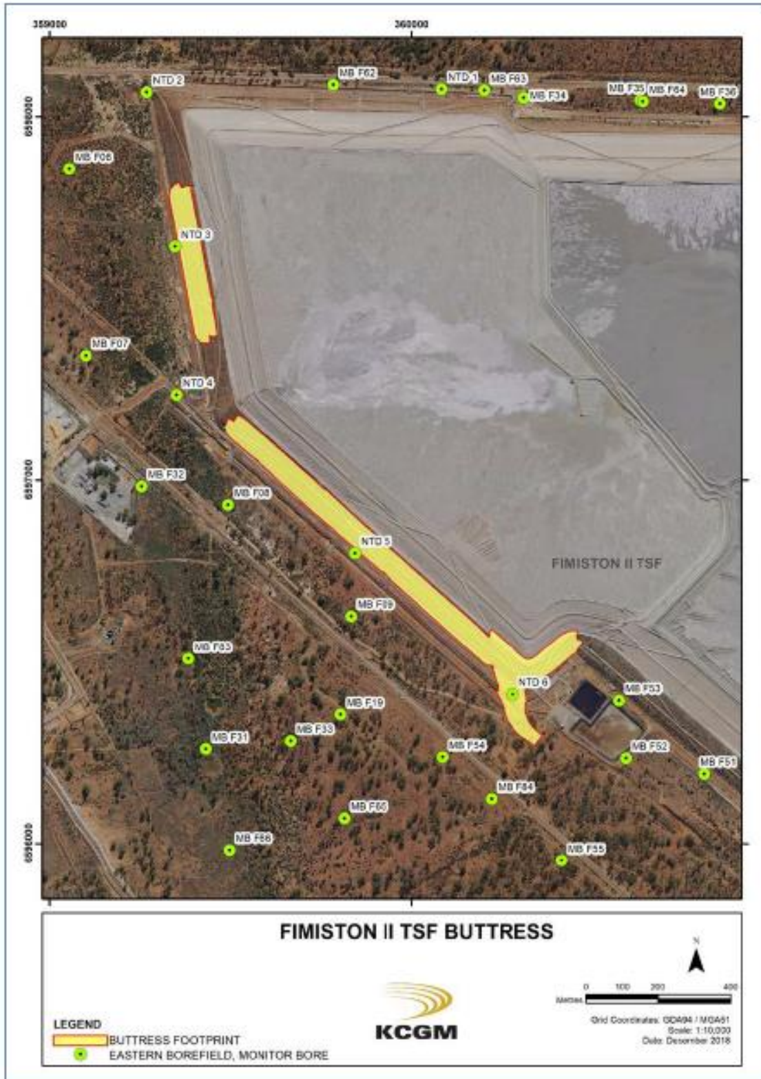
Figure 2: Location of Fimiston II TSF buttress and groundwater monitoring bores
