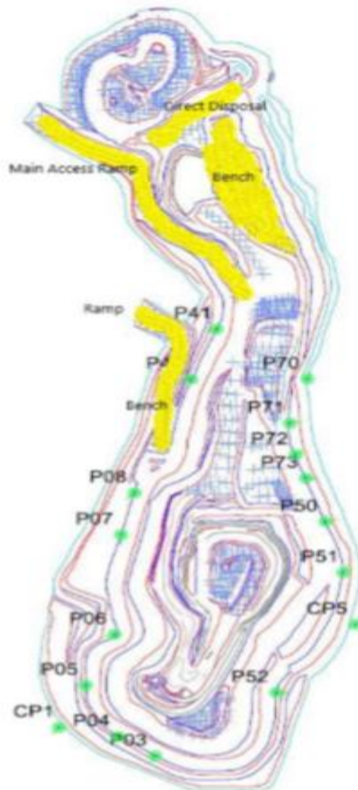
Figure 5: Prism Monitoring and Tyre Disposal Locations
