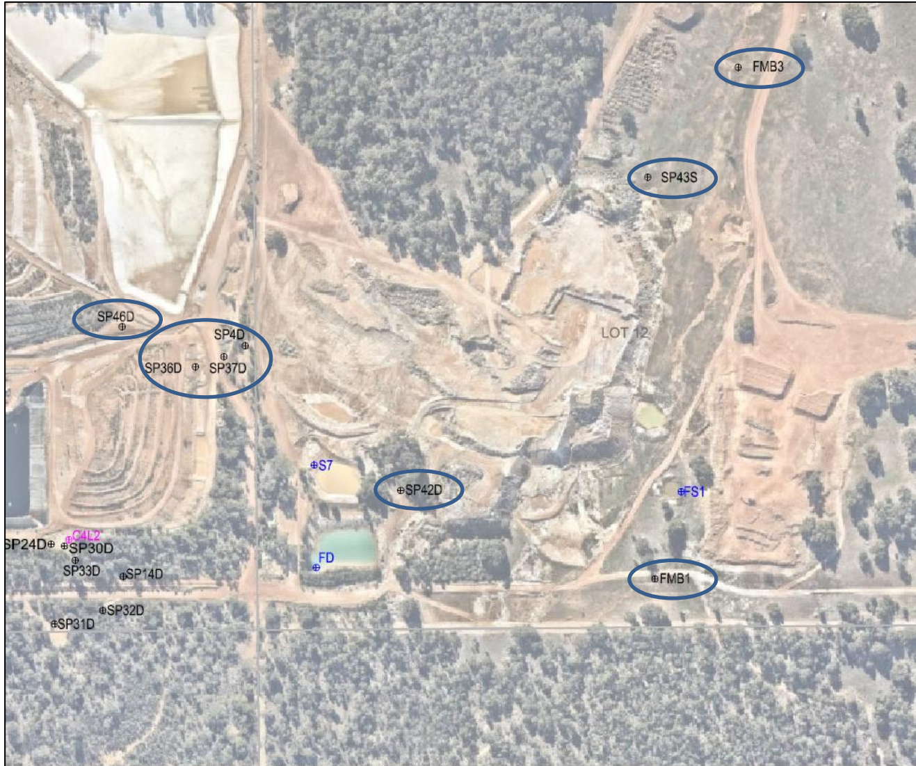
Figure 3: Map of the proposed groundwater monitoring points relating to the proposed leachate ponds - SP43S, FMB1 and FMB3 SP4D, SP36D, SP37D, SP42D and SP46D (Bores in blue circles)
