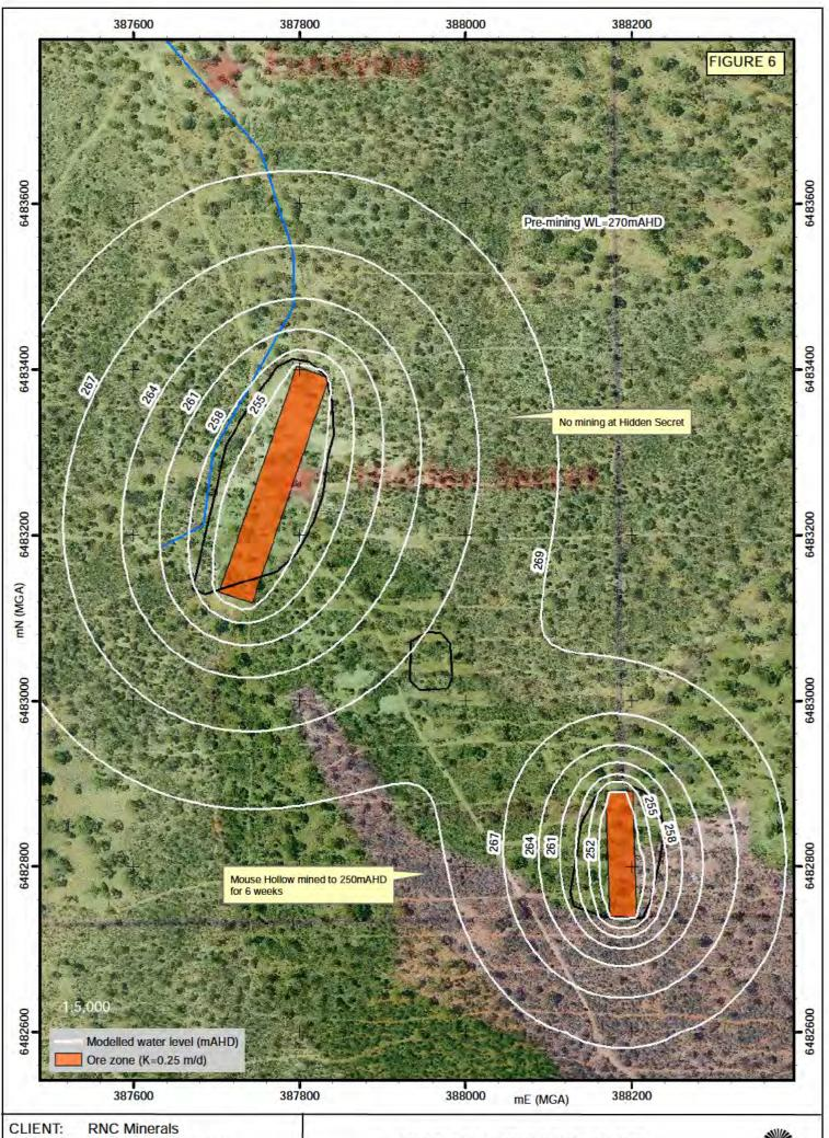
MODELLED WATER LEVEL AT END MINING OF MOUSE HOLLOW PIT
