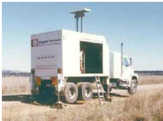
Figure 2: Purpose built CPT rig
