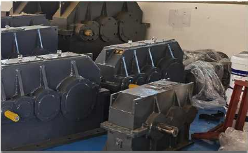
ZSY reducer is adopted, with low noise and stable output
