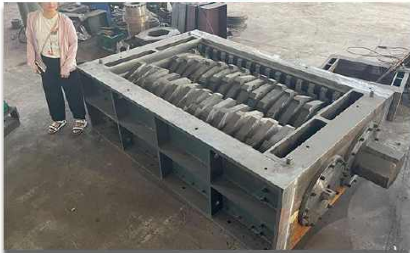
The wallboard is thickened, which will not deform after long-term use and is more durable
