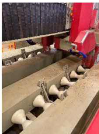
Saw to cut armour wire
