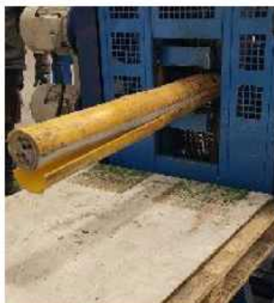
Removal of outer sheath
