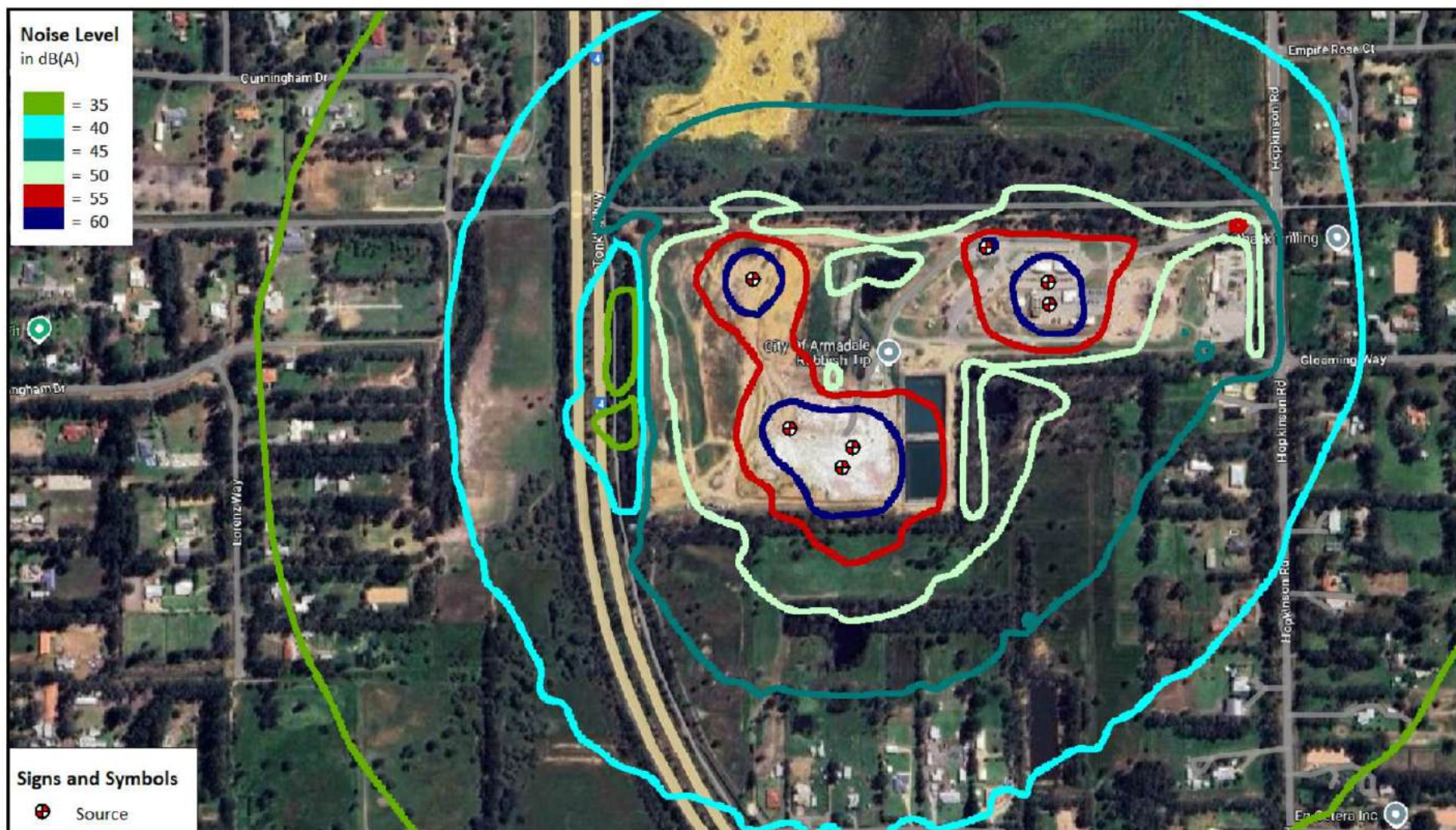
Figure 8: Worst-case noise level contours for the dozer replaced by a loader in scenario 1.
