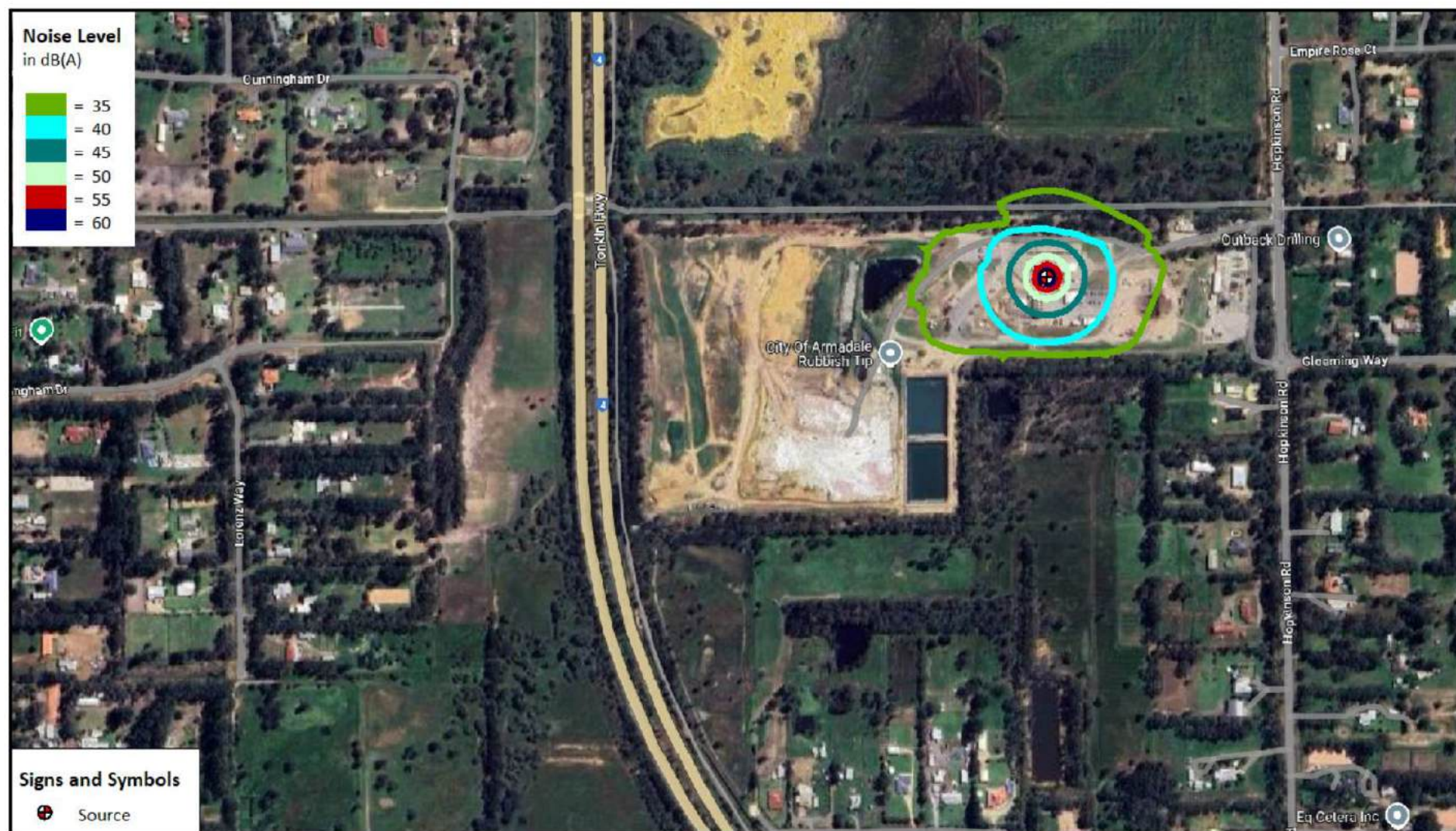
Figure 7: Worst-case noise level L_{A\text{Max}} contours for scenario 4.
