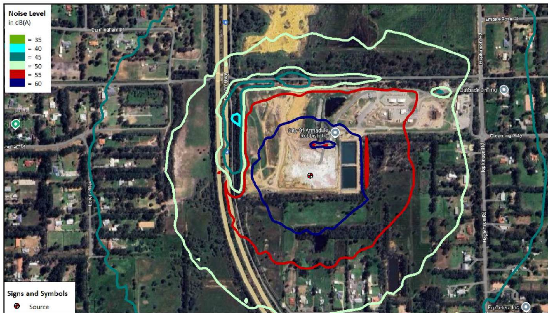
Figure 6: Worst-case noise level L_{A_{Max}} contours for scenario 3.
