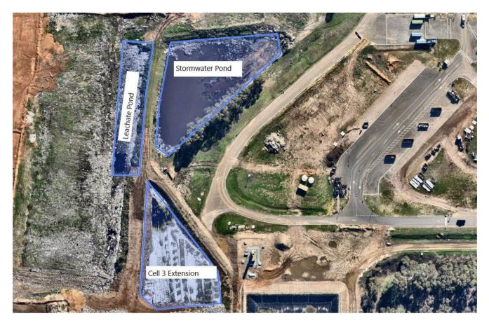
Leachate pond is used for collection of leachate and Stormwater pond is used for stormwater collection.
