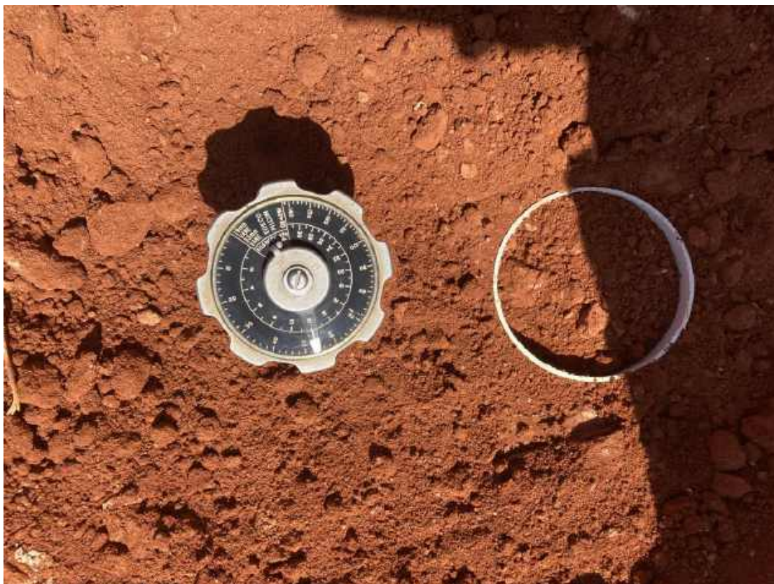
Plate 8: Field Shear test next to UD sample location at North embankment Cut-off trench (3.0m depth)
