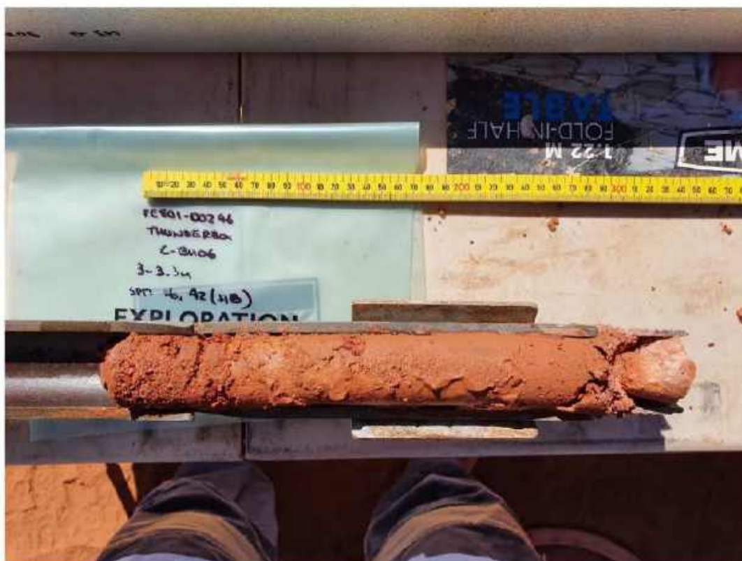
Plate 38: C-BH06 – SPT at 3.0 m
