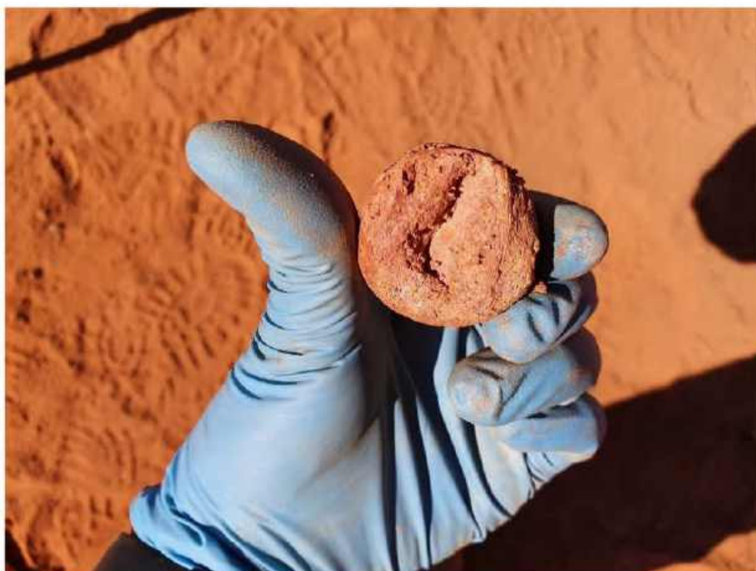
Plate 54: C-BH06 – SPT at 15.0 m
