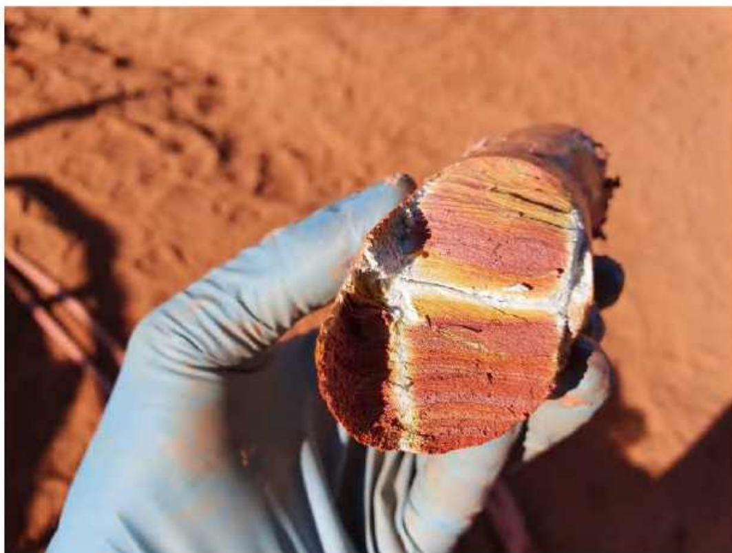
Plate 56: C-BH06 – SPT at 18.0 m
