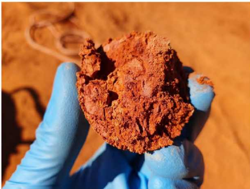
Plate 39: C-BH06 – SPT at 3.0 m
