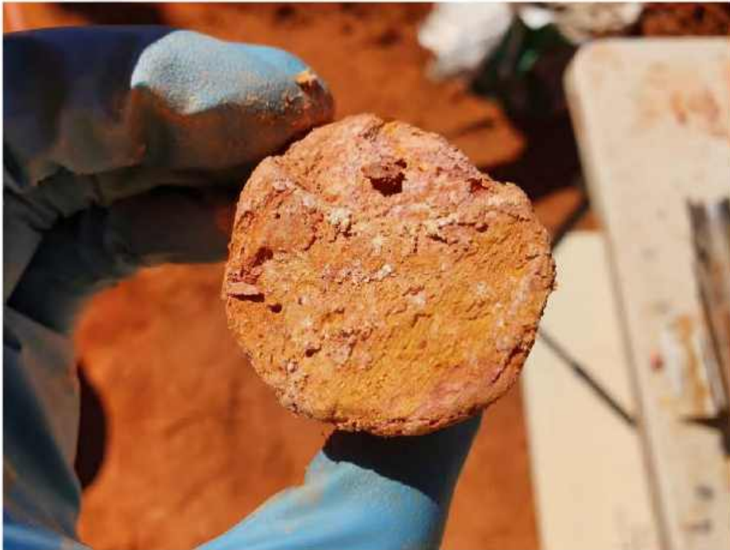
Plate 51: C-BH06 – SPT at 12.0 m
