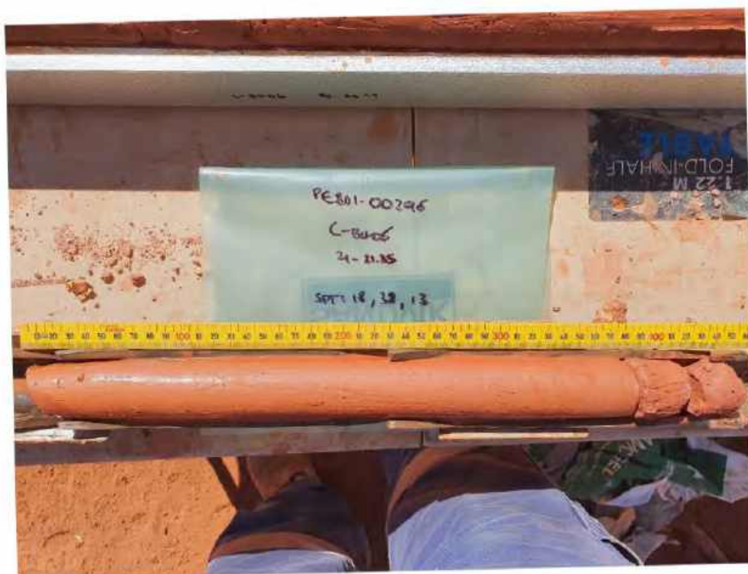
Plate 58: C-BH06 – SPT at 21.0 m
