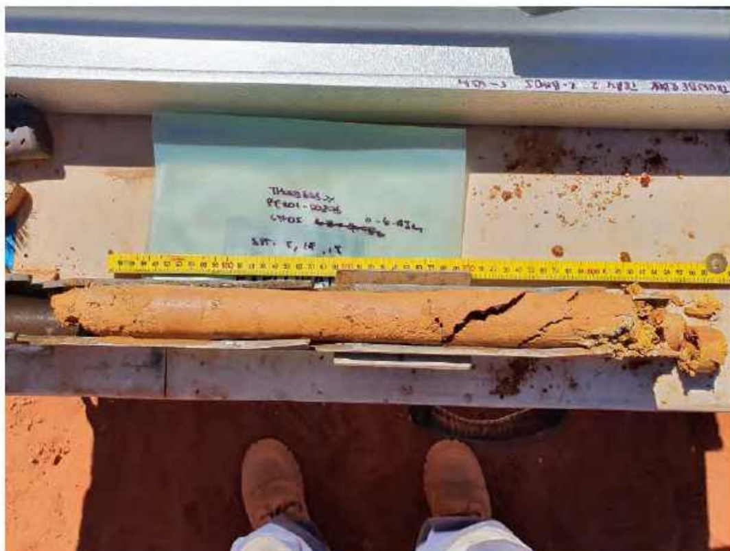
Plate 12: C-BH05 – SPT at 6.0 m
