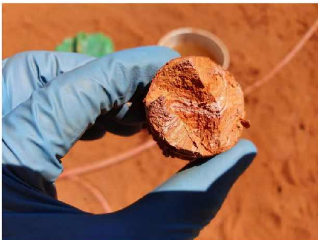
Plate 46: C-BH06 – SPT at 7.5 m
