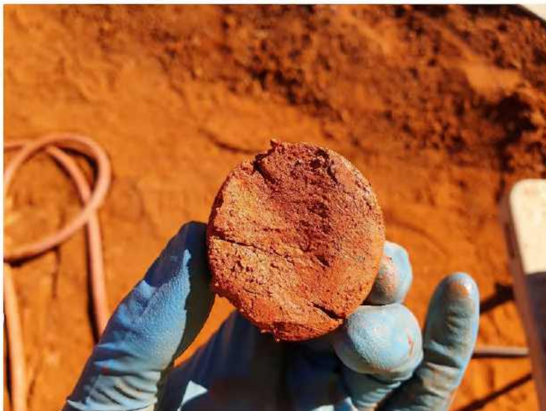
Plate 59: C-BH06 – SPT at 21.0 m
