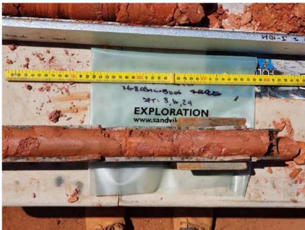
Plate 45: C-BH06 – SPT at 7.5 m
