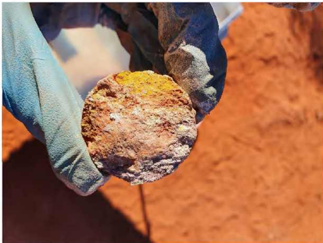
Plate 18: C-BH05 – SPT at 12.25 m
