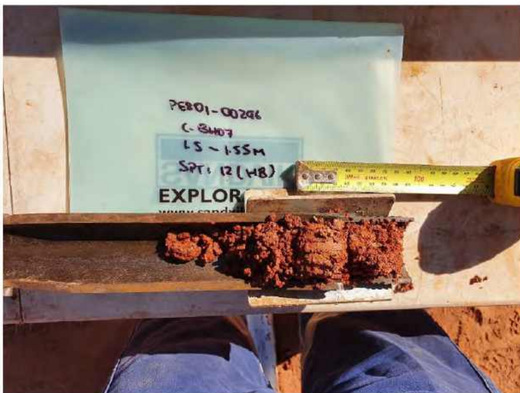
Plate 70: C-BH07 – SPT at 1.5 m
