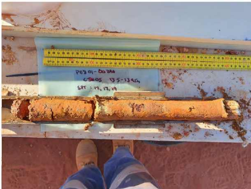
Plate 19: C-BH05 – SPT at 13.5 m
