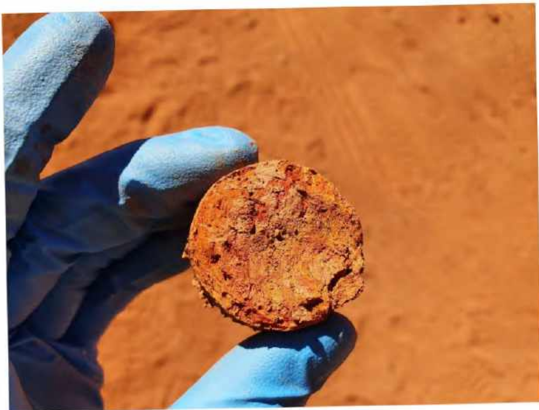
Plate 25: C-BH05 – SPT at 18.0 m
