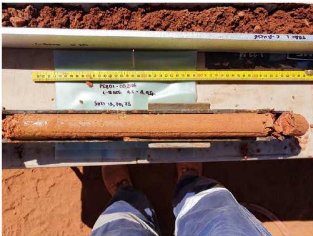
Plate 40: C-BH06 – SPT at 4.5 m
