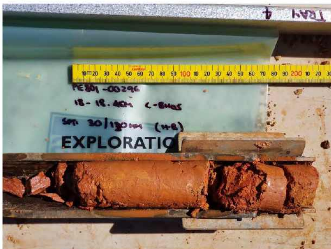
Plate 24: C-BH05 – SPT at 18.0 m
