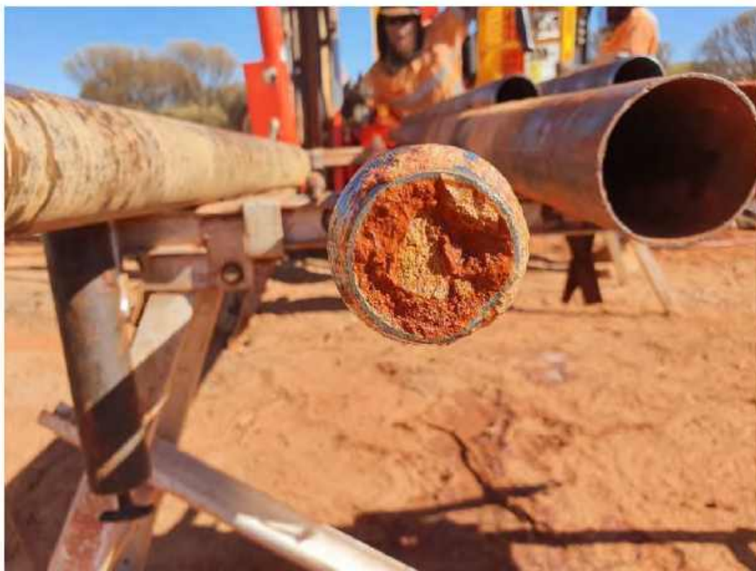
Plate 71: C-BH07 – SPT at 1.5 m
