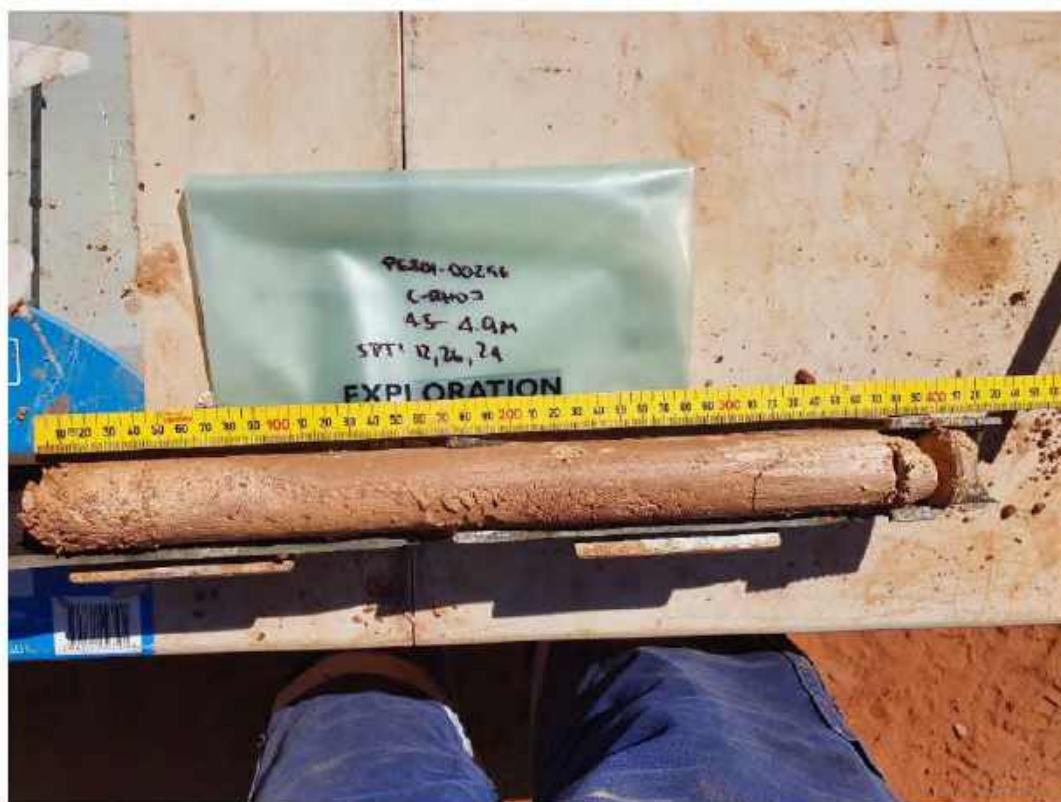
Plate 74: C-BH07 – SPT at 4.5 m
