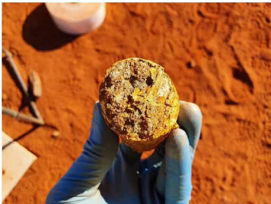
Plate 23: C-BH05 – SPT at 15.0 m
