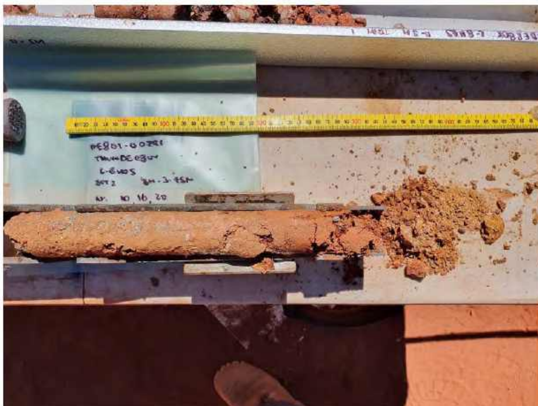
Plate 7: C-BH05 – SPT at 3.0 m
