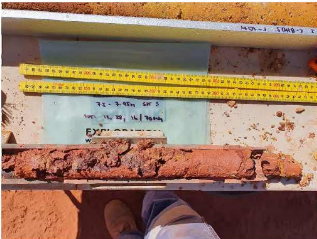
Plate 14: C-BH05 – SPT at 7.5 m
