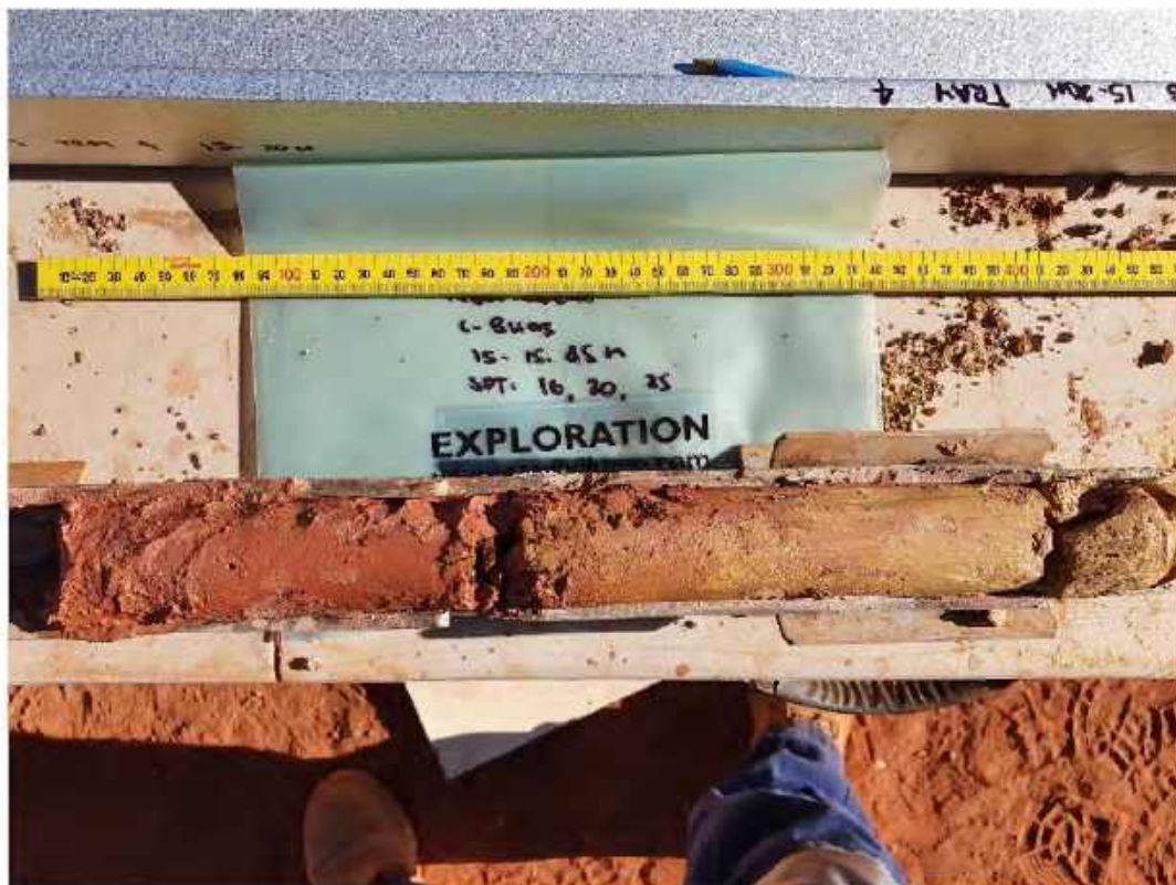
Plate 22: C-BH05 – SPT at 15.0 m
