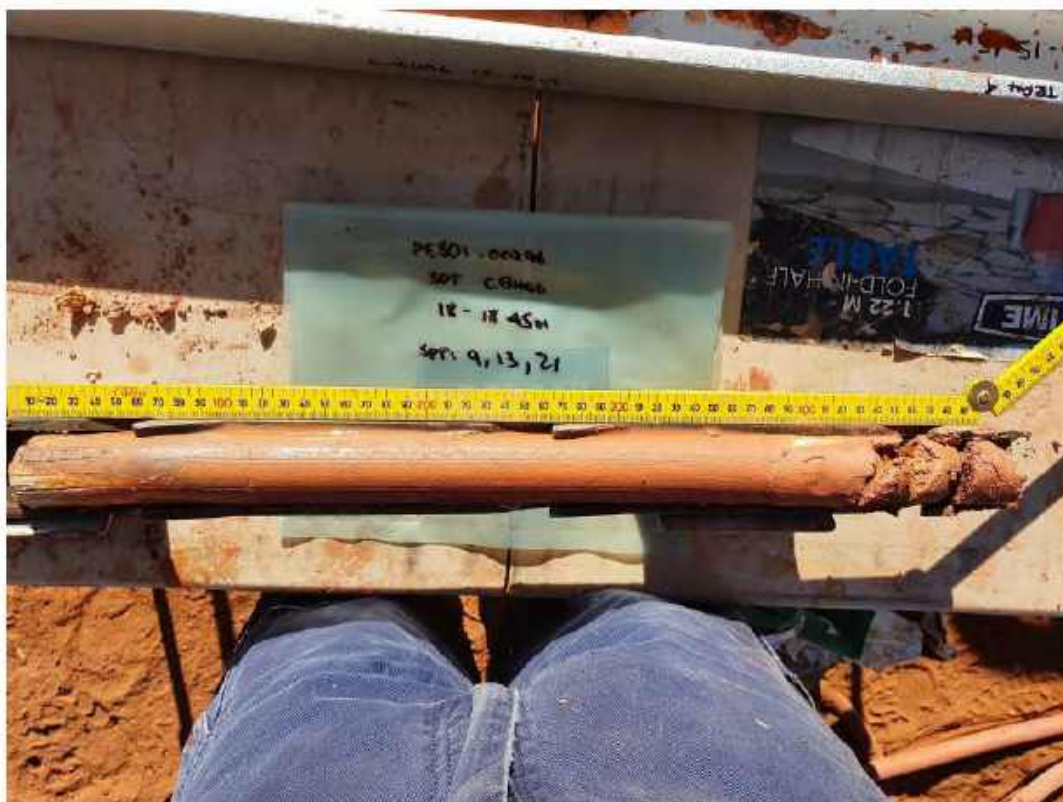
Plate 55: C-BH06 – SPT at 18.0 m
