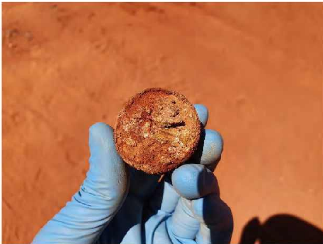
Plate 30: C-BH05 – SPT at 24.0 m
