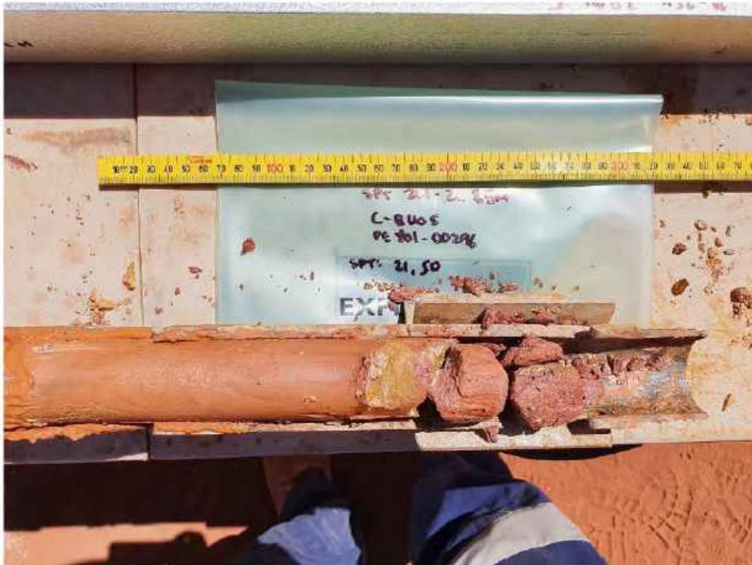
Plate 27: C-BH05 – SPT at 21.0 m
