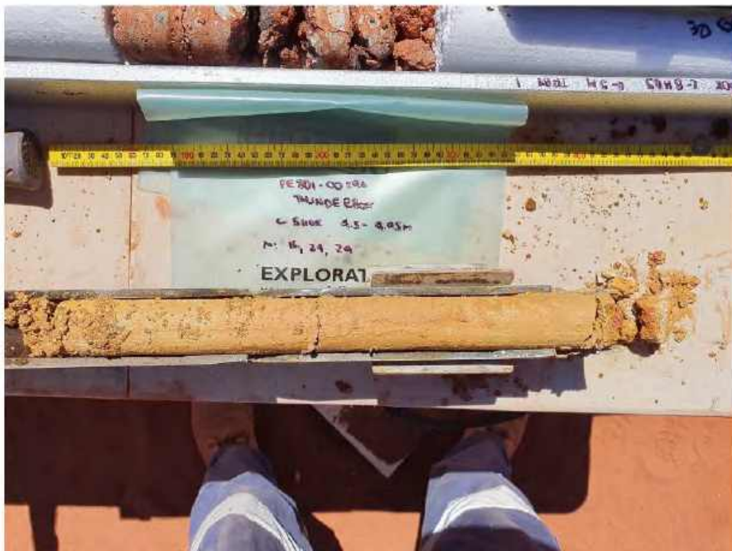
Plate 9: C-BH05 – SPT at 4.5 m
