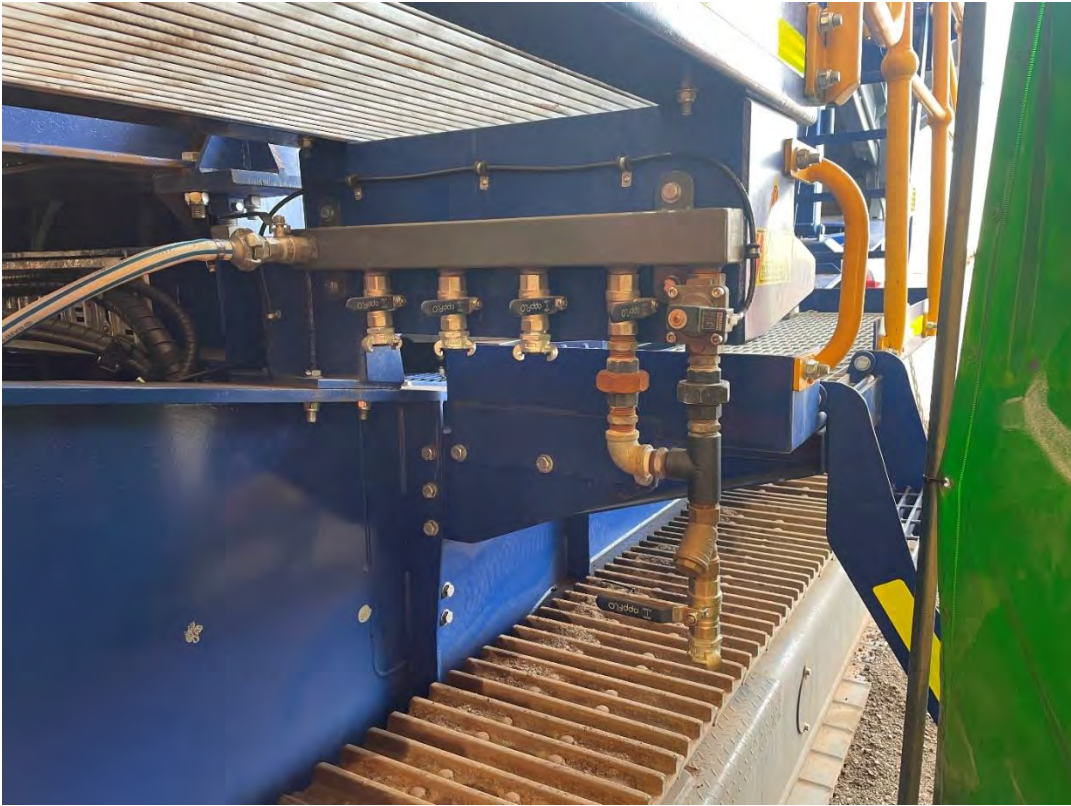
Figure 15 - Dust suppression sprays on Terex Pegson Maxtrak 1300 (secondary cone crusher) used on Sites C and F
