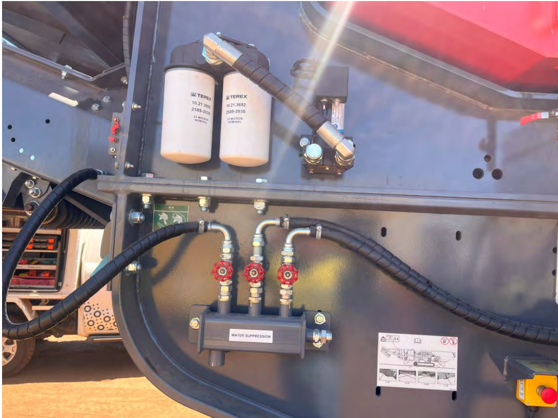
Figure 18 - Striker JM1310 Metso C125 (primary jaw crusher) Dust suppression Manifold used on Site C
