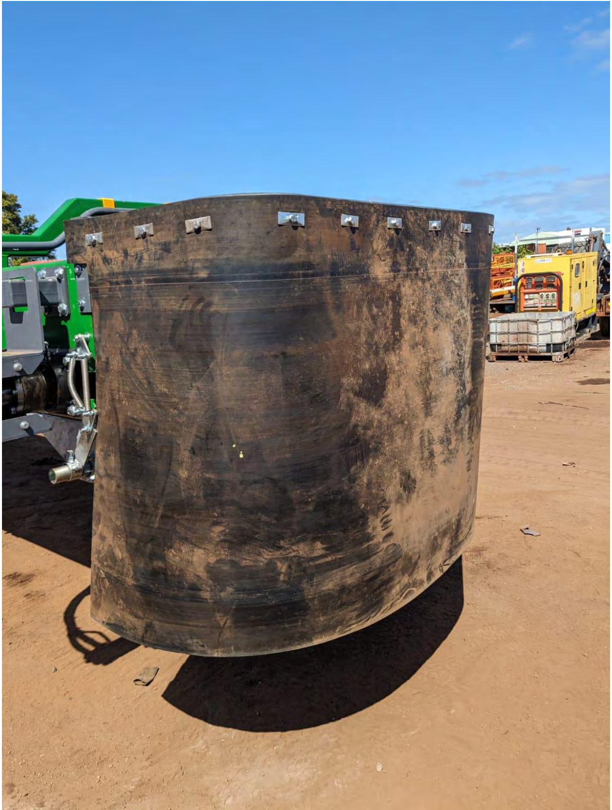
Figure 21 - KES 8048 Stacker Transfer Chute with dust sprays used on both Site C and F Site F
