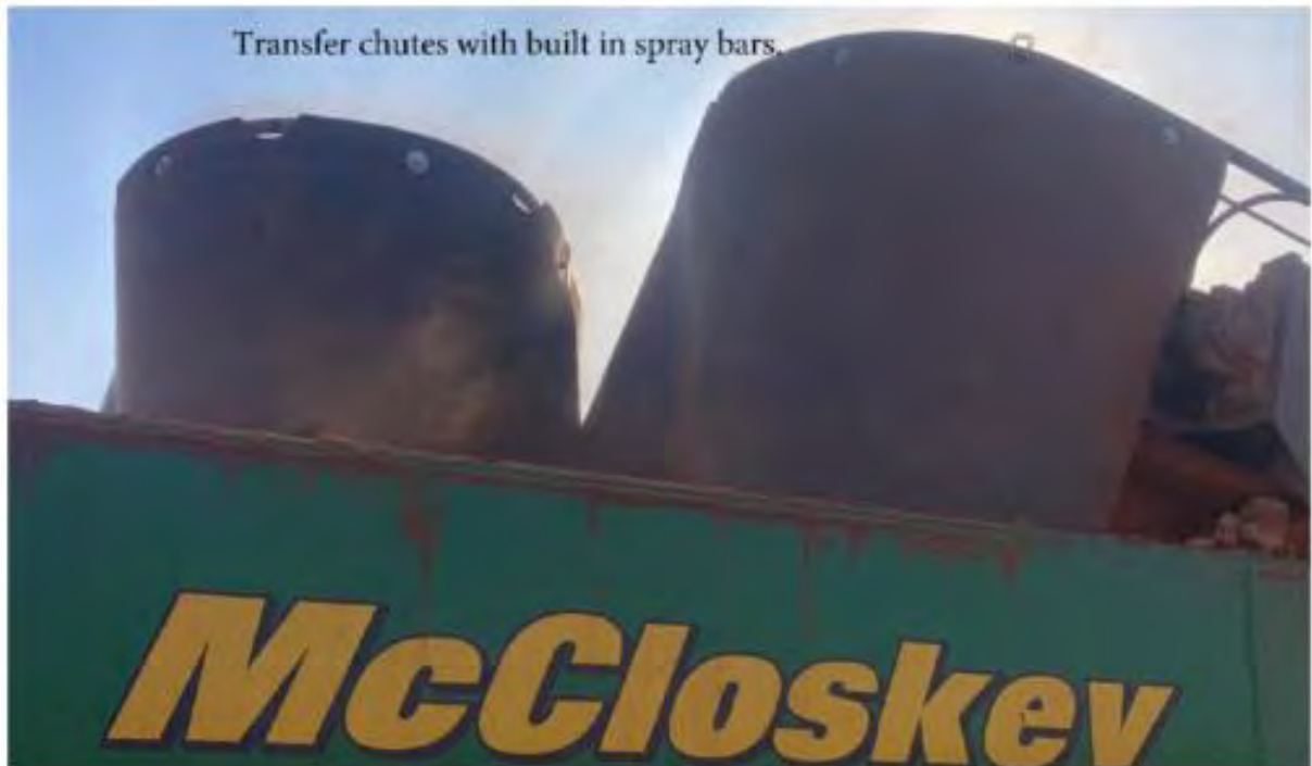
Figure 31 - Transfer points with dust controls
