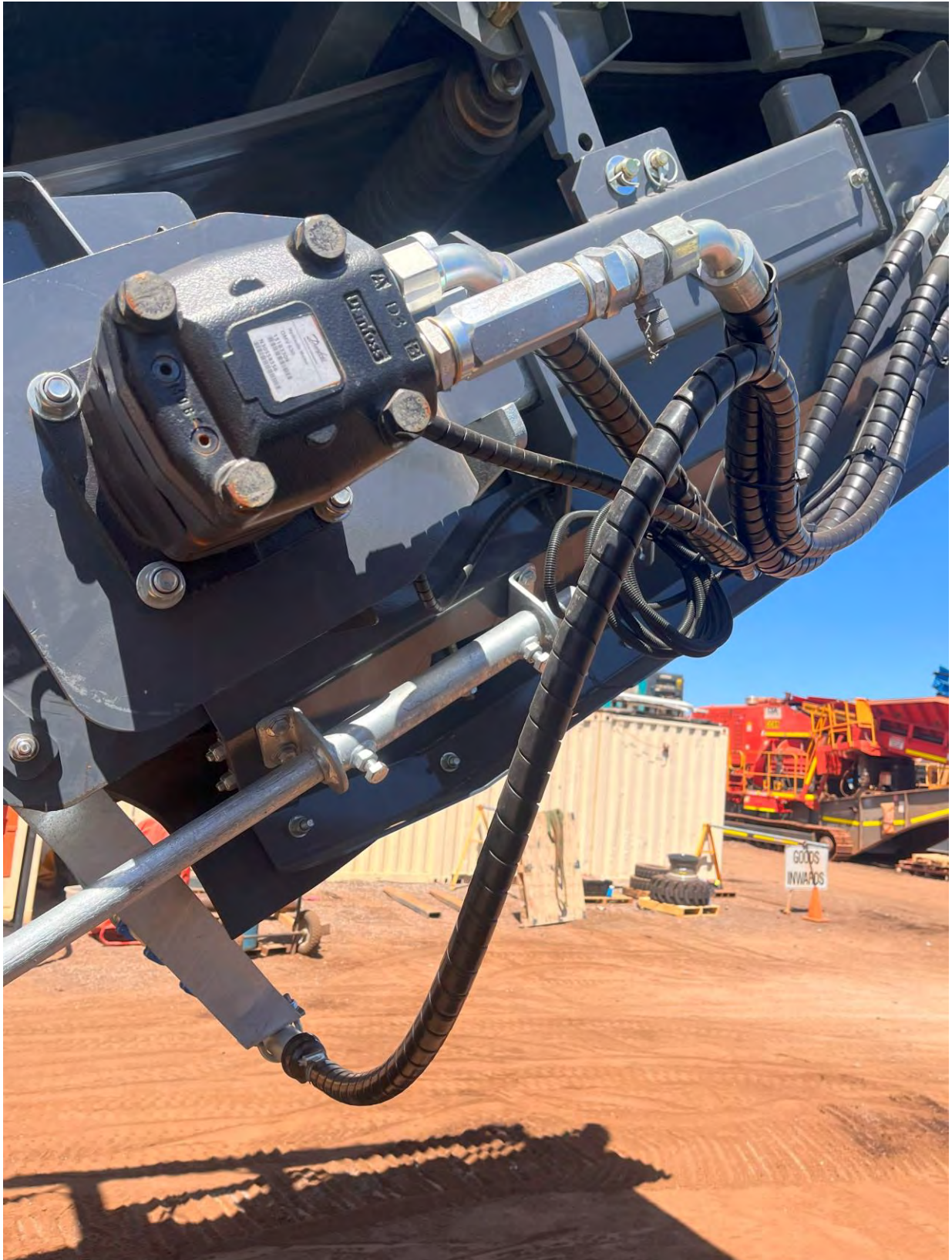
Figure 19 - Striker JM1310 Metso C125 (primary jaw crusher) head drum spray bar in transport mode used on Site C
