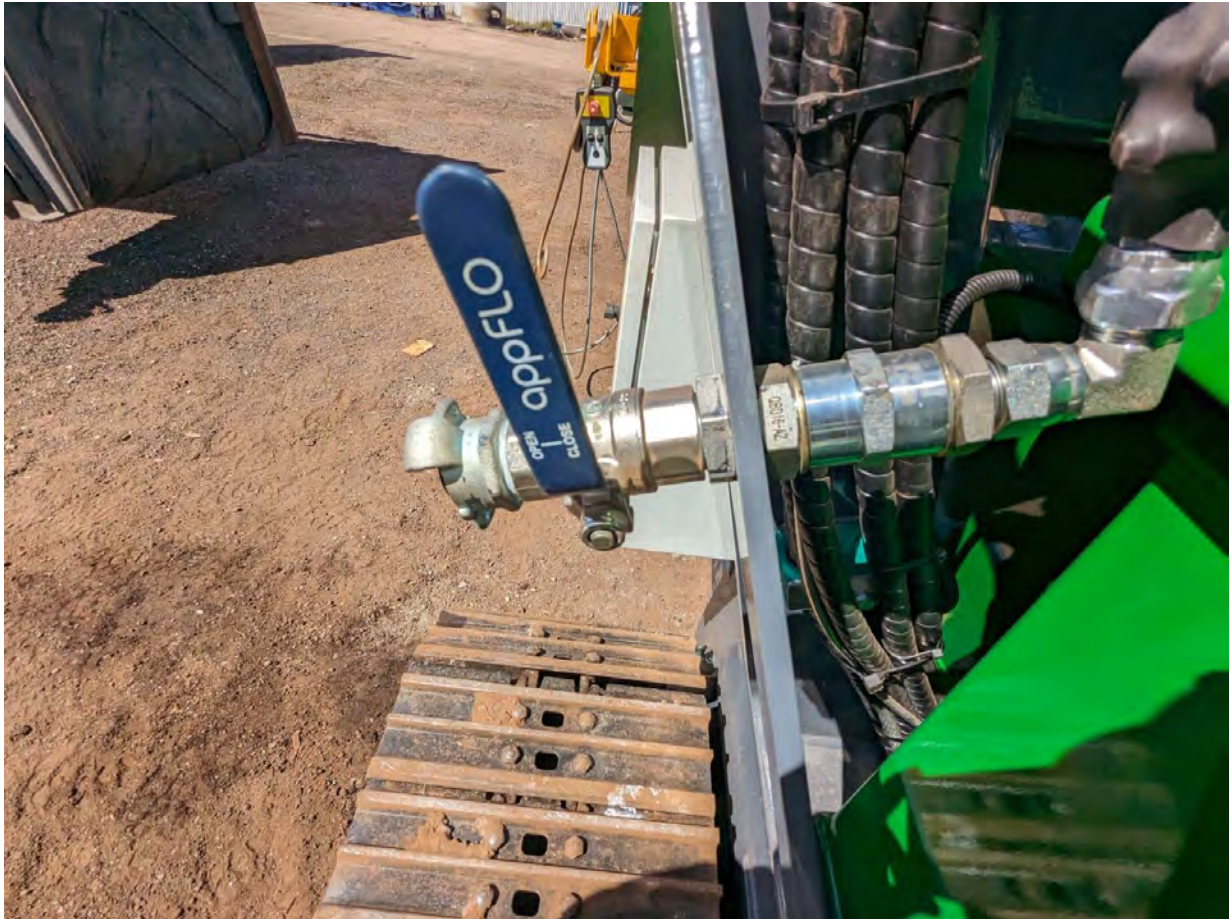
Figure 20 - KES 8048 Stacker Water Manifold inlet used in both Site C and F Site F
