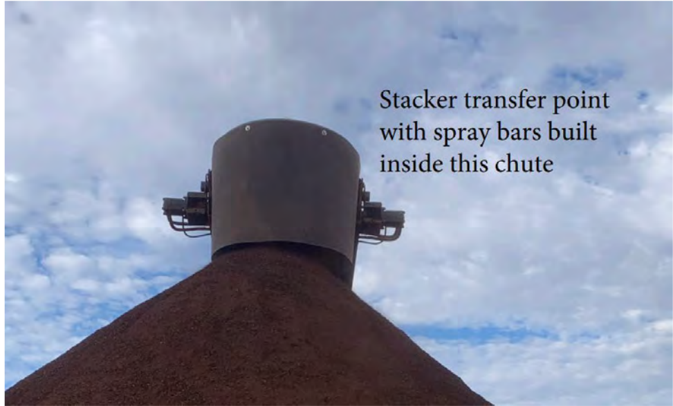
Figure 4-2 Stacker transfer with dust controls
