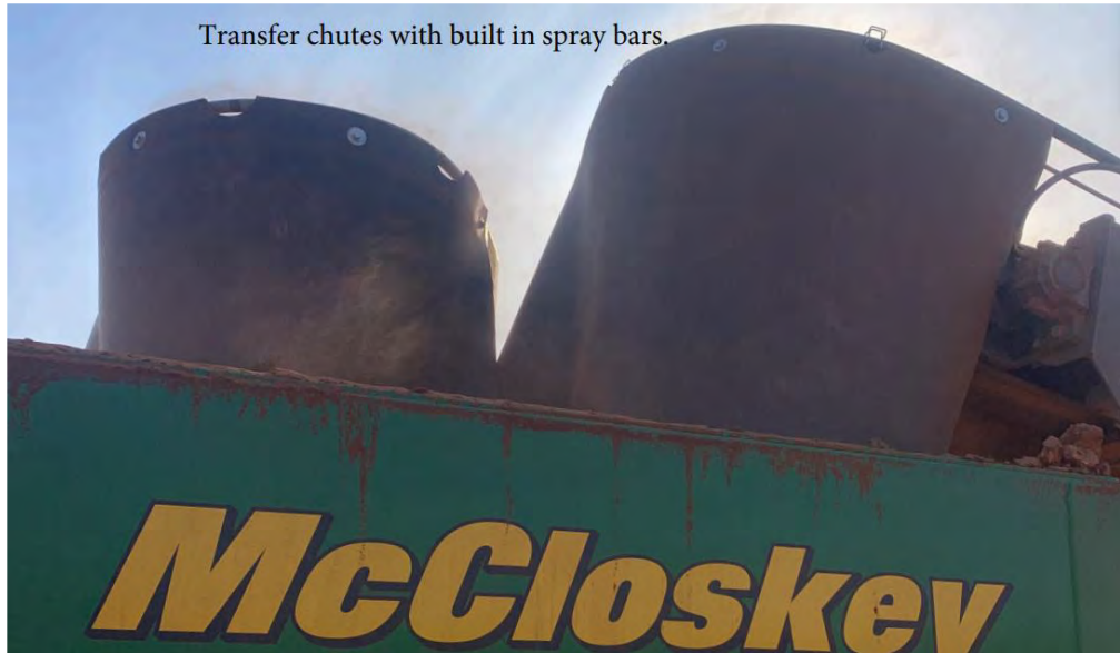
Figure 4-3 Transfer points with dust controls
