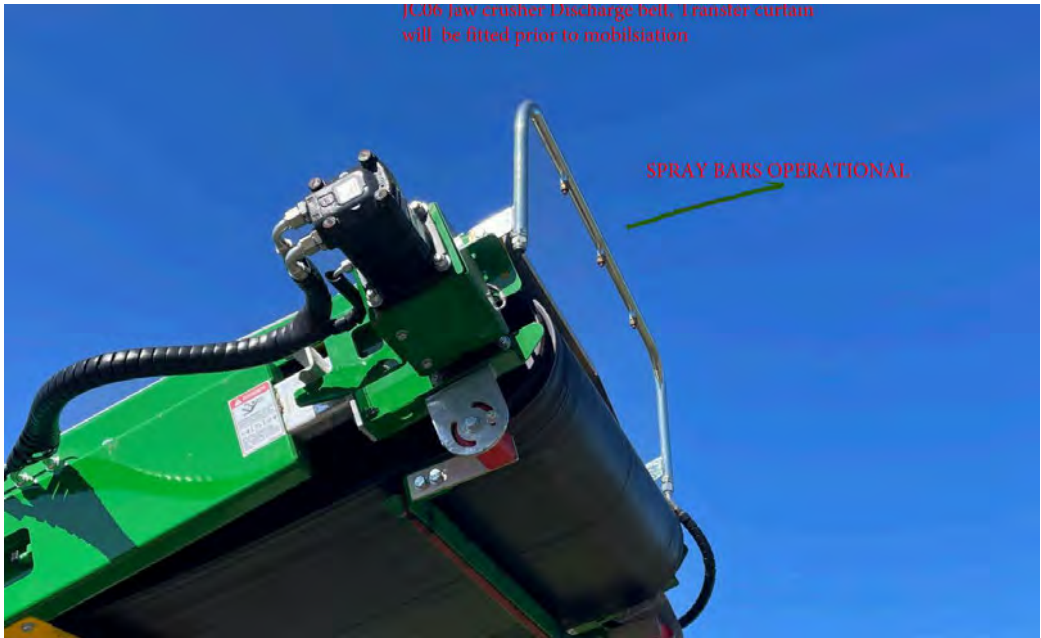
Figure 4-5 Jaw Crusher with spray bars
