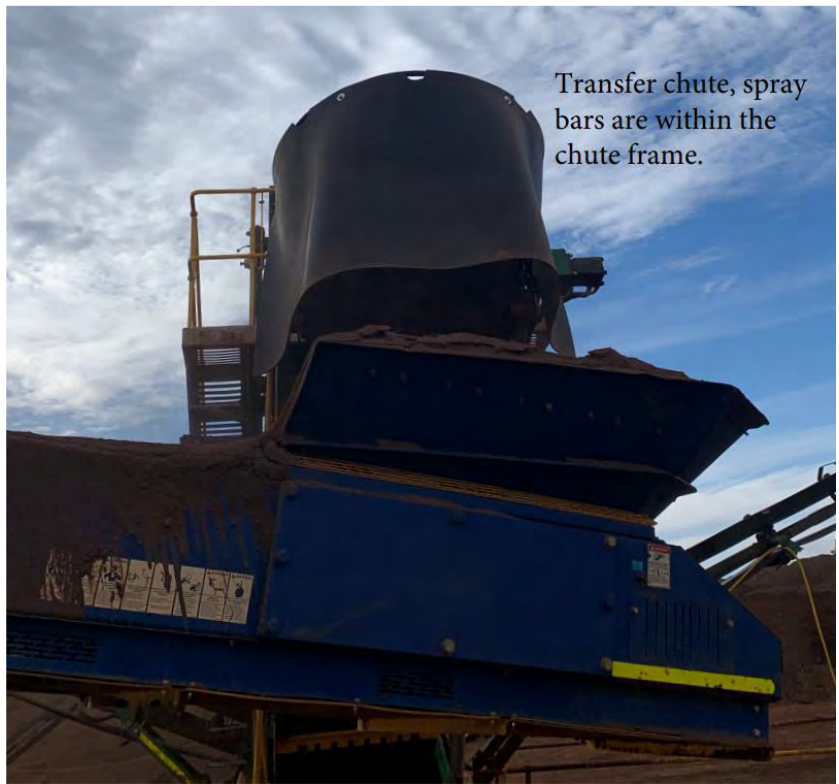
Figure 4-4 Transfer Chute with dust controls
