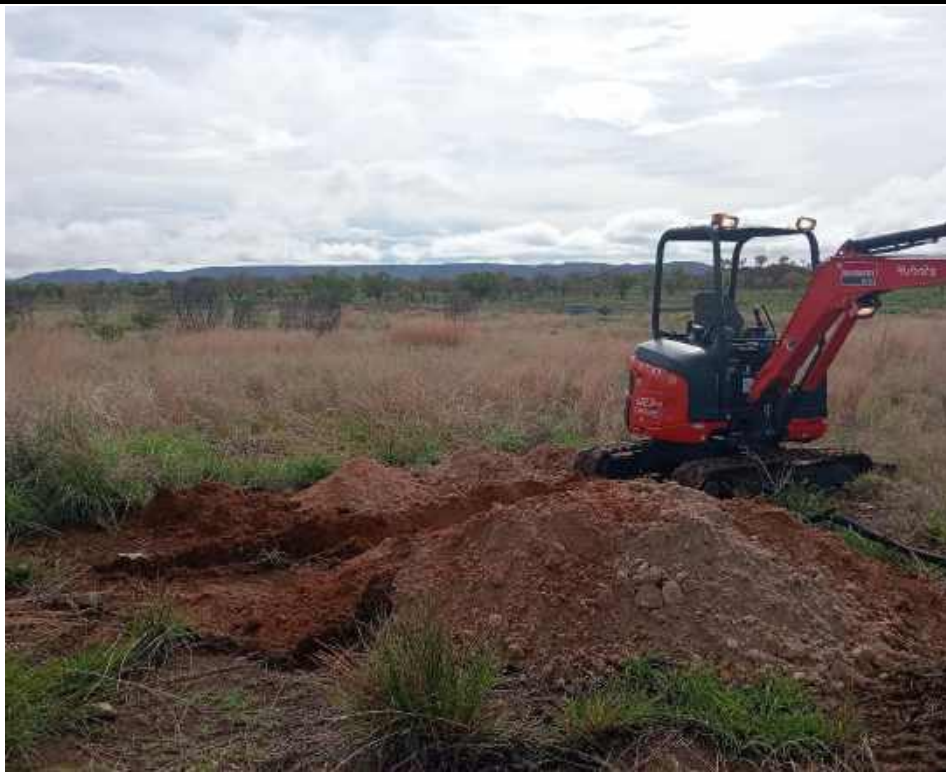
Photo 2. Test Location 01 (TP1), Sub-surface Probing by Using an Excavator
