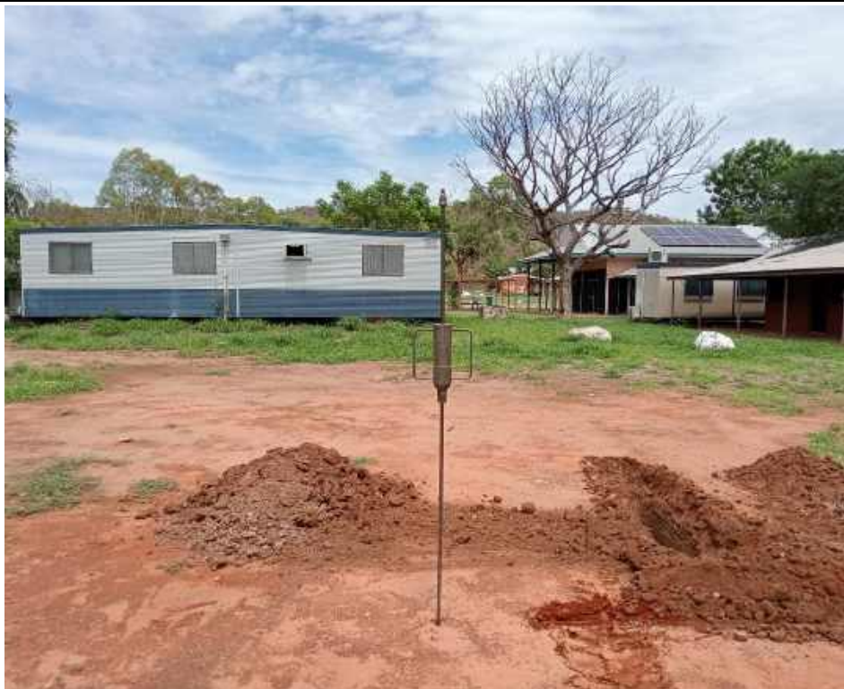
Photo 9. Test Location 22 (DCP22), Testing by Using a Dynamic Cone Penetrometer
