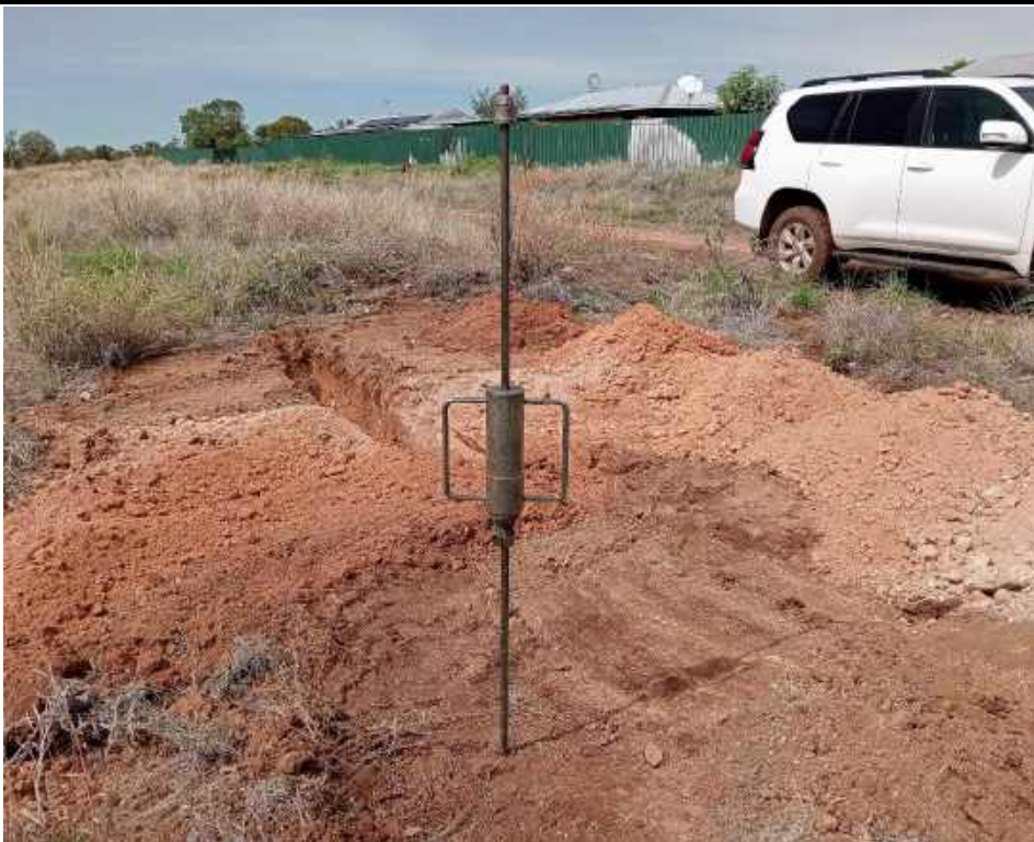
Photo 4. Test Location 09 (DCP9), Testing by using a Dynamic Cone Penetrometer
