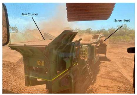
Figure 4: Crusher and screen in action
