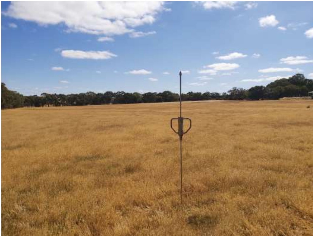
Photo 08: Conducting Dynamic Cone Penetrometer test at DCP2 location
