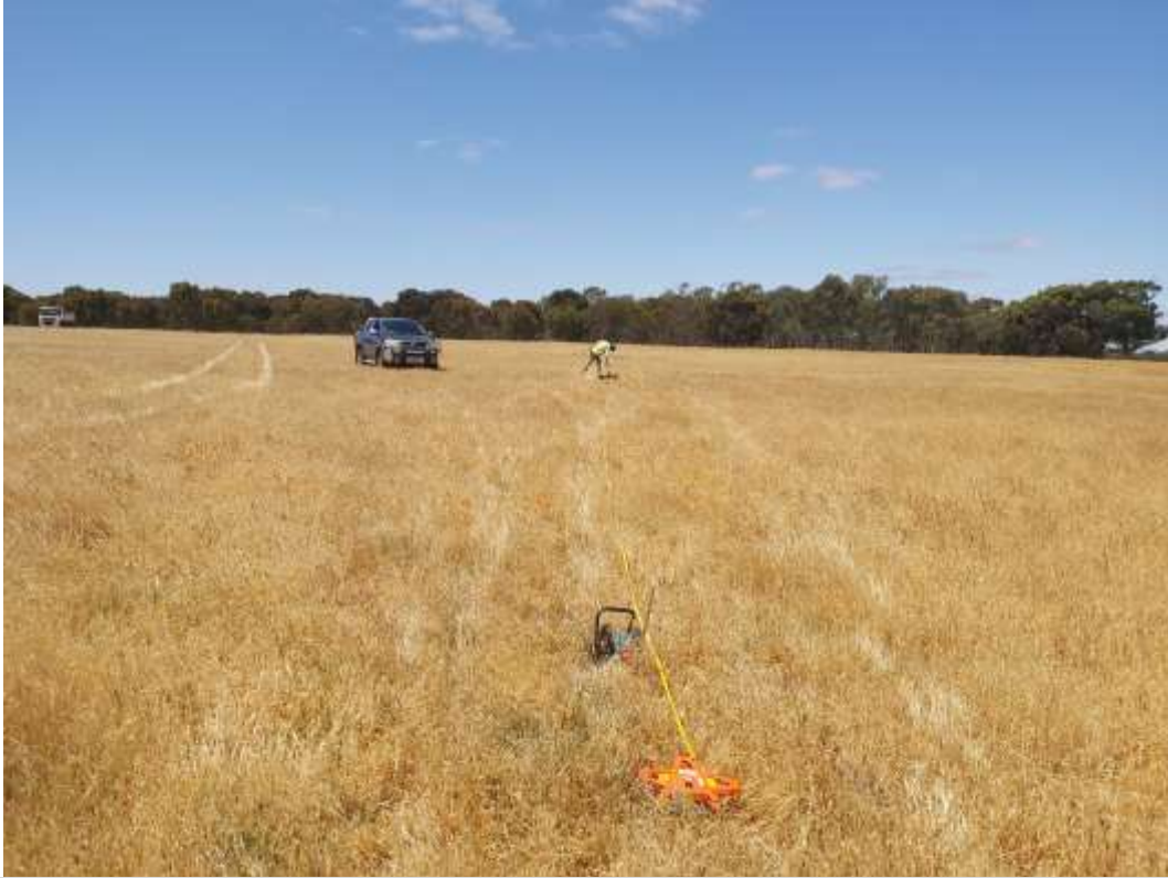
Photo 03: Conducting Electrical/ Soil Resistivity (ER) at ER Test 1 location by Wenner 4 Pole Method
