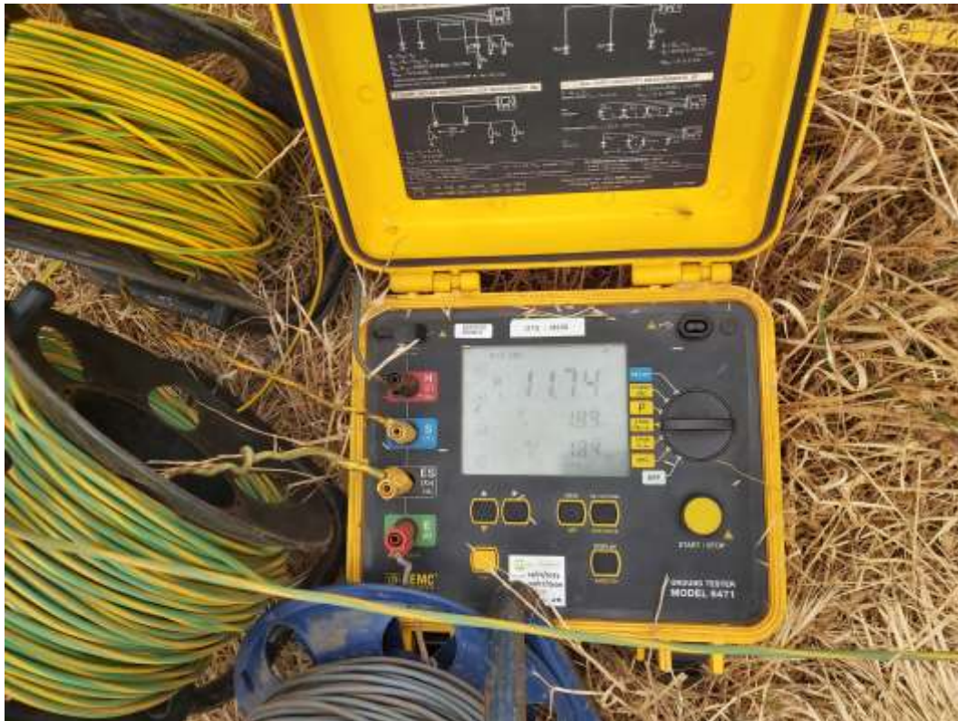
Photo 04. Electrical/ Soil Resistivity (ER) test 1 reading at 8 m interval (N-S) direction
