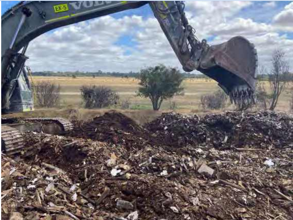
Photograph 10: Wood material found within test pit location WC09 (refer to Figure 4).
