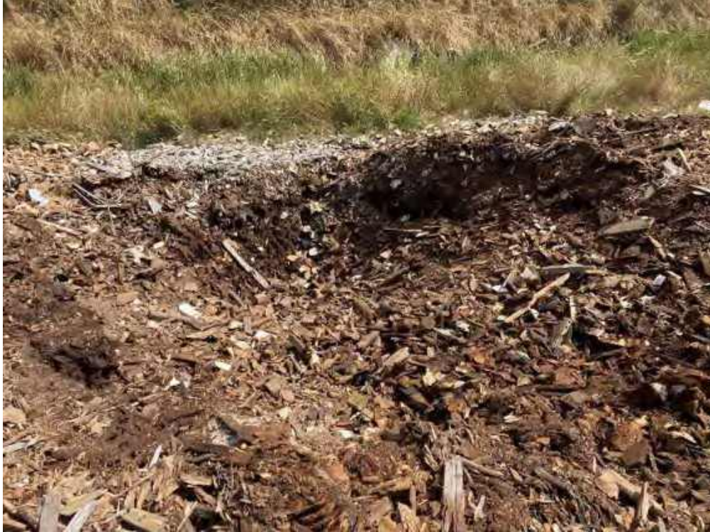
Photograph 7: Wood material found within test pit location WC06 (refer to Figure 4).
