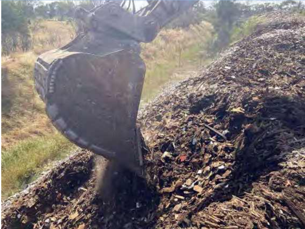
Photograph 9: Wood material found within test pit location WC08 (refer to Figure 4).
