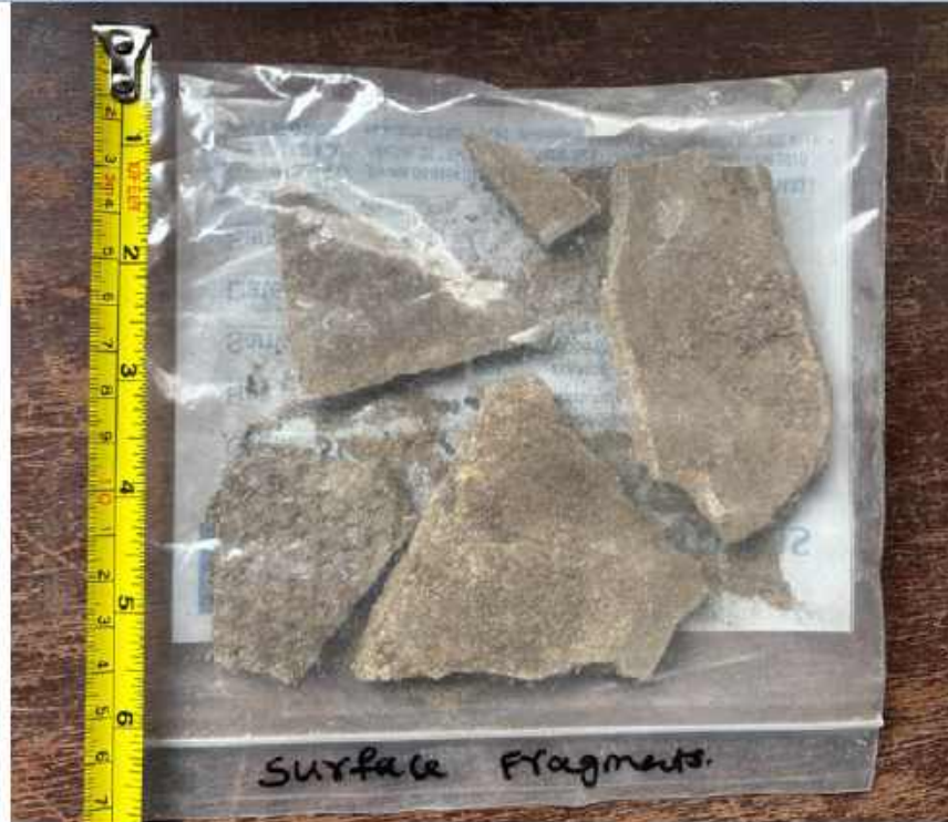
Photograph 3: Surface PACM fragments, identified during stockpile walkover.
