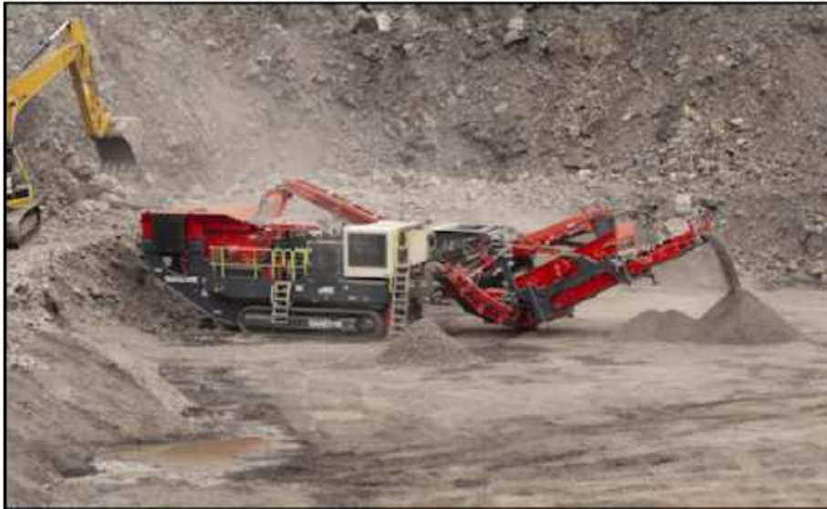
Plate 6-3: Indicative Mobile Crushing and Screening Plant
