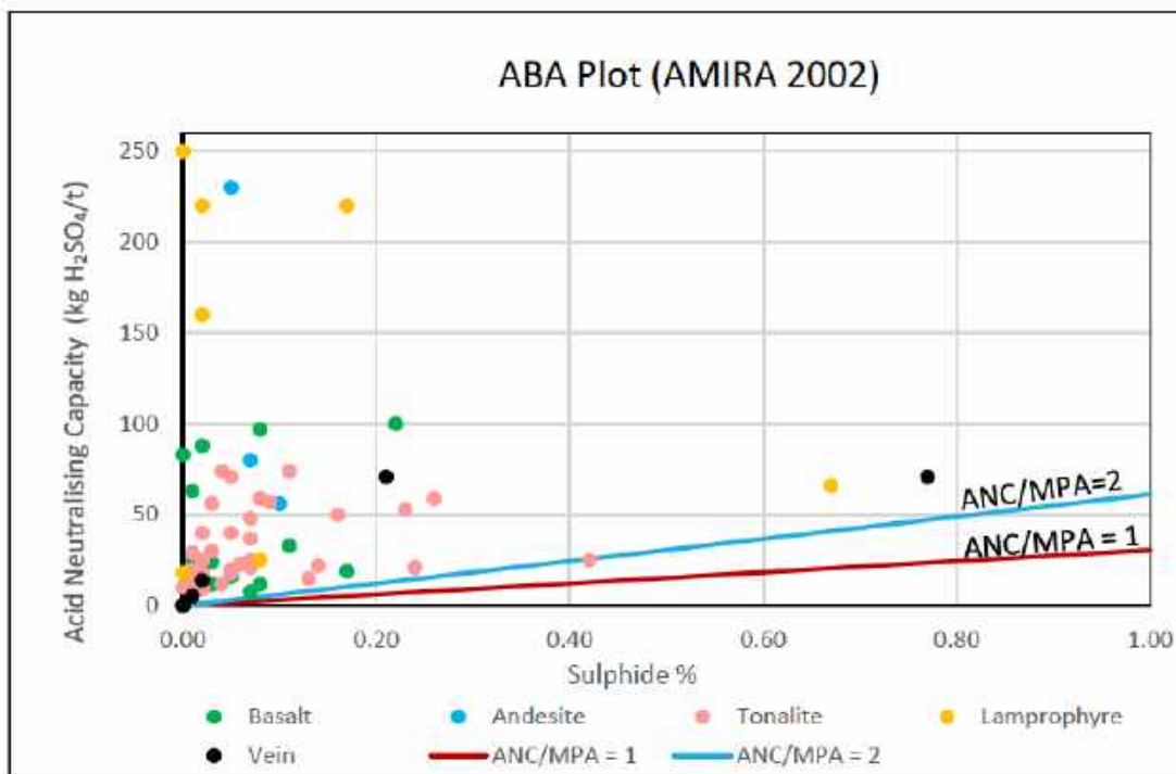
Figure 3-2: ANC to MPA ratio plot of Wonder Waste Samples by Lithology Type
