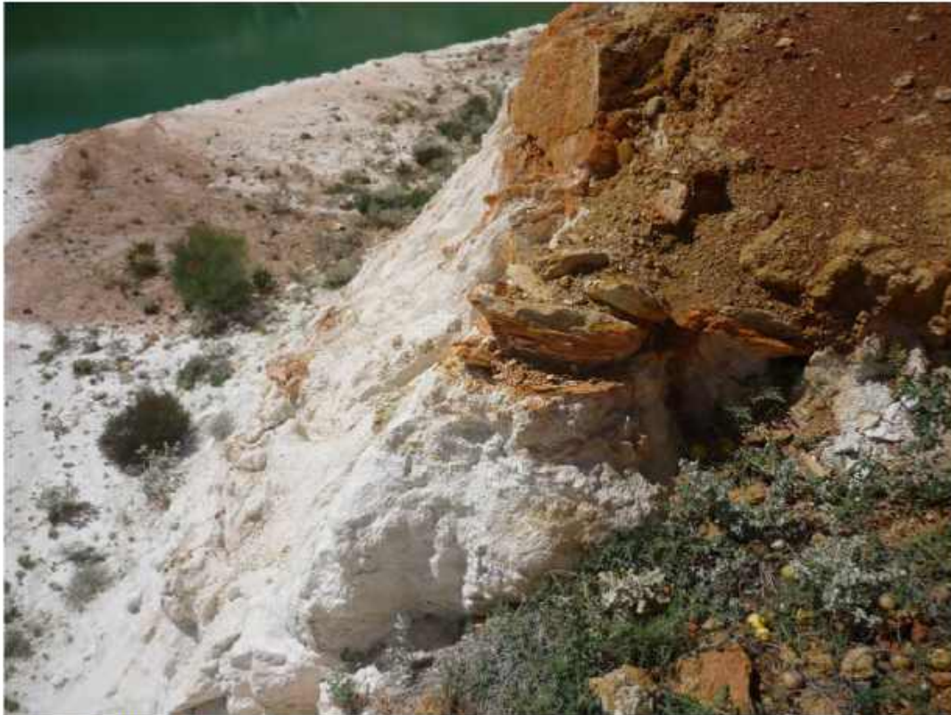
Photograph 5: Laterite zone underlain by pale grey stiff to very stiff clayey silt (2/02/2012)
