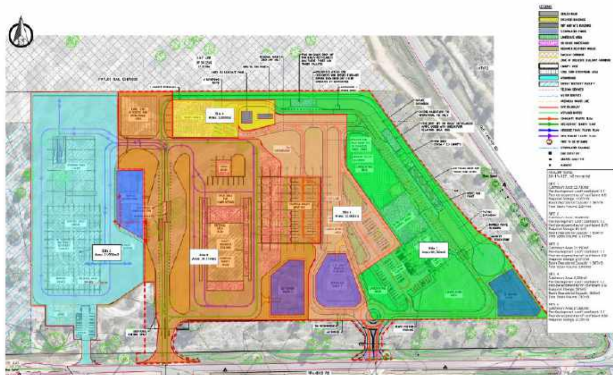
Figure 4-1: General Catchment Areas and Preliminary Basin Locations
