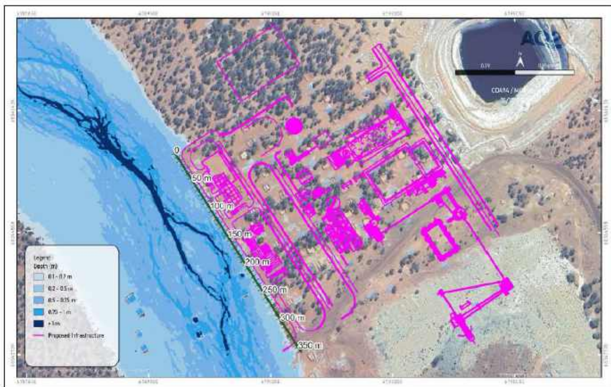
Figure 7: Process Plant - Post-Development Flood Depth (AQ2 2025a)
