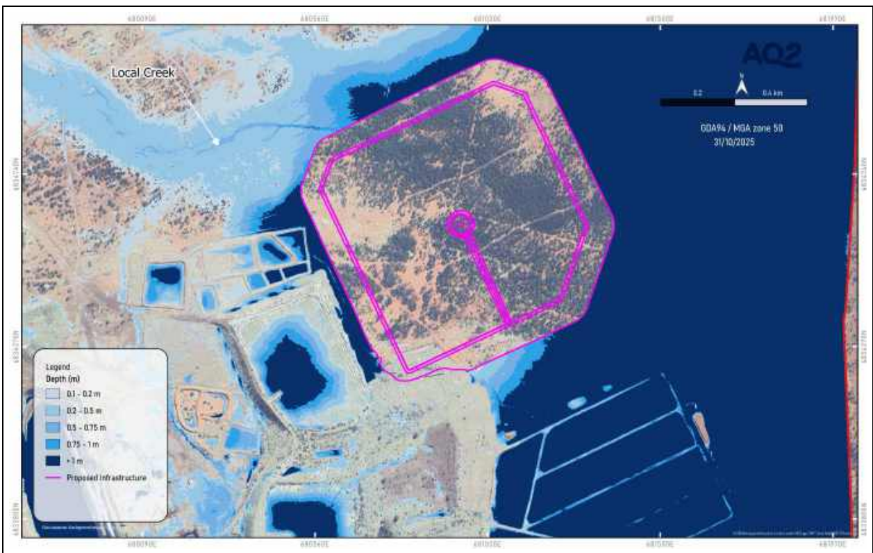
Figure 4.13 TSF Area: PMF Post-Development Flood Depth Map
