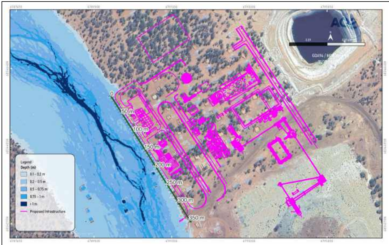
Figure 4.9 Processing Area: 1% AEP Post-Development Flood Depth Map
