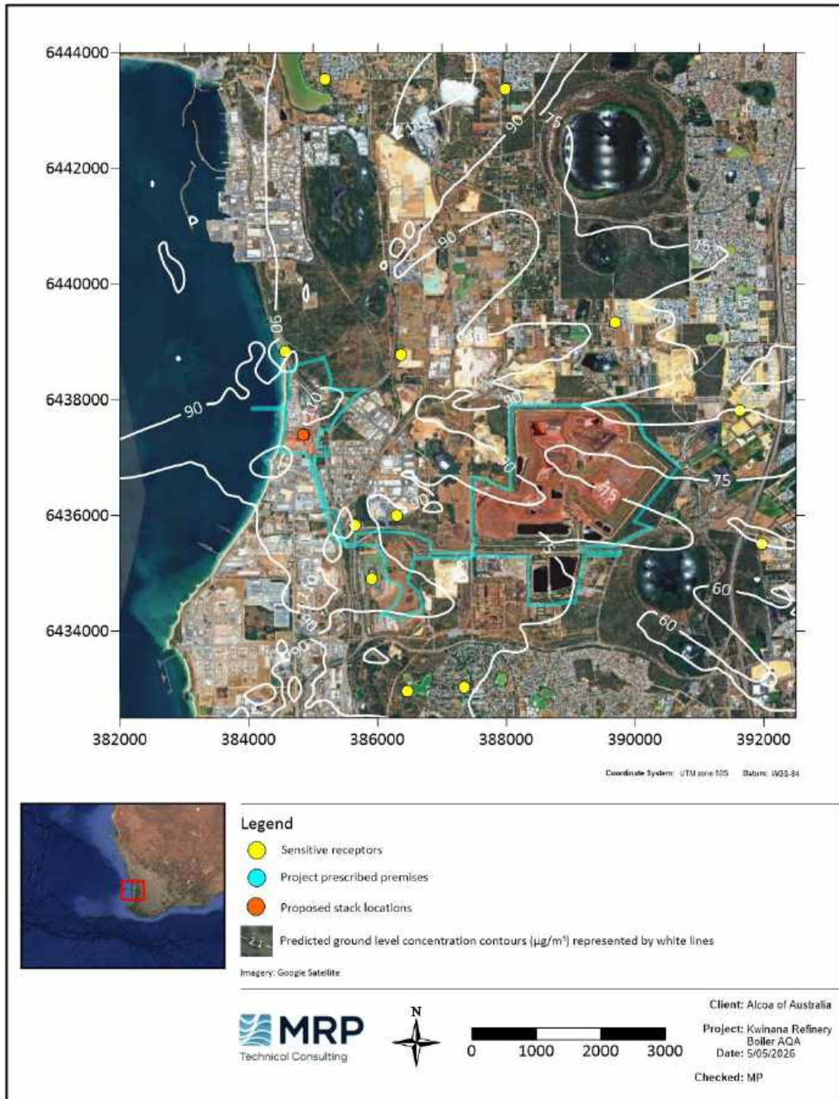
Figure 5-3: Predicted maximum 1-hour average GLCs of NO 2 (Zoomed in) – Scenario 1: Current operations - Cumulative
