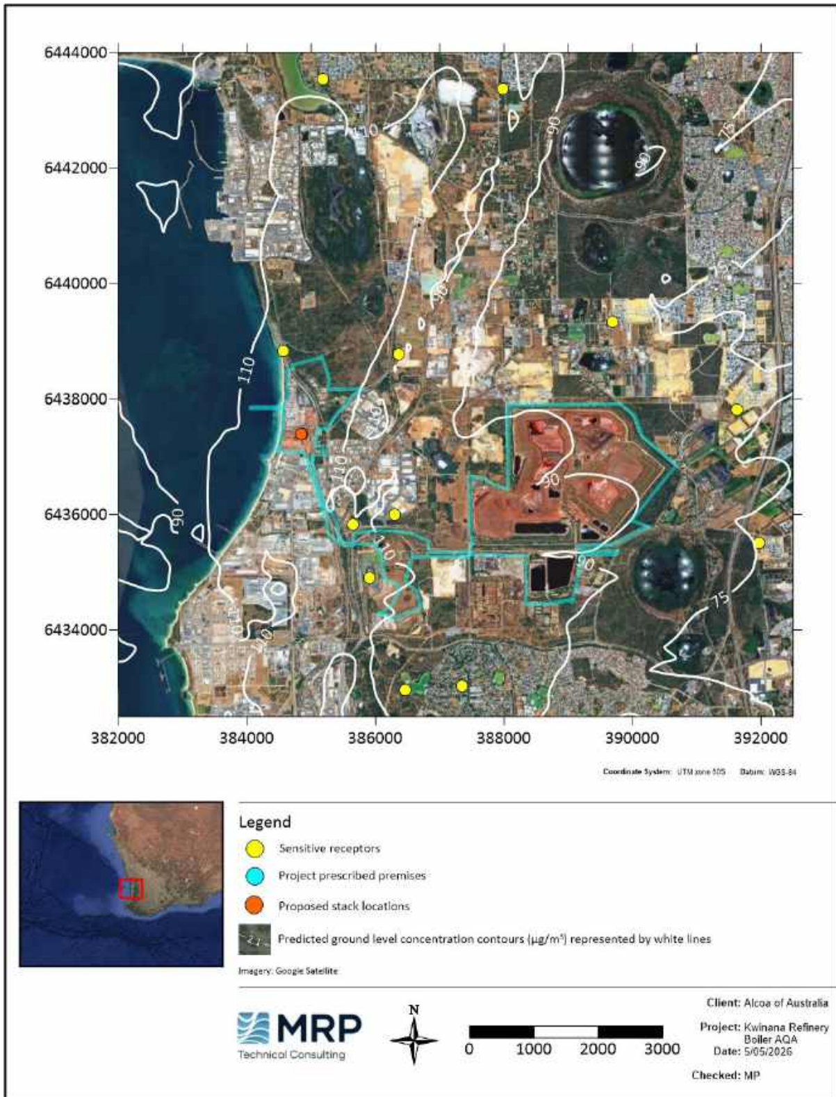
Figure 5-7: Predicted maximum 1-hour average GLCs of NO 2 (Zoomed in) – Scenario 2: Future approved - Cumulative
