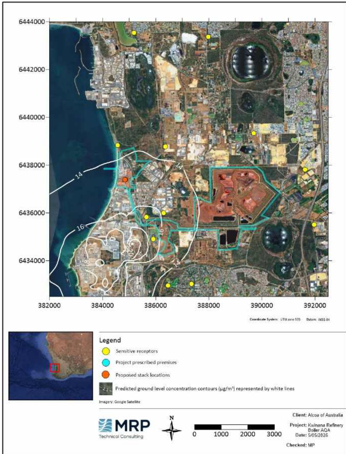
Figure 5-9: Predicted annual average GLCs of \text{NO}_2 (Zoomed in) – Scenario 2: Future approved - Cumulative
