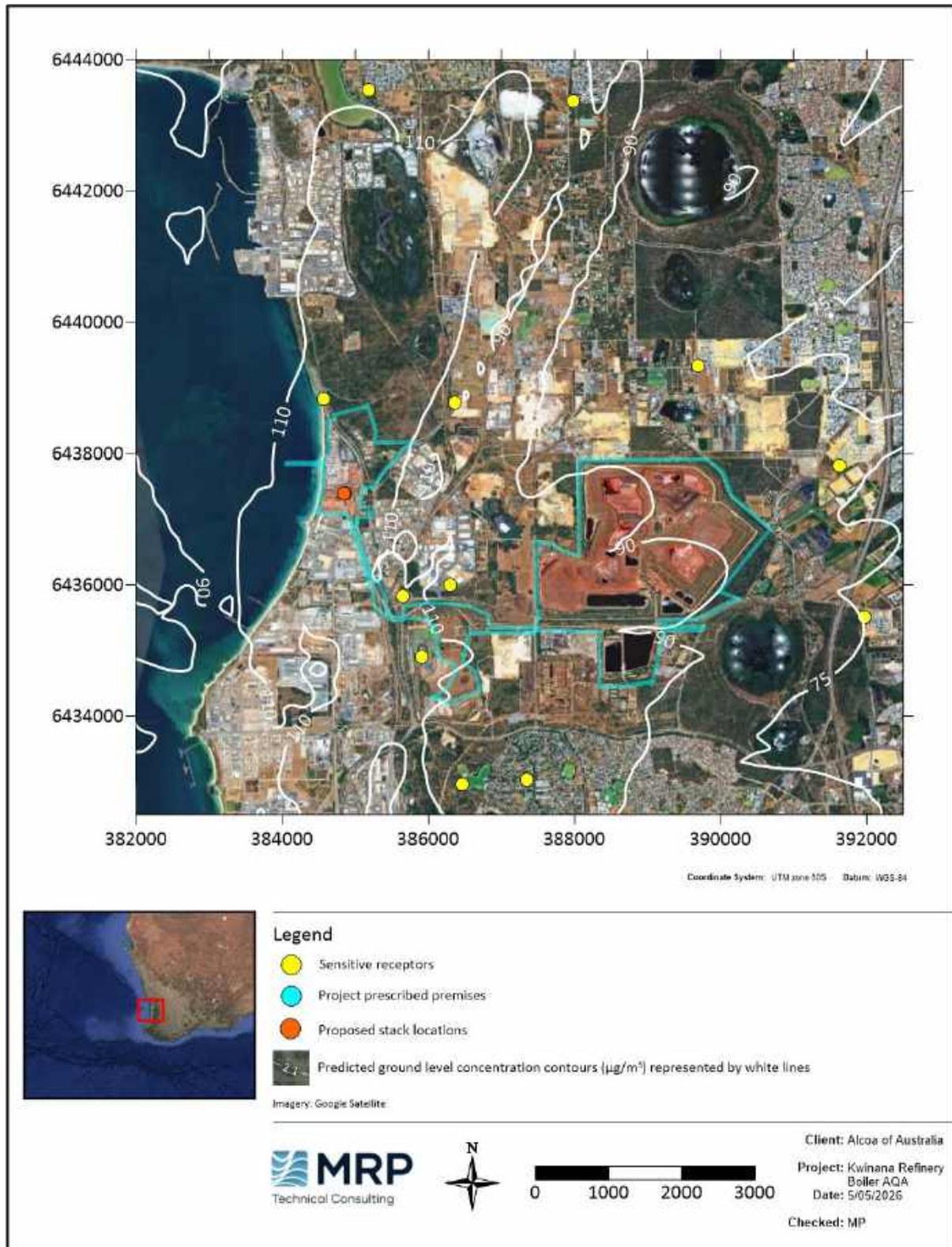
Figure 5-23: Predicted maximum 1-hour average GLCs of NO 2 (Zoomed in) – Scenario 4b – Boiler combination 2 – Cumulative
