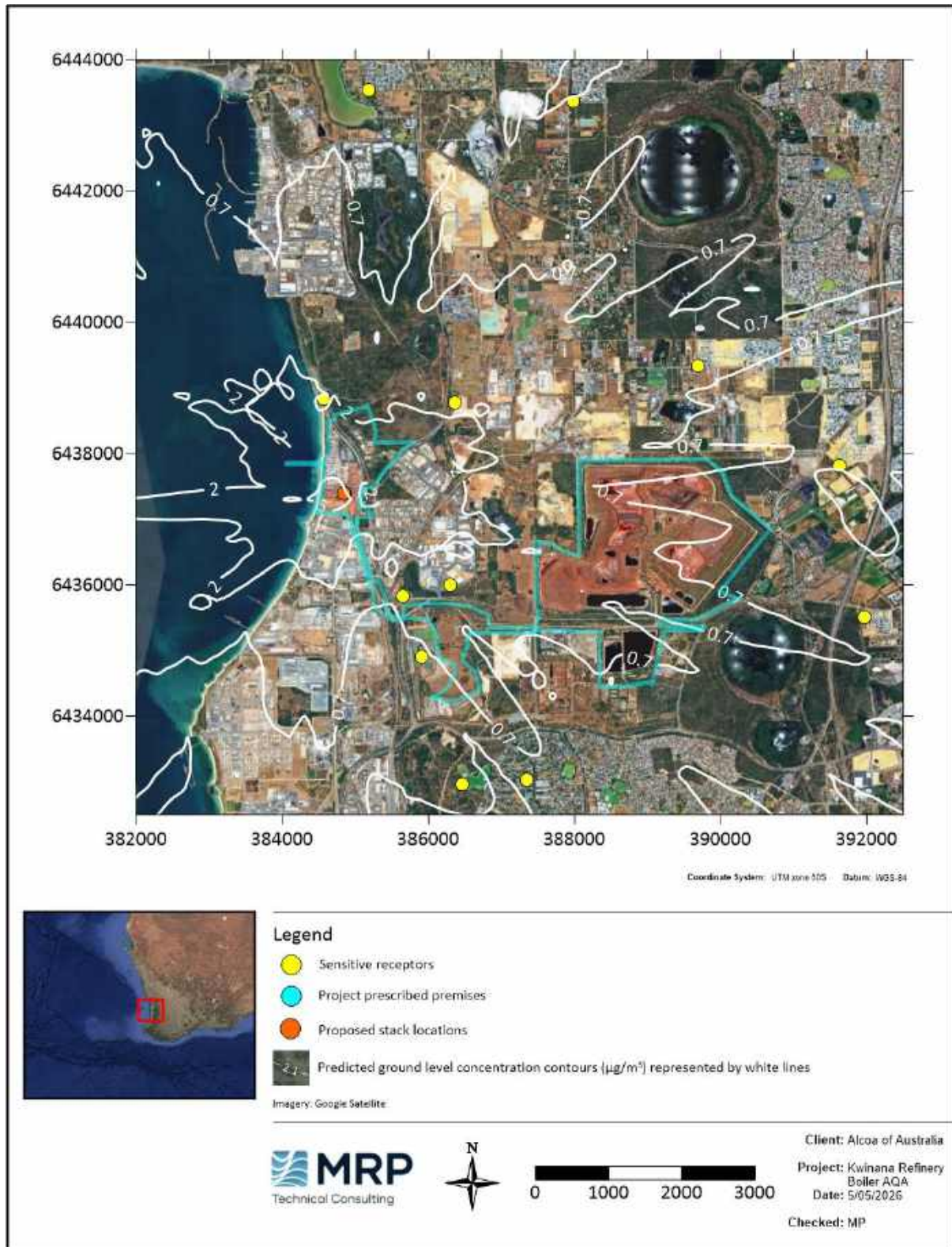
Figure 5-53: Predicted maximum 8-hour average GLCs of CO (Zoomed in) – Scenario 3a – Boiler combination 1 – Isolation
