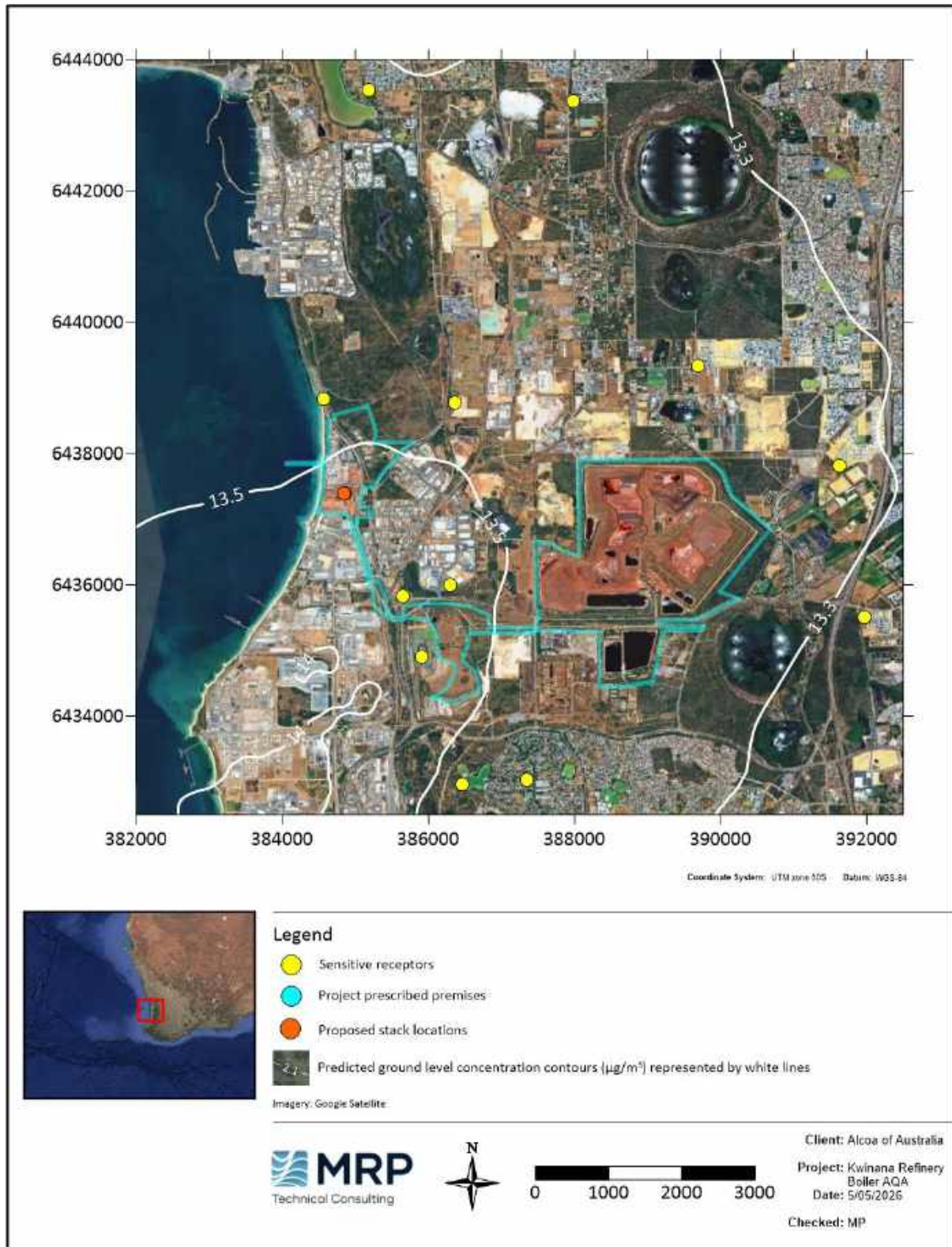
Figure 5-81: Predicted annual average GLCs of PM 10 (Zoomed in) – Scenario 4b – Boiler combination 2 – Cumulative
