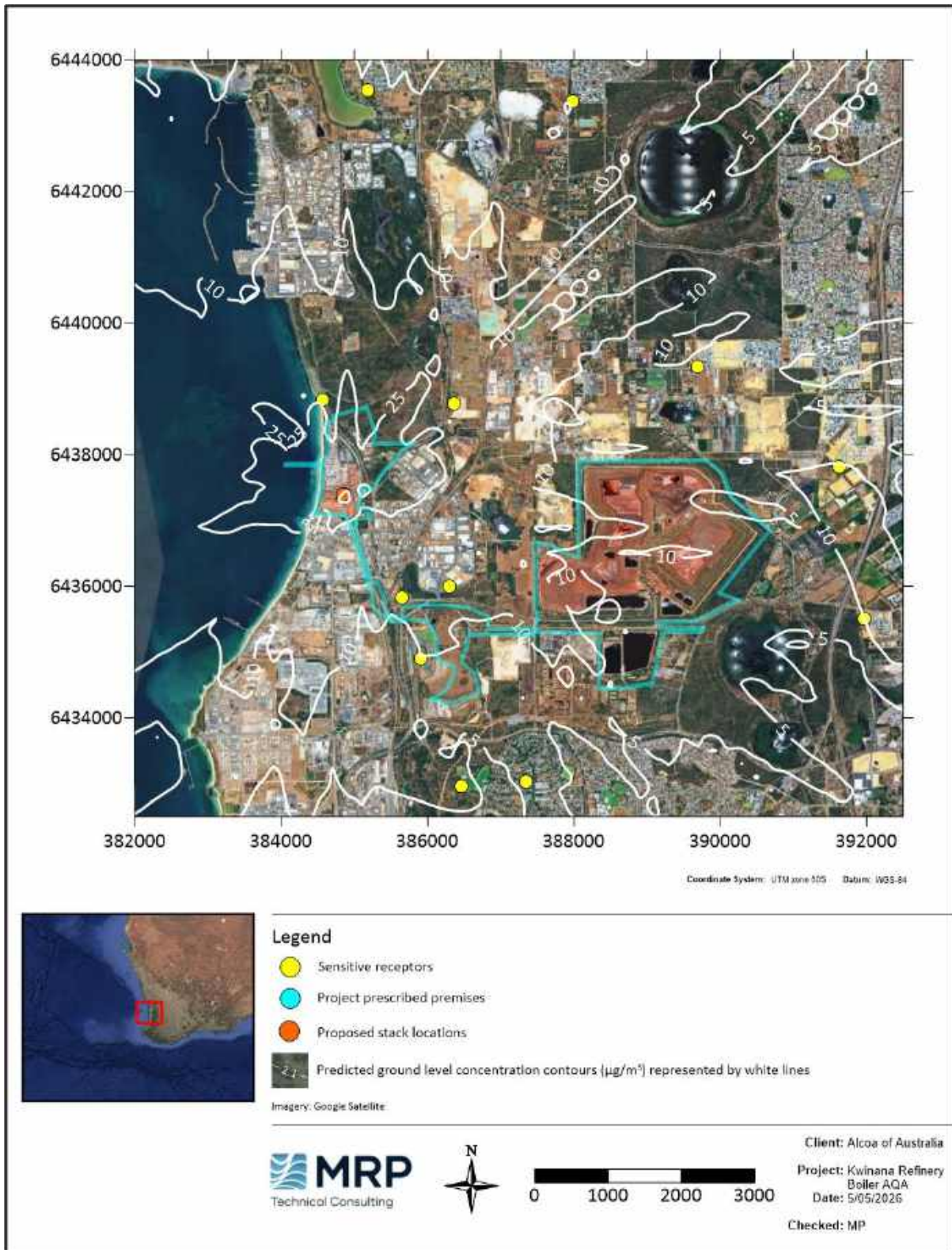
Figure 5-19: Predicted maximum 1-hour average GLCs of NO 2 (Zoomed in) – Scenario 4a – Boiler combination 2 – Isolation
