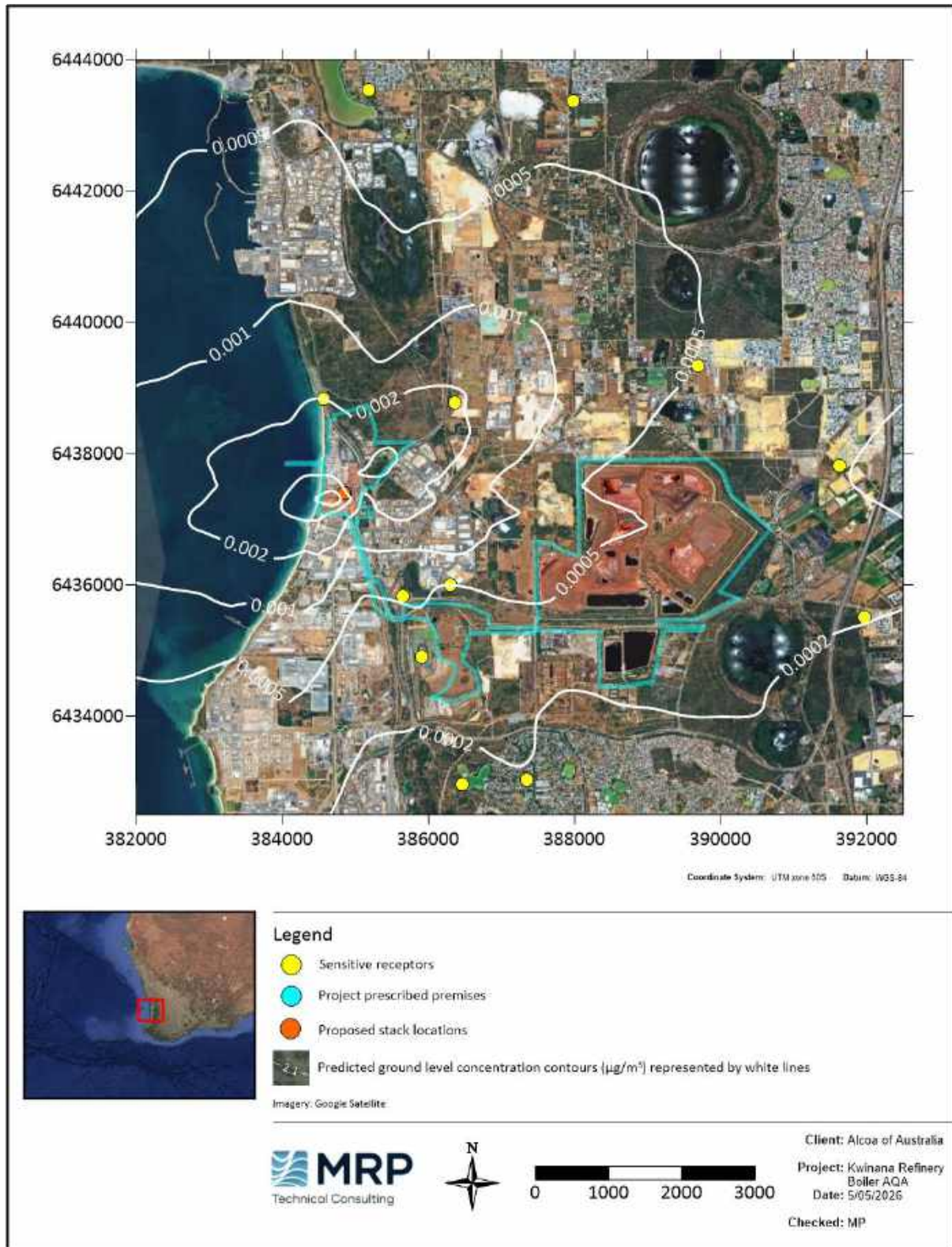
Figure 5-77: Predicted annual average GLCs of PM 10 (Zoomed in) – Scenario 4a – Boiler combination 2 – Isolation
