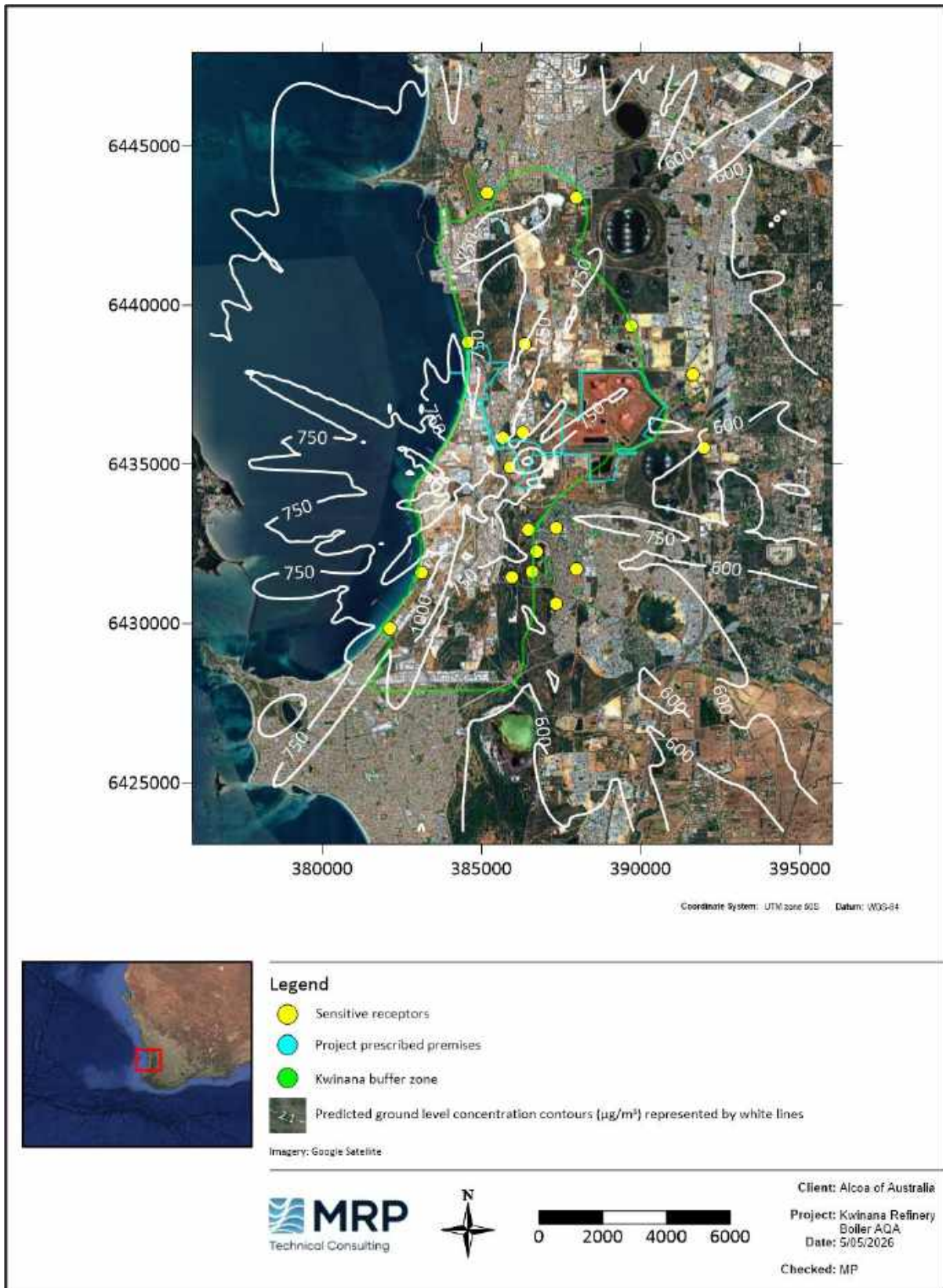
Figure 5-54: Predicted maximum 1-hour average GLCs of CO (Across modelled domain) – Scenario 3b – Boiler combination 1 – Cumulative
