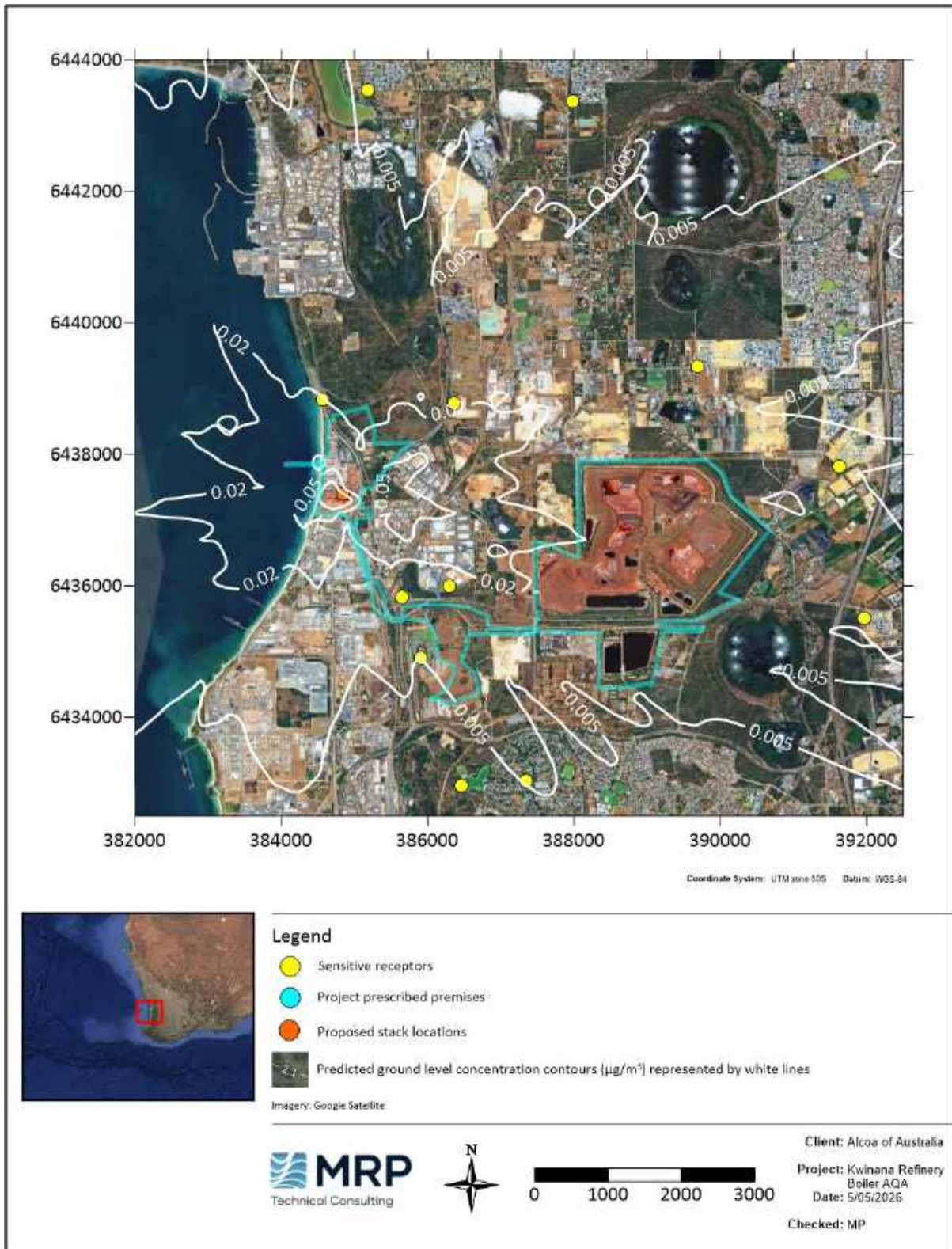
Figure 5-91: Predicted maximum 24-hour average GLCs of \text{PM}_{2.5} (Zoomed in) – Scenario 4a – Boiler combination 2 – Isolation
