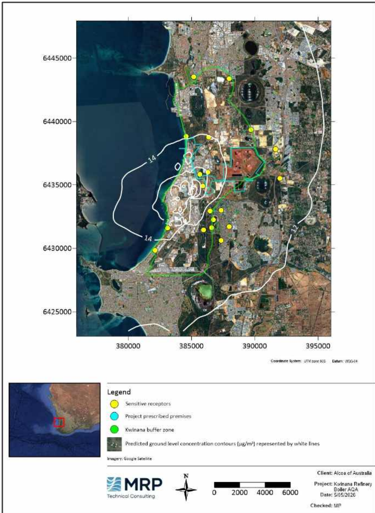
Figure 5-24: Predicted annual average GLCs of \text{NO}_2 (Across modelled domain) – Scenario 4b – Boiler combination 2 – Cumulative
