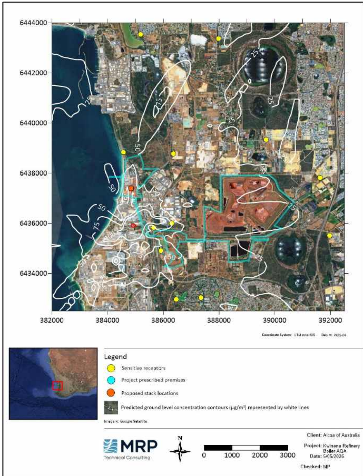
Figure 5-33: Predicted maximum 1-hour average GLCs of SO 2 (Zoomed in) – Scenario 3b – Boiler combination 1 – Cumulative
