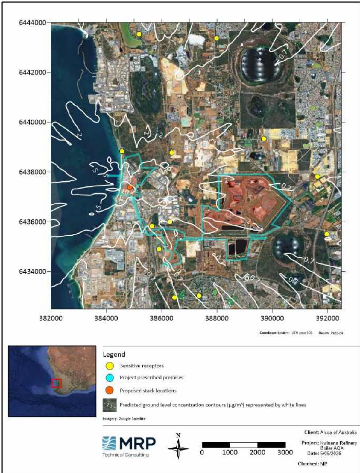
Figure 5-61: Predicted maximum 8-hour average GLCs of CO (Zoomed in) – Scenario 4a – Boiler combination 2 – Isolation
