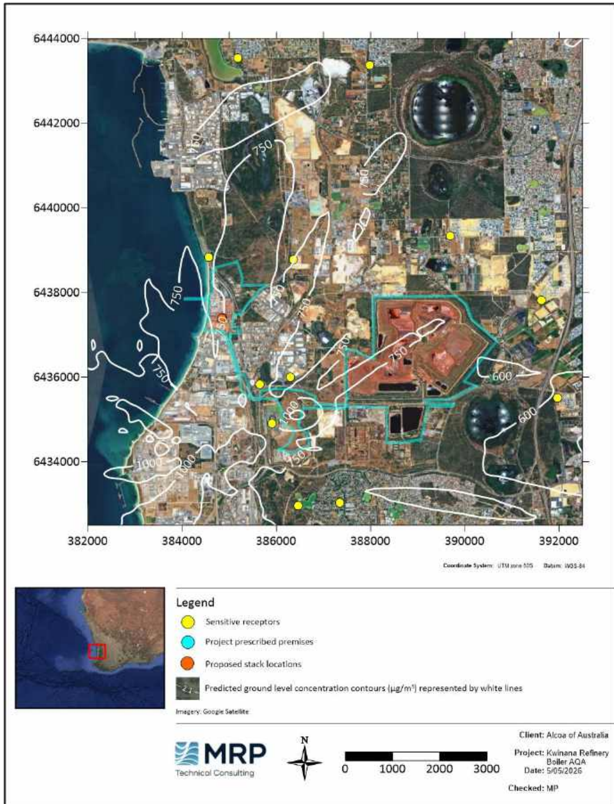
Figure 5-63: Predicted maximum 1-hour average GLCs of CO (Zoomed in) – Scenario 4b – Boiler combination 2 – Cumulative
