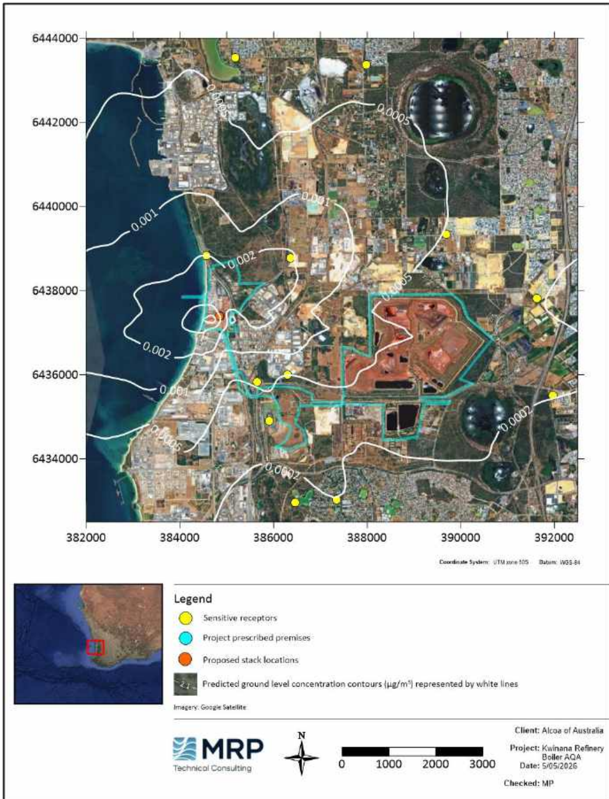
Figure 5-85: Predicted annual average GLCs of PM 2.5 (Zoomed in) – Scenario 3a – Boiler combination 1 – Isolation
