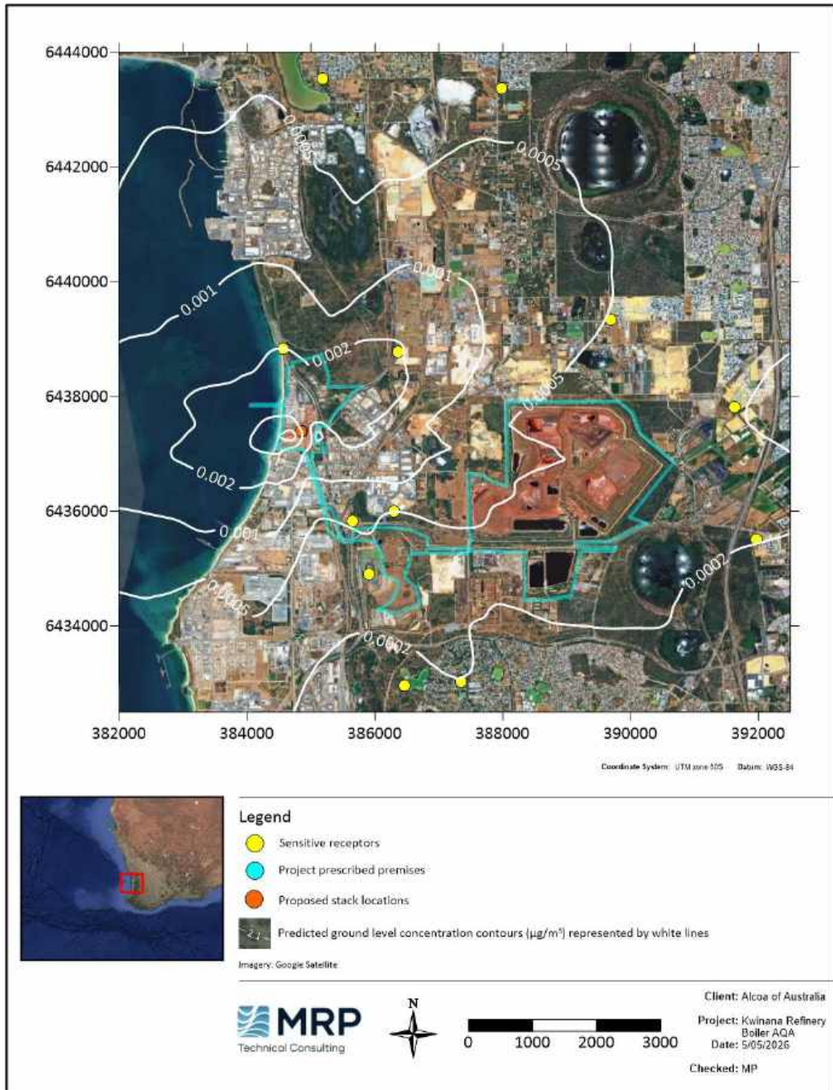
Figure 5-69: Predicted annual average GLCs of PM 10 (Zoomed in) – Scenario 3a – Boiler combination 1 – Isolation
