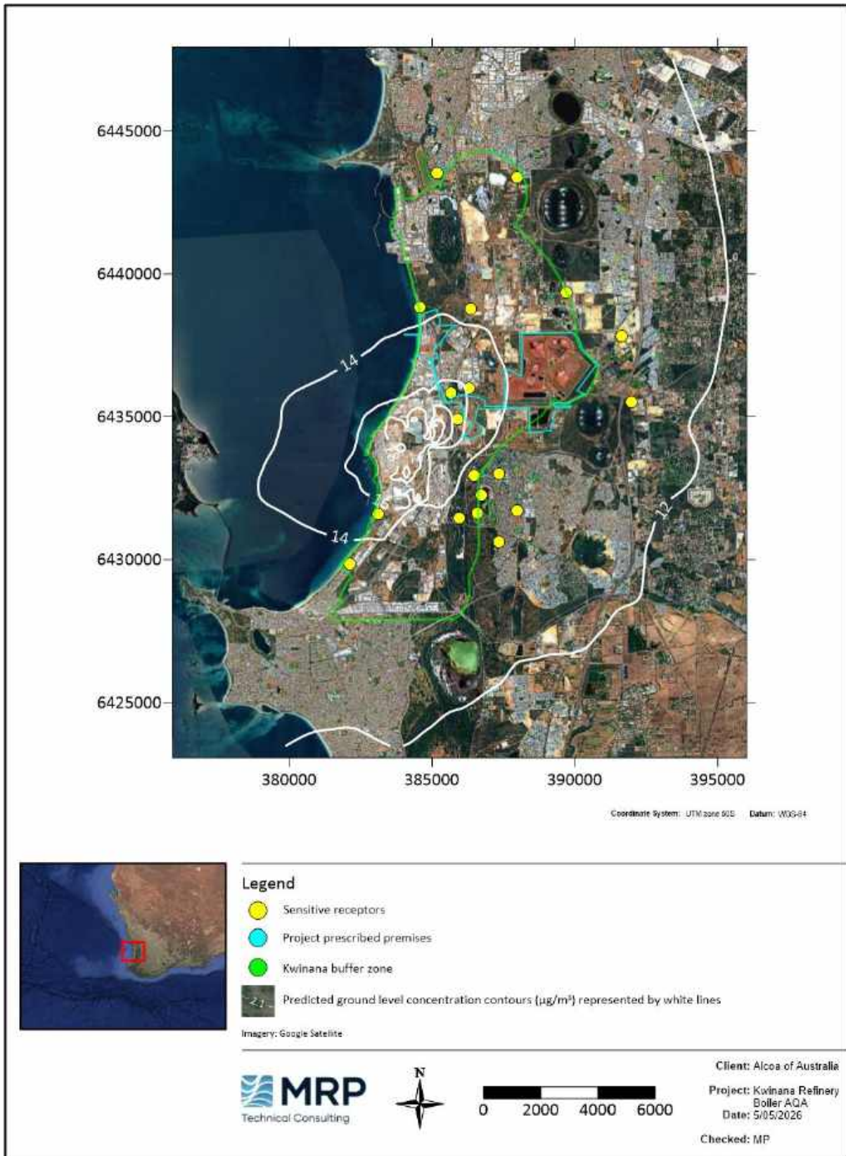
Figure 5-8: Predicted annual average GLCs of \text{NO}_2 (Across modelled domain) – Scenario 2: Future approved - Cumulative
