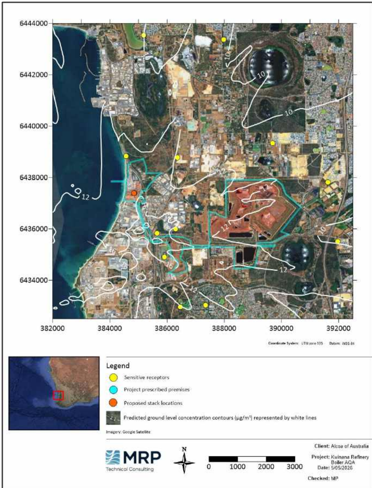
Figure 5-35: Predicted maximum 24-hour average GLCs of SO 2 (Zoomed in) – Scenario 3b – Boiler combination 1 – Cumulative
