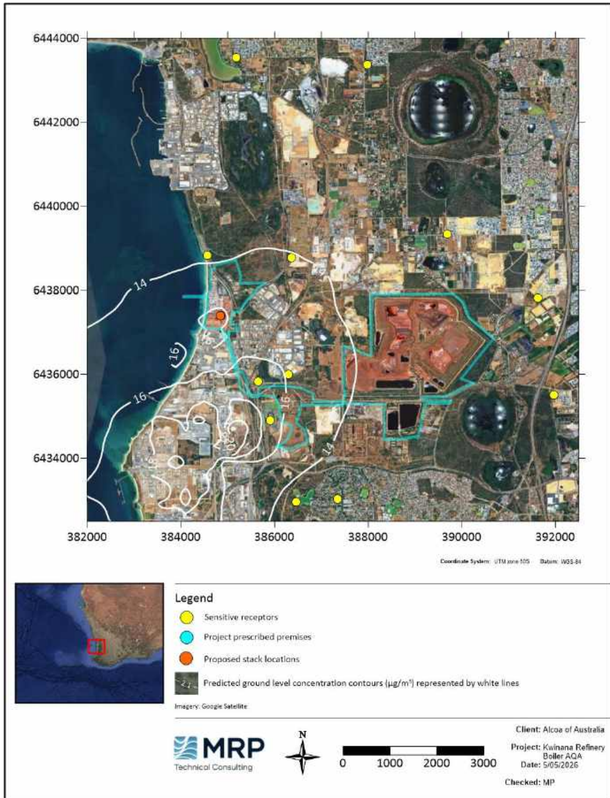
Figure 5-25: Predicted annual average GLCs of NO 2 (Zoomed in) – Scenario 4b – Boiler combination 2 – Cumulative
