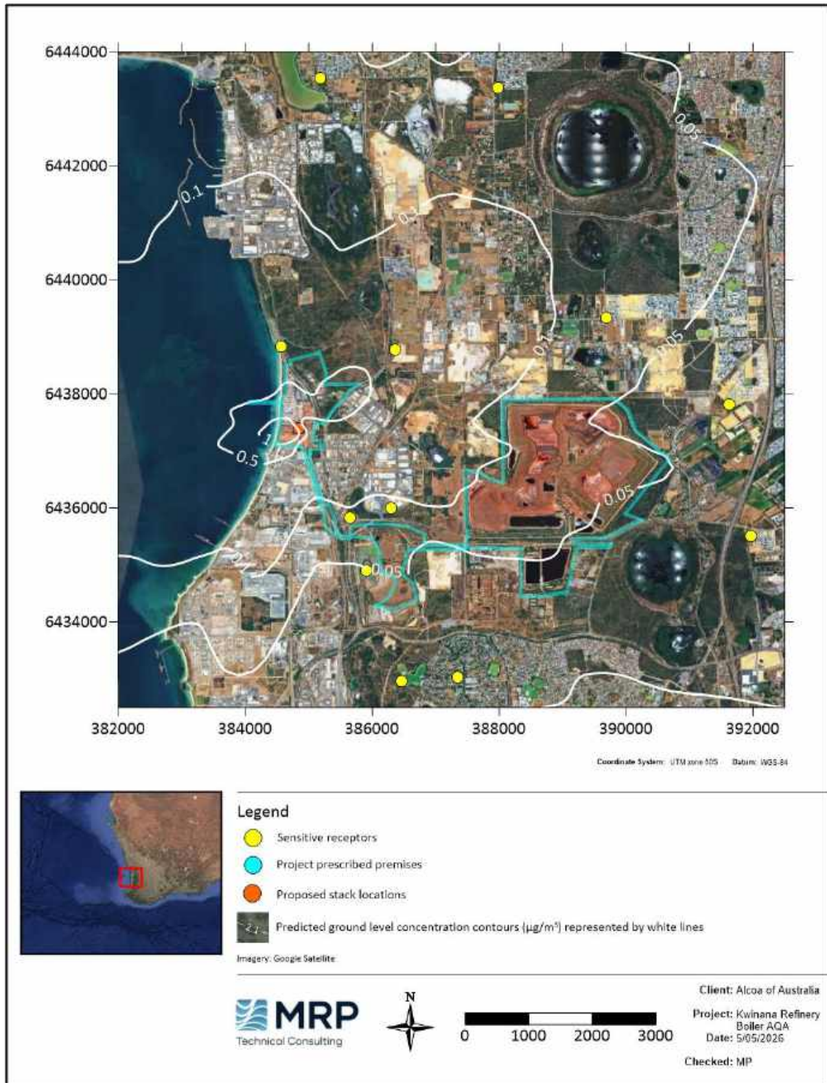
Figure 5-21: Predicted annual average GLCs of NO 2 (Zoomed in) – Scenario 4a – Boiler combination 2 – Isolation
