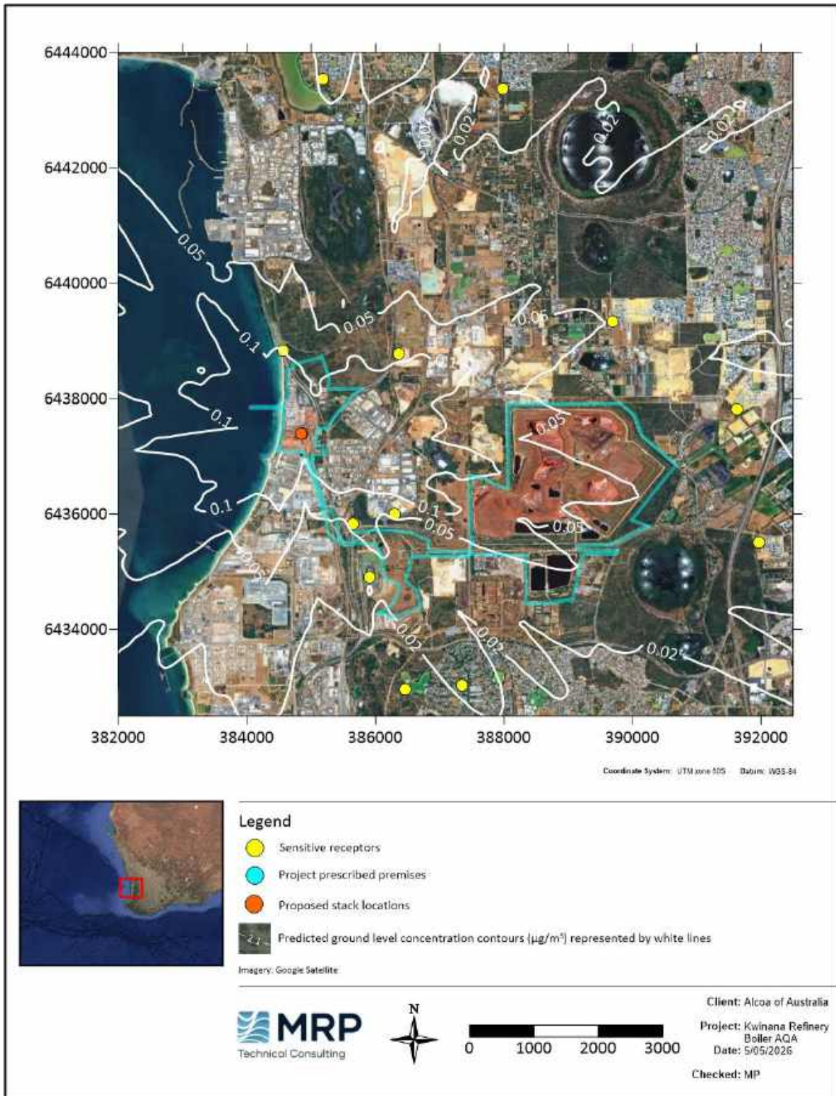
Figure 5-41 Predicted maximum 24-hour average GLCs of SO 2 (Zoomed in) – Scenario 4a – Boiler combination 2 – Isolation
