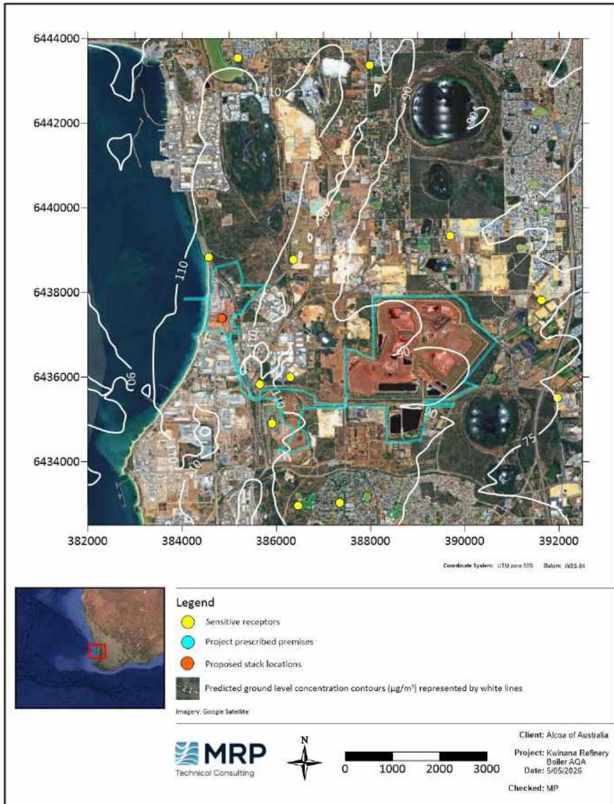
Figure 5-15: Predicted maximum 1-hour average GLCs of NO 2 (Zoomed in) – Scenario 3b – Boiler combination 1 – Cumulative
