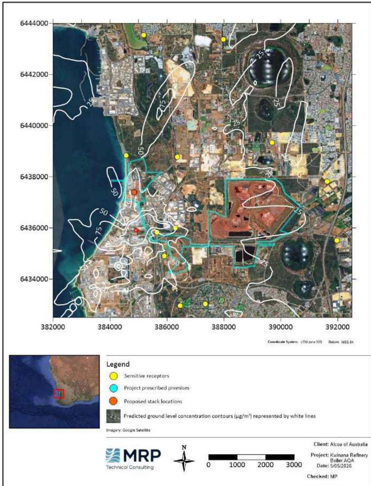
Figure 5-45: Predicted maximum 1-hour average GLCs of SO 2 (Zoomed in) – Scenario 4b – Boiler combination 2 – Cumulative
