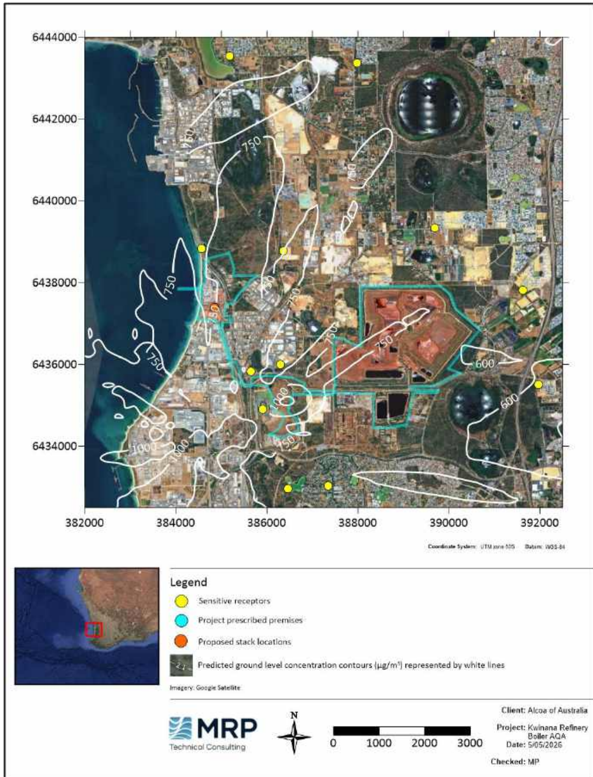
Figure 5-55: Predicted maximum 1-hour average GLCs of CO (Zoomed in) – Scenario 3b – Boiler combination 1 – Cumulative
