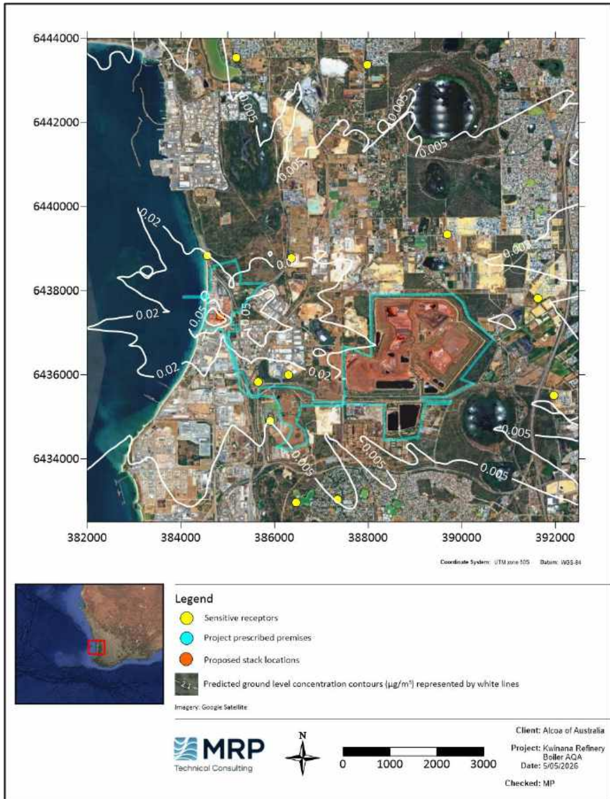
Figure 5-75: Predicted maximum 24-hour average GLCs of PM 10 (Zoomed in) – Scenario 4a – Boiler combination 2 – Isolation
