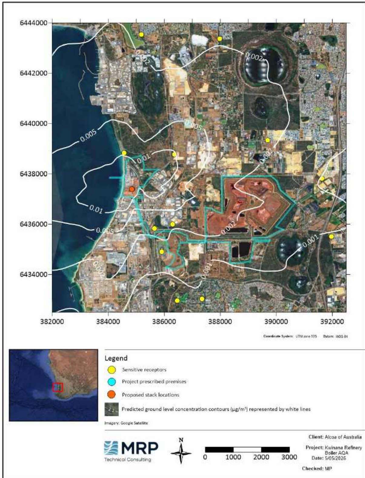
Figure 5-43: Predicted annual average GLCs of SO 2 (Zoomed in) – Scenario 4a – Boiler combination 2 – Isolation
