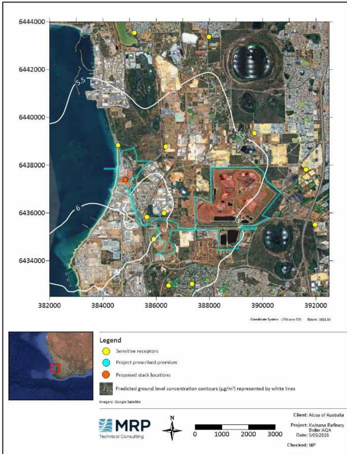
Figure 5-37: Predicted annual average GLCs of SO 2 (Zoomed in) – Scenario 3b – Boiler combination 1 – Cumulative
