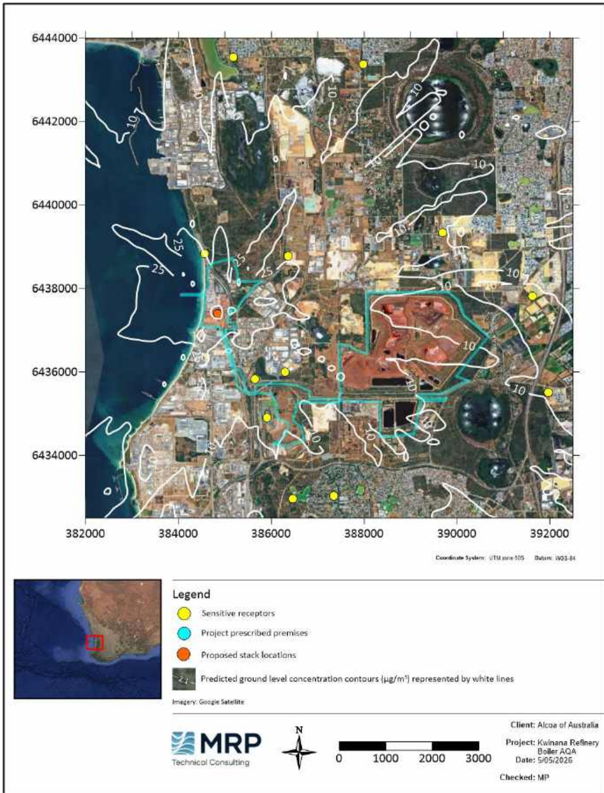
Figure 5-11: Predicted maximum 1-hour average GLCs of NO 2 (Zoomed in) – Scenario 3a – Boiler combination 1 – Isolation
