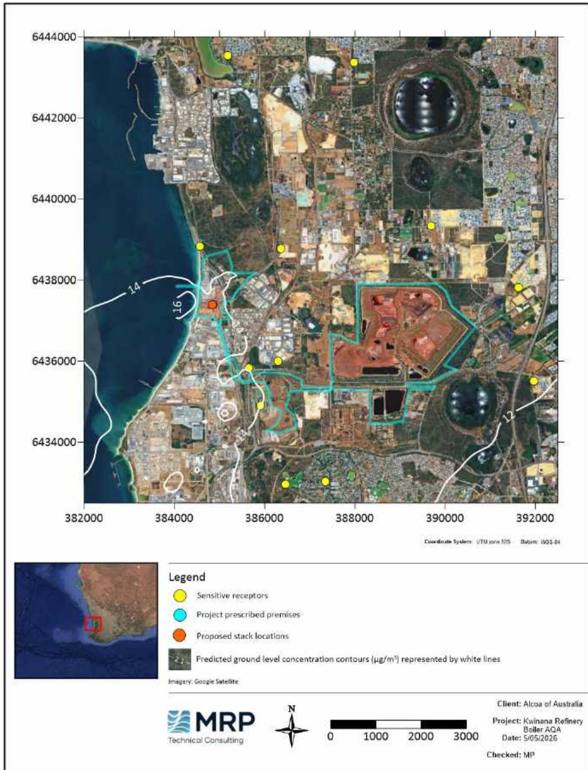
Figure 5-5 Predicted annual average GLCs of NO 2 (Zoomed in) – Scenario 1: Current operations - Cumulative
